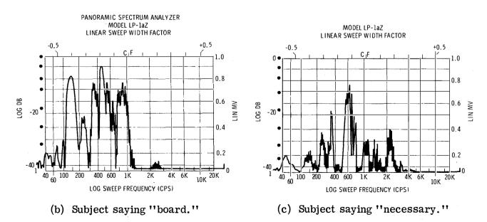
Figure 8. - A spectrum display of Apollo microphone output.
