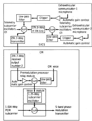
Figure 5. - Command module relay of EVCS signal flow.
