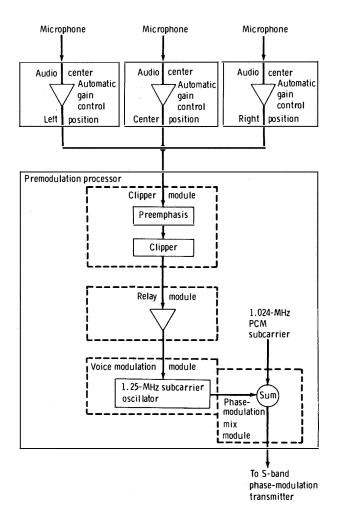
Figure 3. - Command module normalvoice signal flow.
