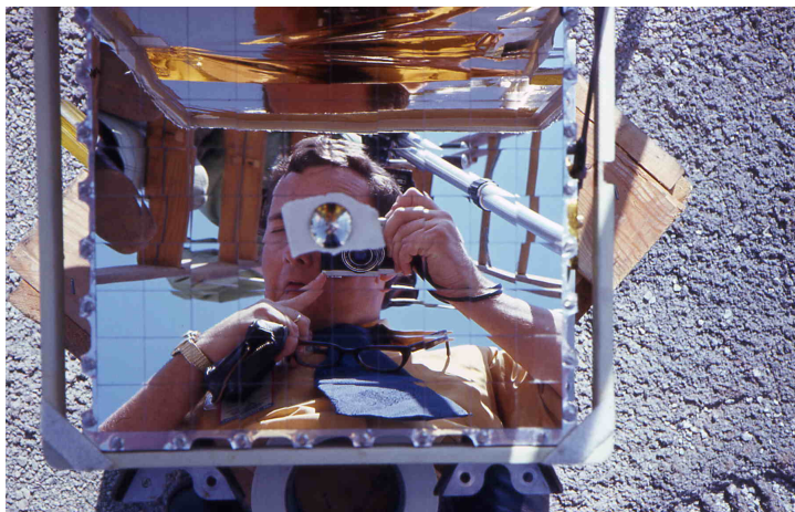
Form Factor meter Photographed To Validate Model Radiator “View Factors” To LM
