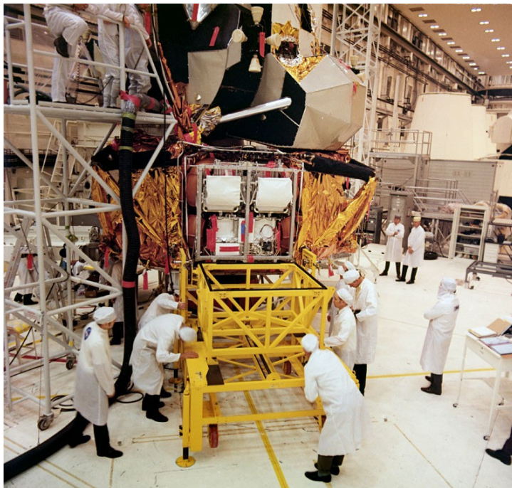
Folded LRV Stowed In Lunar Module With Floor Panels Removed For Battery Installation
