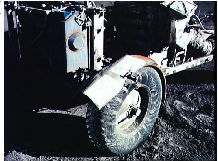
Astronauts Provided Fender Extension Fix
