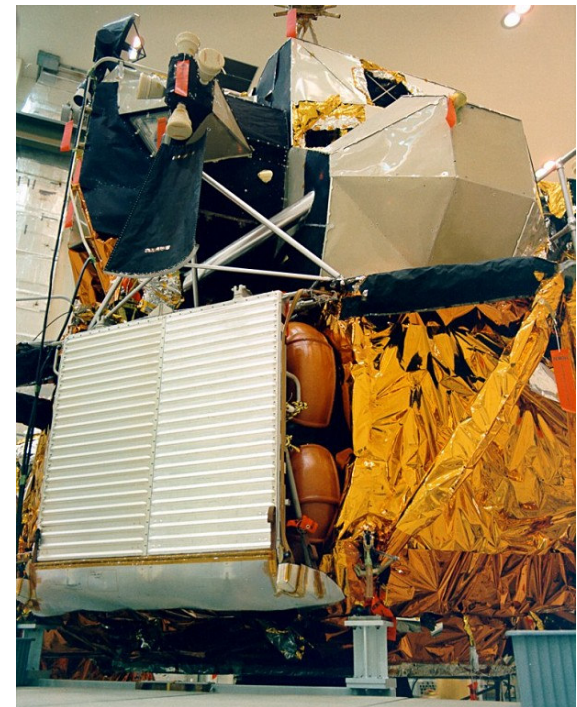
Folded LRV Stowed In Lunar Module With Floor Panels In Place After Battery Installation
