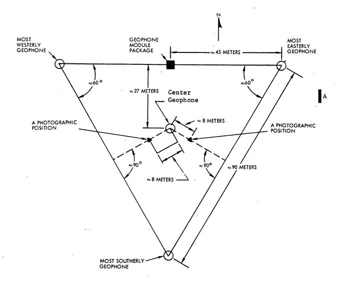
Figure 1. LSPE Geophone Deployment and Photographic Locations
