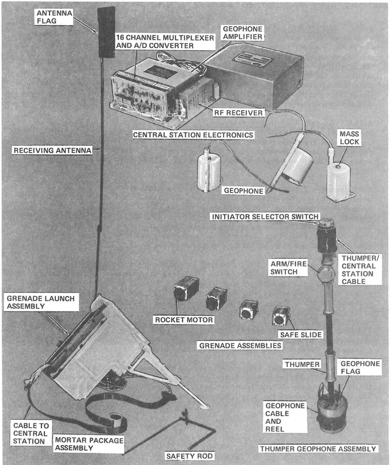
Figure 2-48. Active Seismic Experiment (ASE) Subsystem
