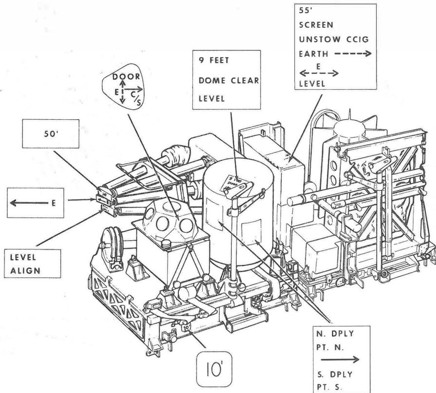
Figure 4-2. Deployment Decals (Typical)
