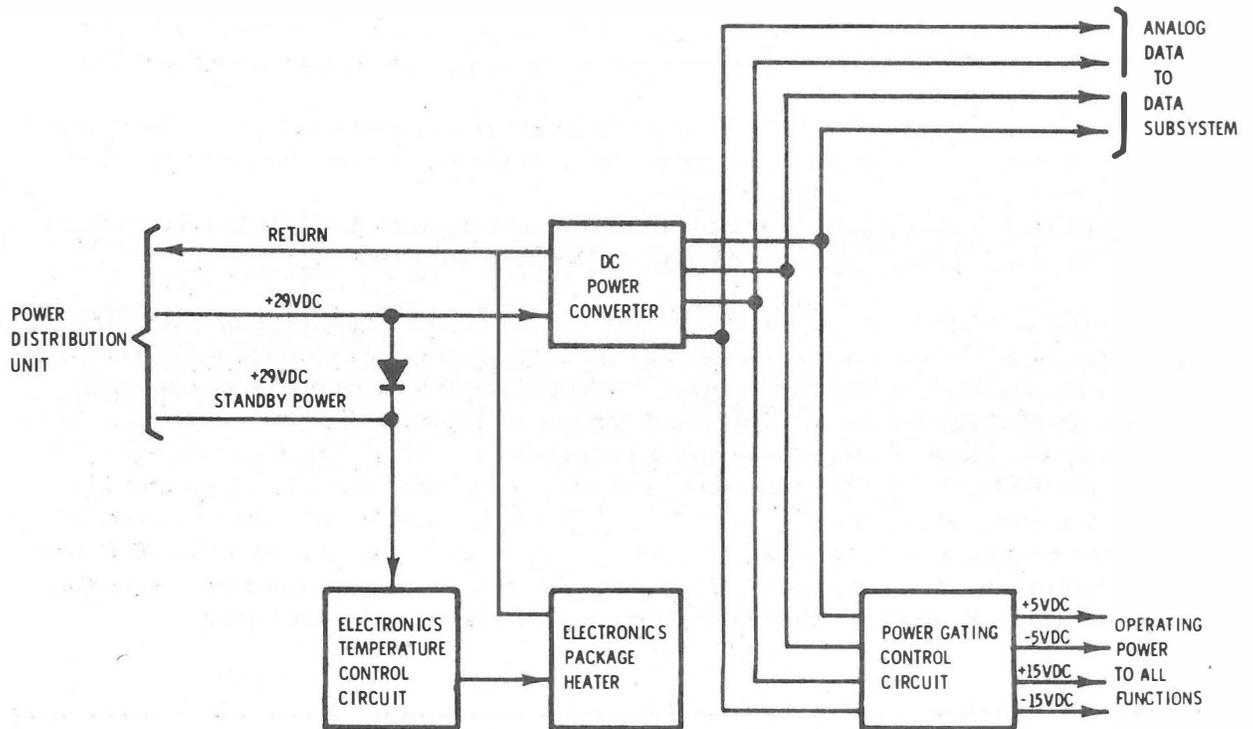
Figure 2-71. HFE Power and Electronics Thermal Control Function, Block Diagram
