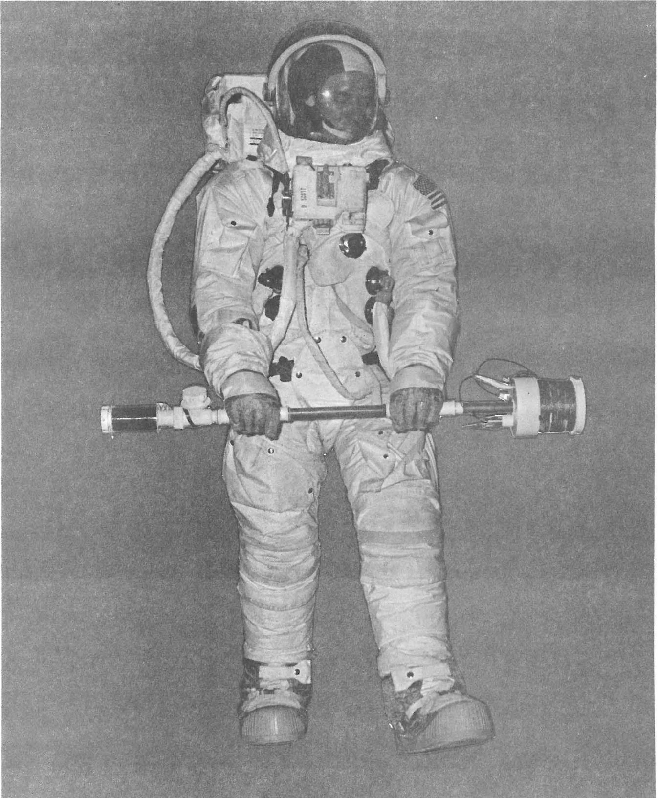
Figure 4-11. Geophone Deployment
