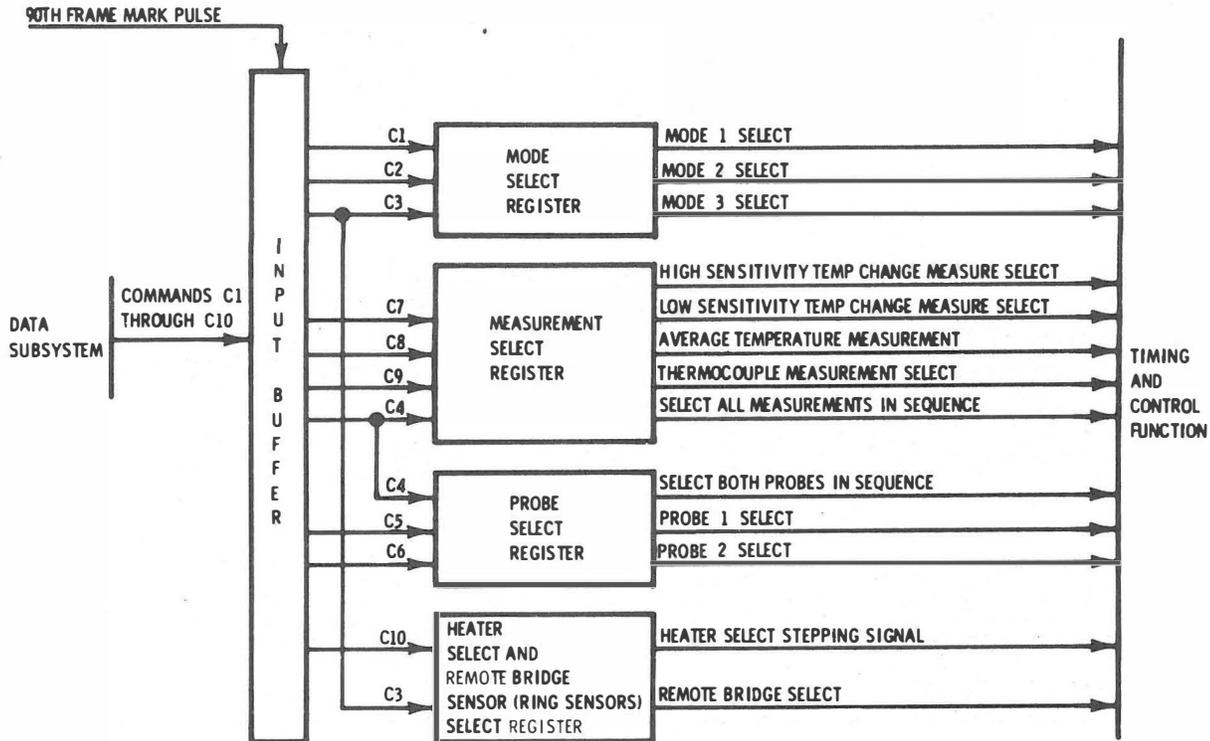
Figure 2-66. HFE Command Processing Function, Block Diagram
