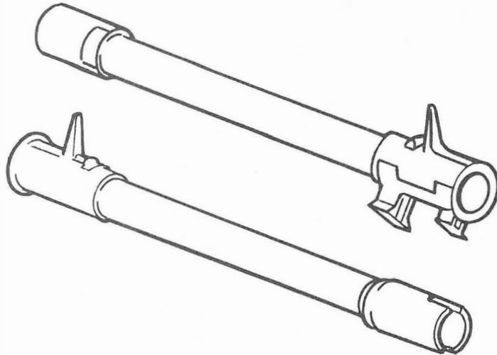
Figure 2-6. Antenna Mast Sections
