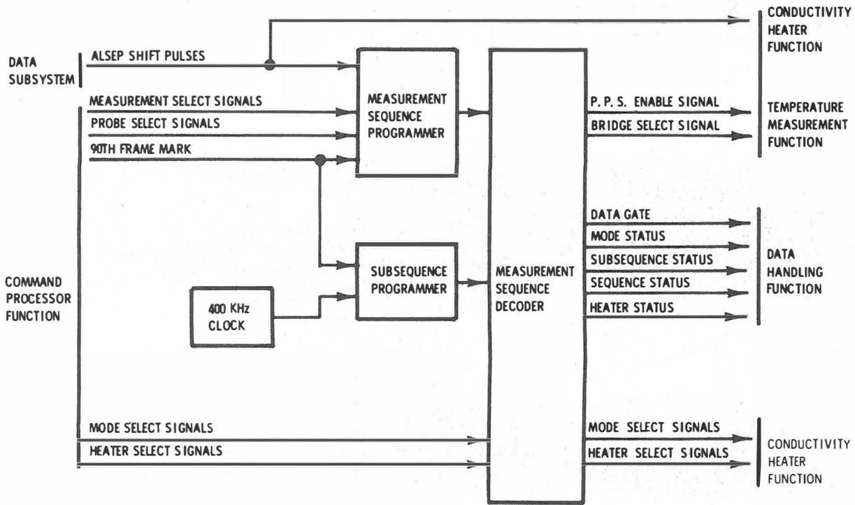
Figure 2-67. HFE Timing and Control Function, Block Diagram
