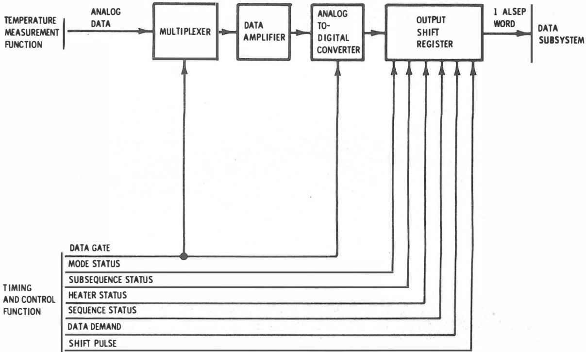
Figure 2-70. HFE Data Handling Function, Block Diagram
