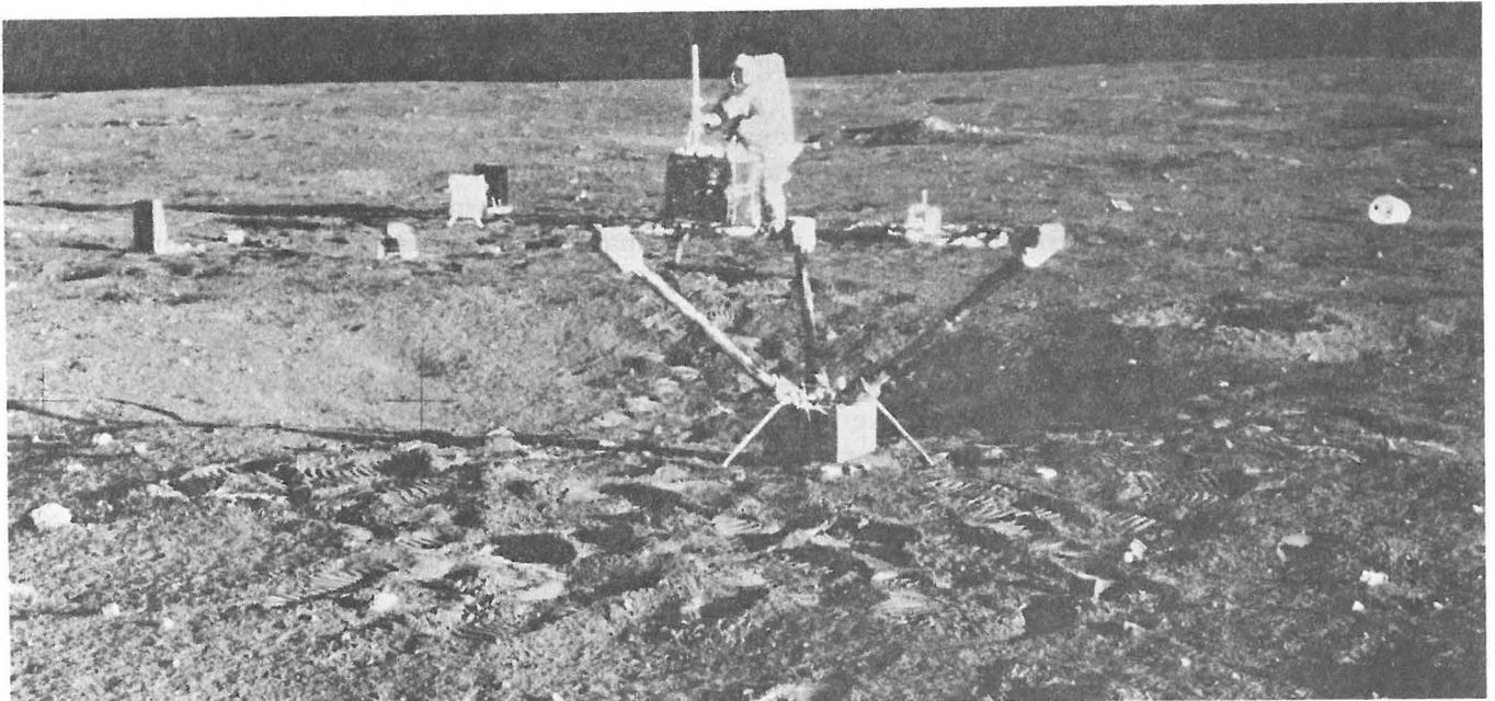
Figure 1-7. Apollo 12 ALSEP Deployed on Lunar Surface
