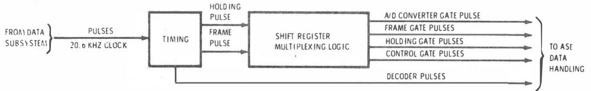
Figure 2-52. ASE Timing and Control Function, Block Diagram
