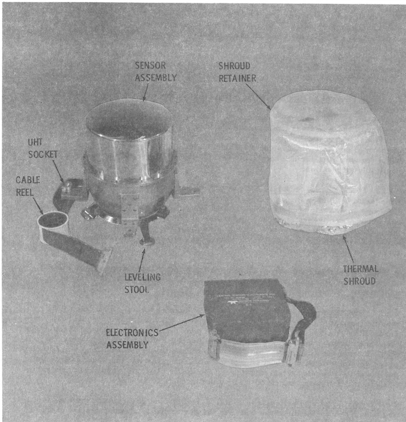
Figure 2-39. Passive Seismic Experiment Subsystem
