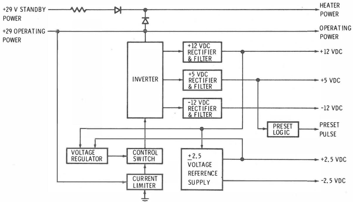
Figure 2-47. PSE Power Converter Function, Block Diagram
