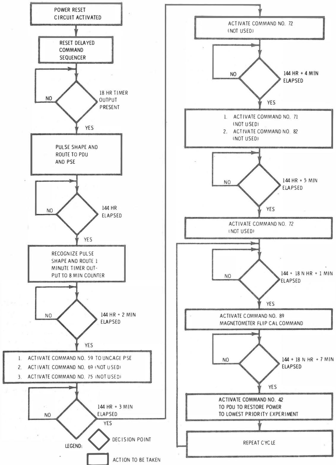
Figure 2-24. Data Subsystem Delayed Command Sequence, Functional Flow Chart
