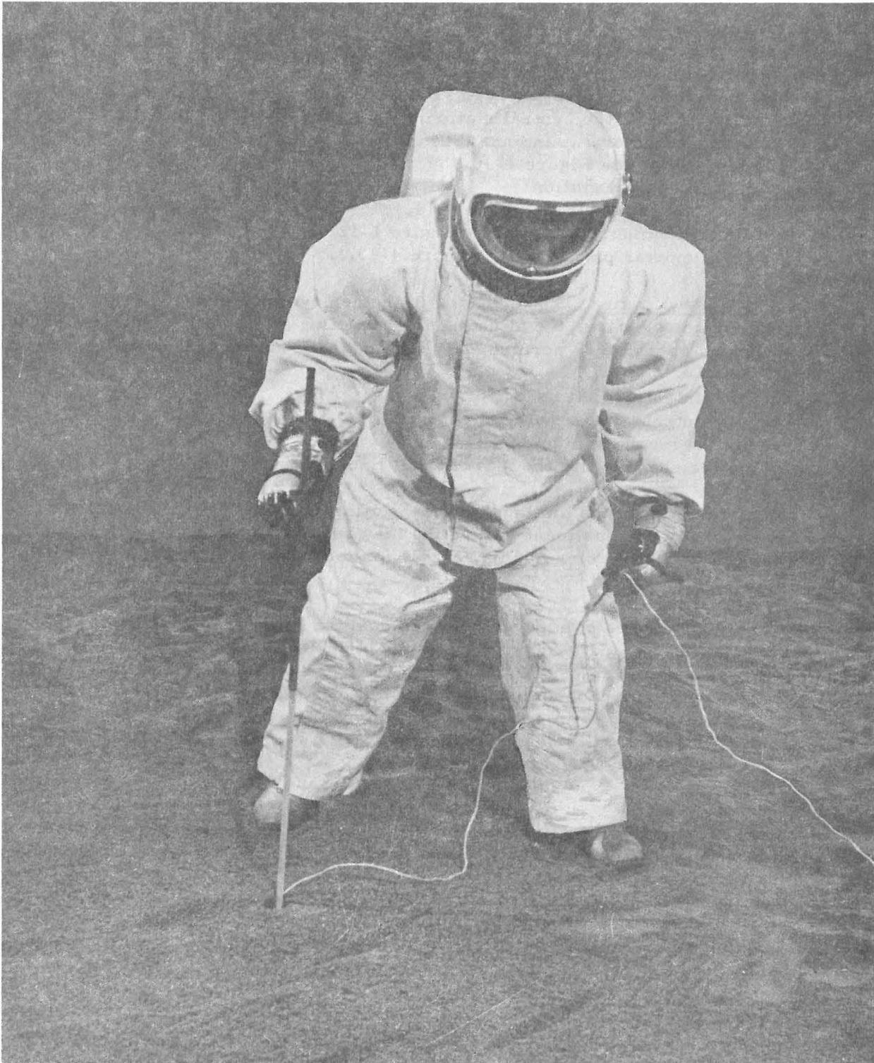
Figure 4-7. HFE Probe Emplacement
