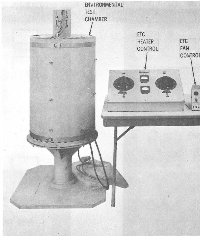
Figure 3-7. Environmental Test Chamber
