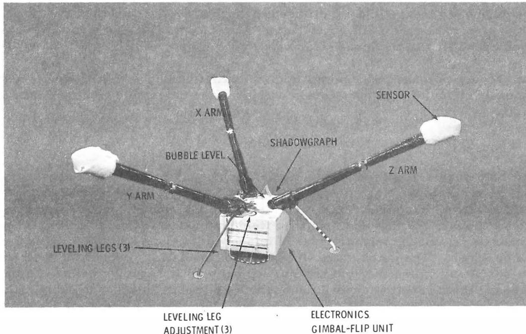
Figure 2-55. Lunar Surface Magnetometer Experiment
