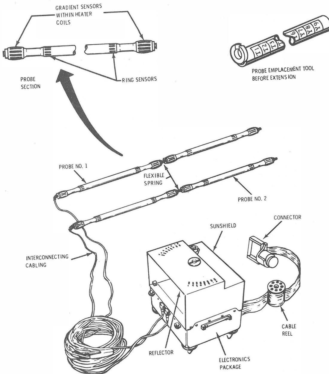
Figure 2-64. Heat Flow Experiment (HFE) Subsystem
