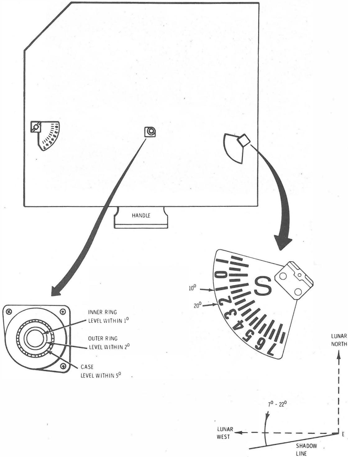
Figure 4-3. Alignment and Leveling Devices (Sheet 1 of 6)
