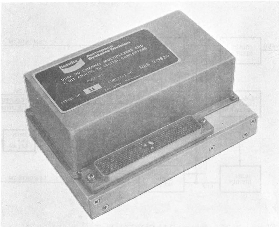
Figure 2-28. Data Subsystem Analog Data Multiplexer/Converter
