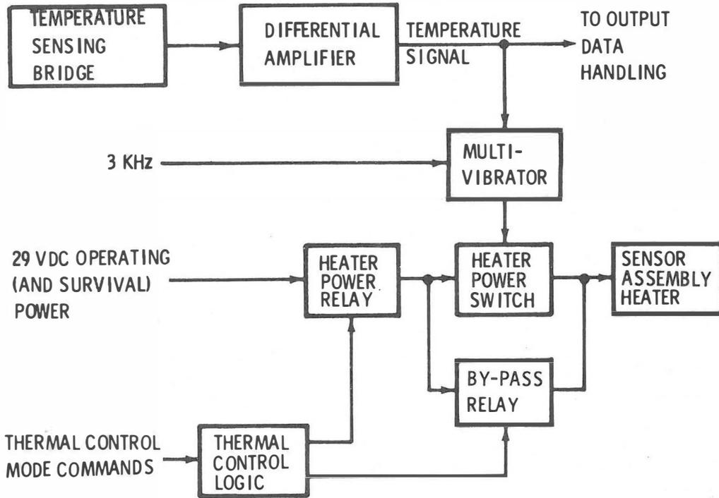
Figure 2-46. PSE Thermal Control Function, Block Diagram
