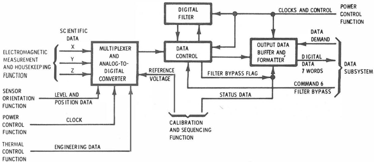
Figure 2-61. LSM Data Handling Function, Block Diagram
