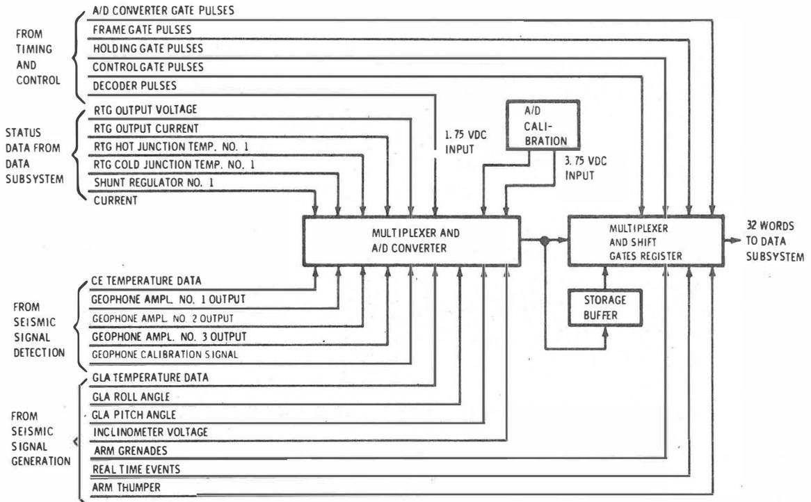
Figure 2-53. ASE Data Handling Function, Block Diagram
