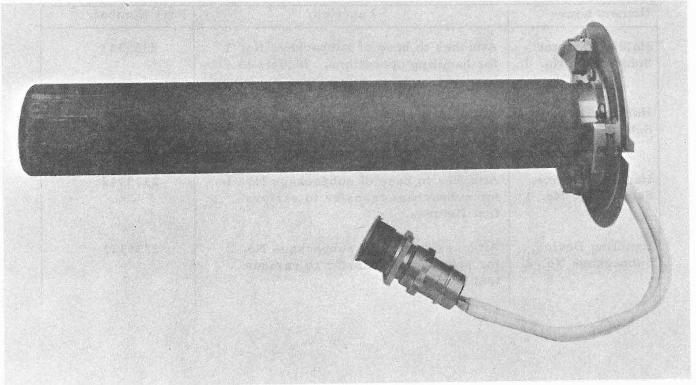
Figure 3-14. Electric Fuel Capsule Simulator
