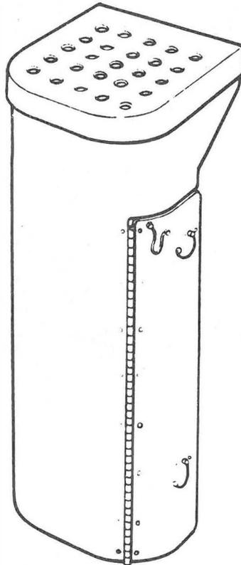
Figure 3-19. Cask Assembly Protective Cover
