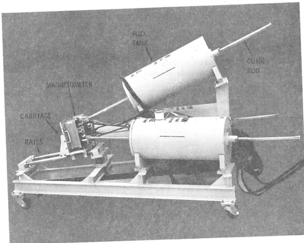
Figure 3-4. Magnetometer Flux Tanks (Configuration B)
