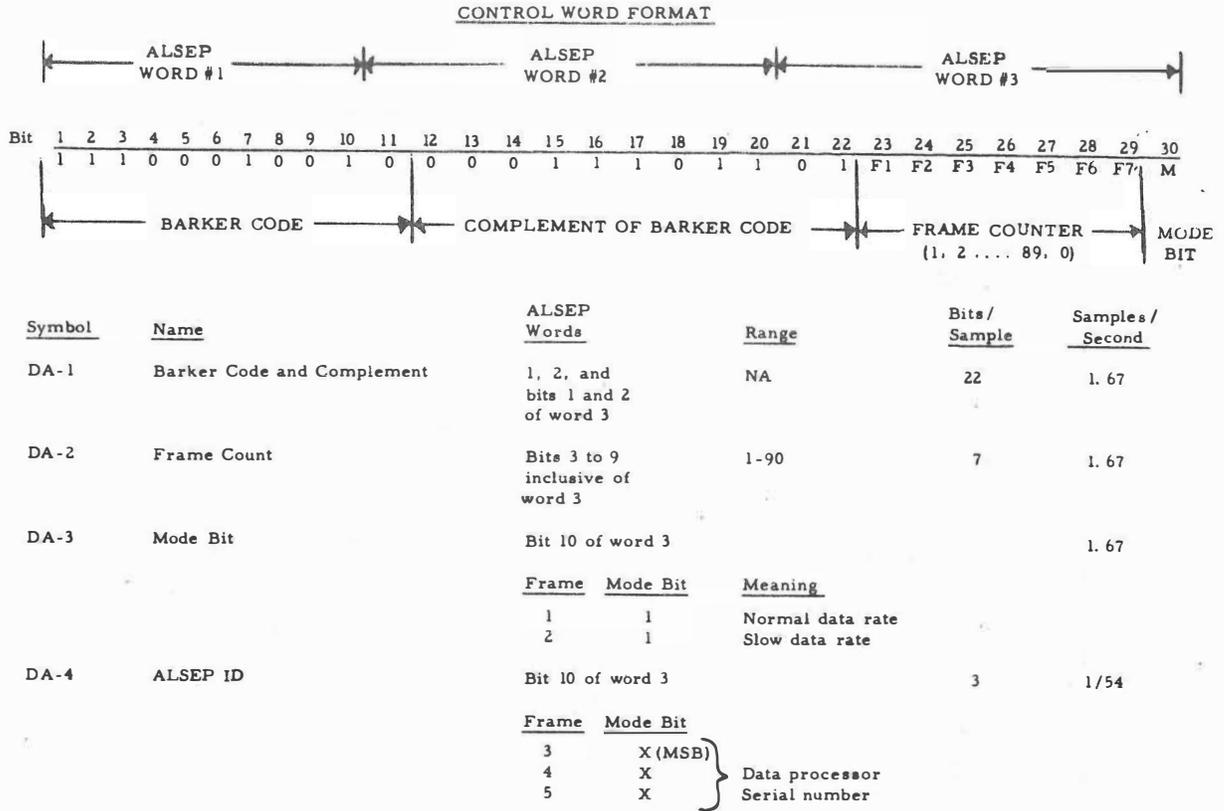
Figure 2-31. ALSEP Telemetry Control Word Bit Assignments
