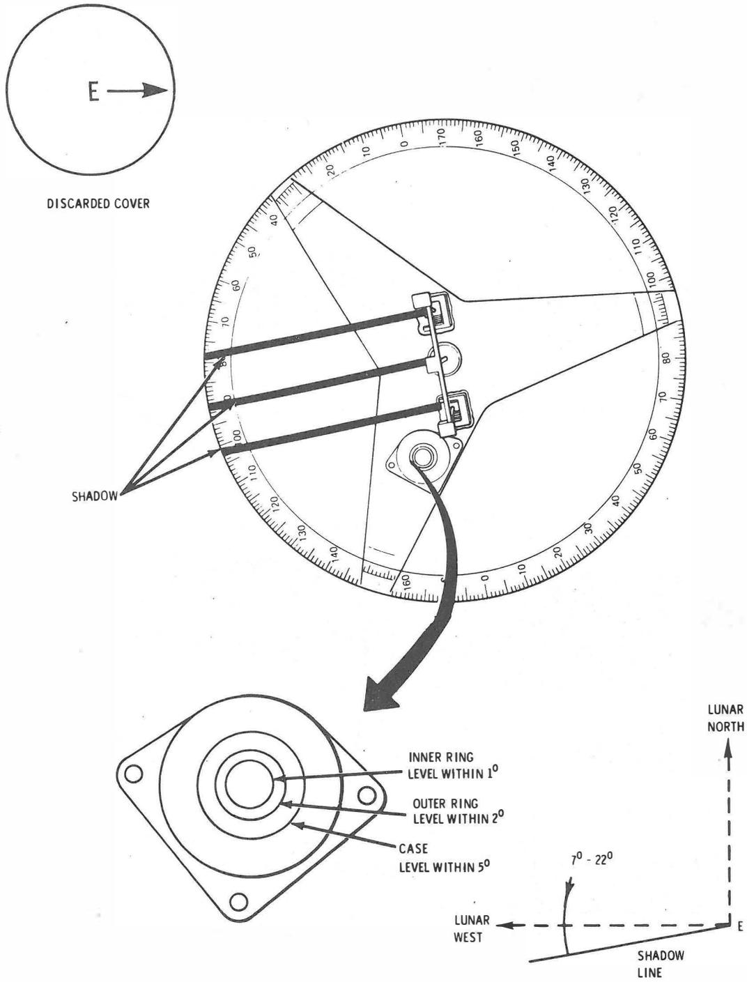
Figure 4-3. Alignment and Leveling Devices (Sheet 3 of 6)
