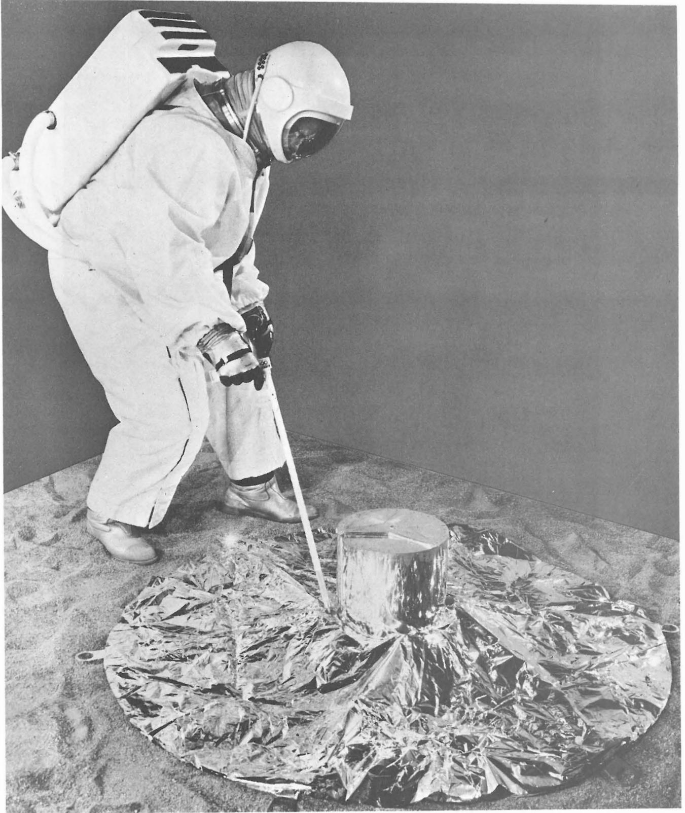
Figure 4-5. PSE Shroud Deployment and Experiment Leveling
