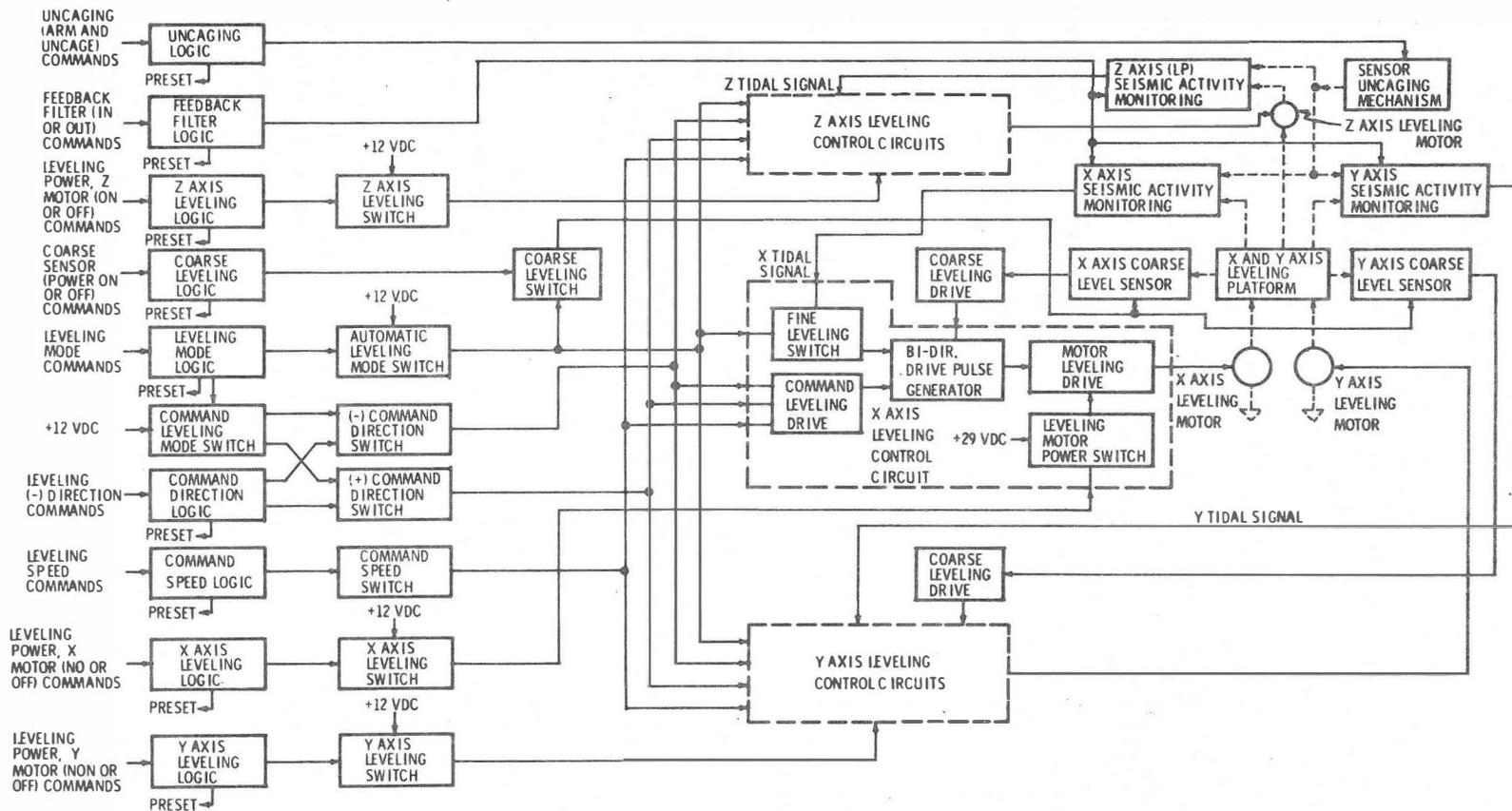
Figure 2-45. PSE Uncaging and Leveling Function, Block Diagram
