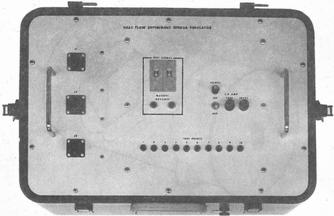
Figure 3-13. Heat Flow Sensor Simulator
