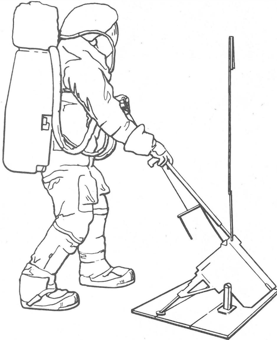
Figure 4-13. Mortar Package Deployment
