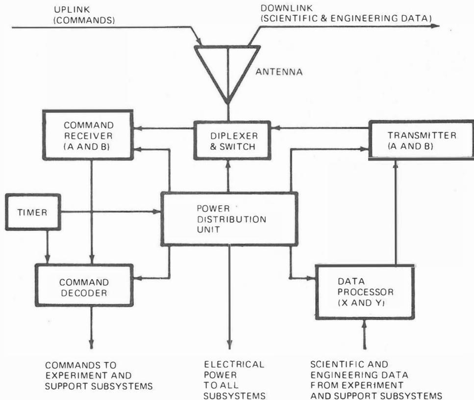
Figure 2-11. Data Subsystem, Simplified Block Diagram
