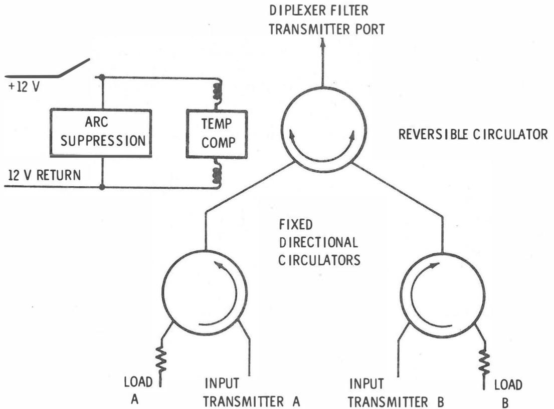
Figure 2-17. Data Subsystem Diplexer Switch Diagram
