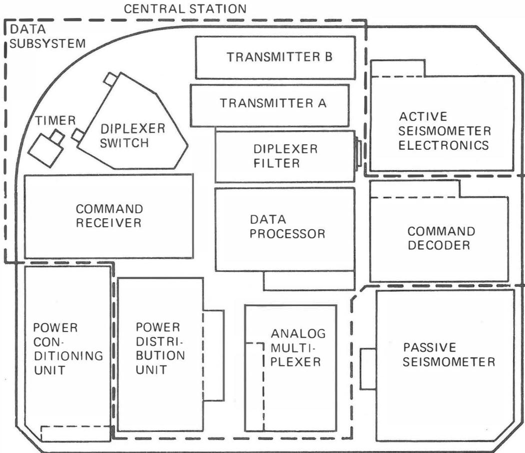
Figure 2-12. Data Subsystem Component Location
