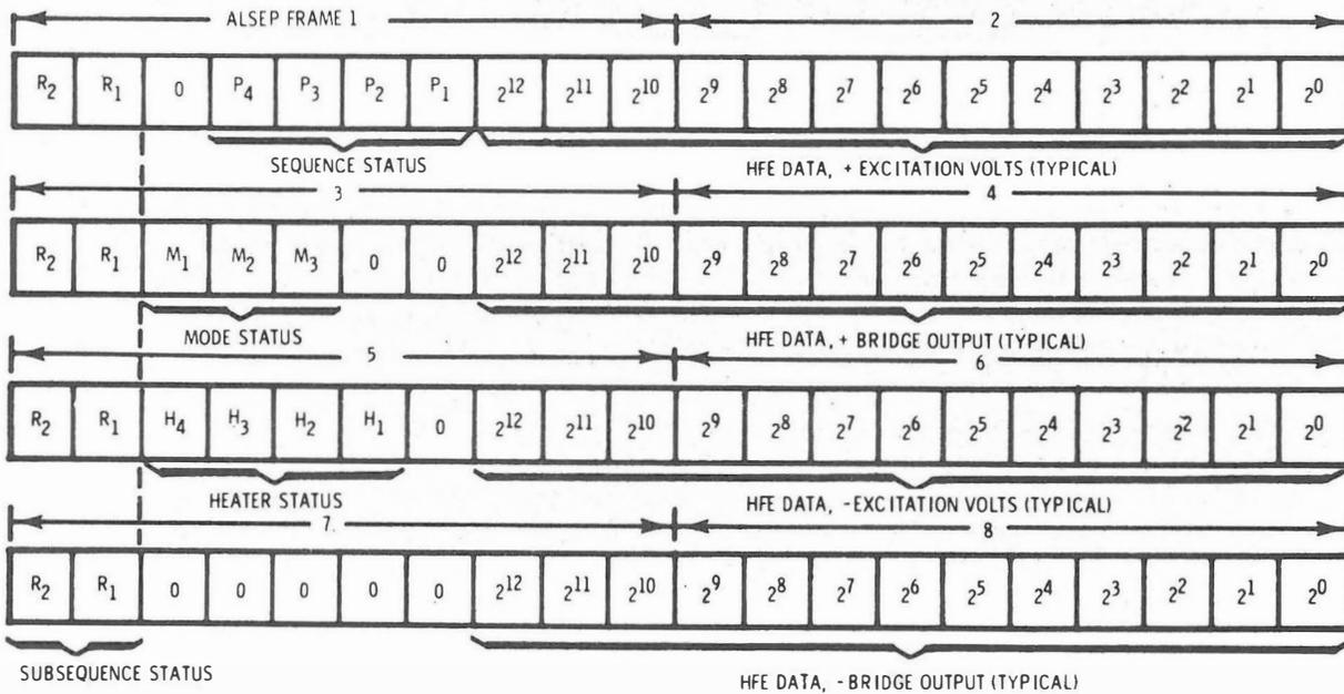
Figure 2-72. HFE Measurement Digital Data Format
