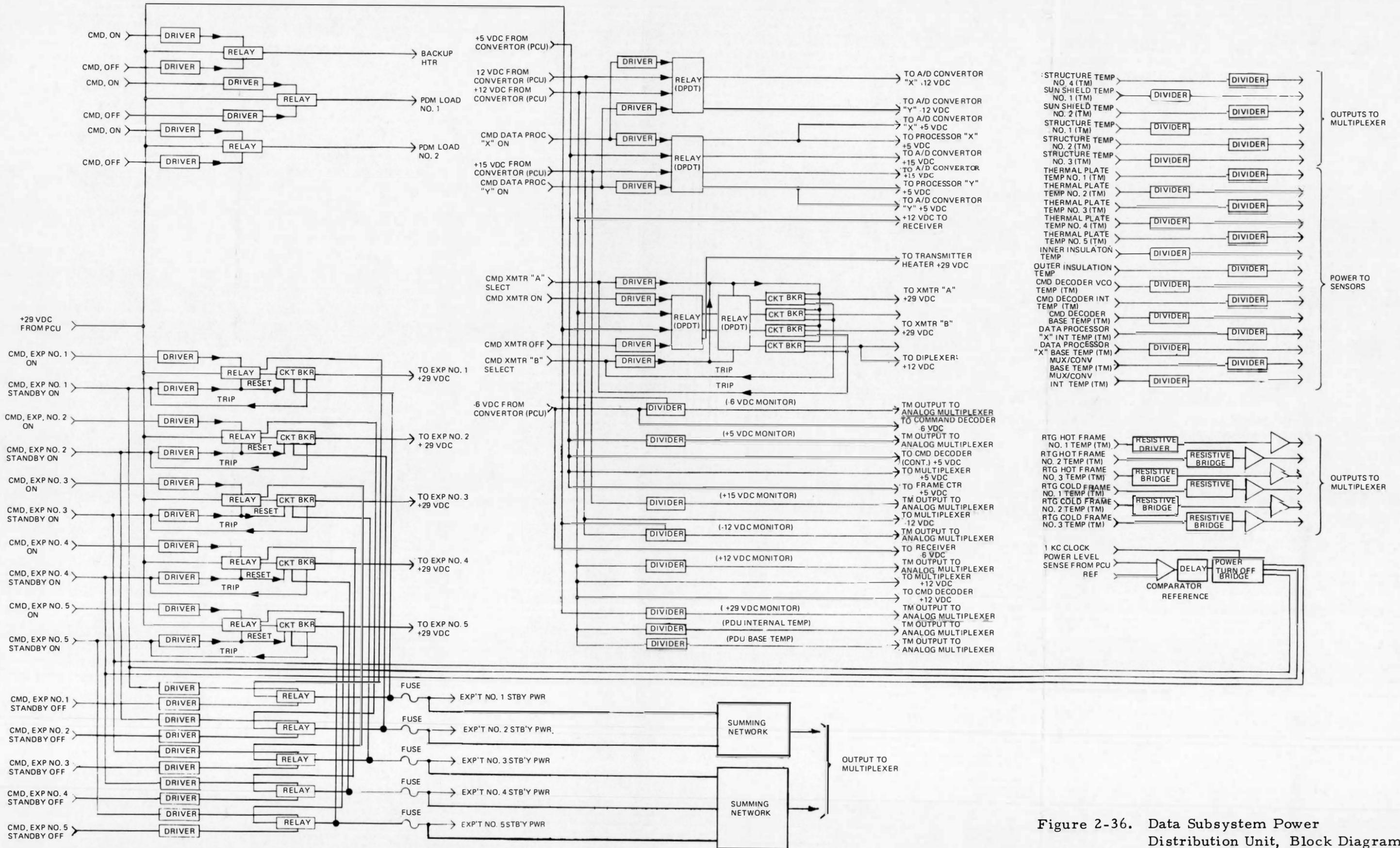
Figure 2-36. Data Subsystem Power Distribution Unit, Block Diagram
