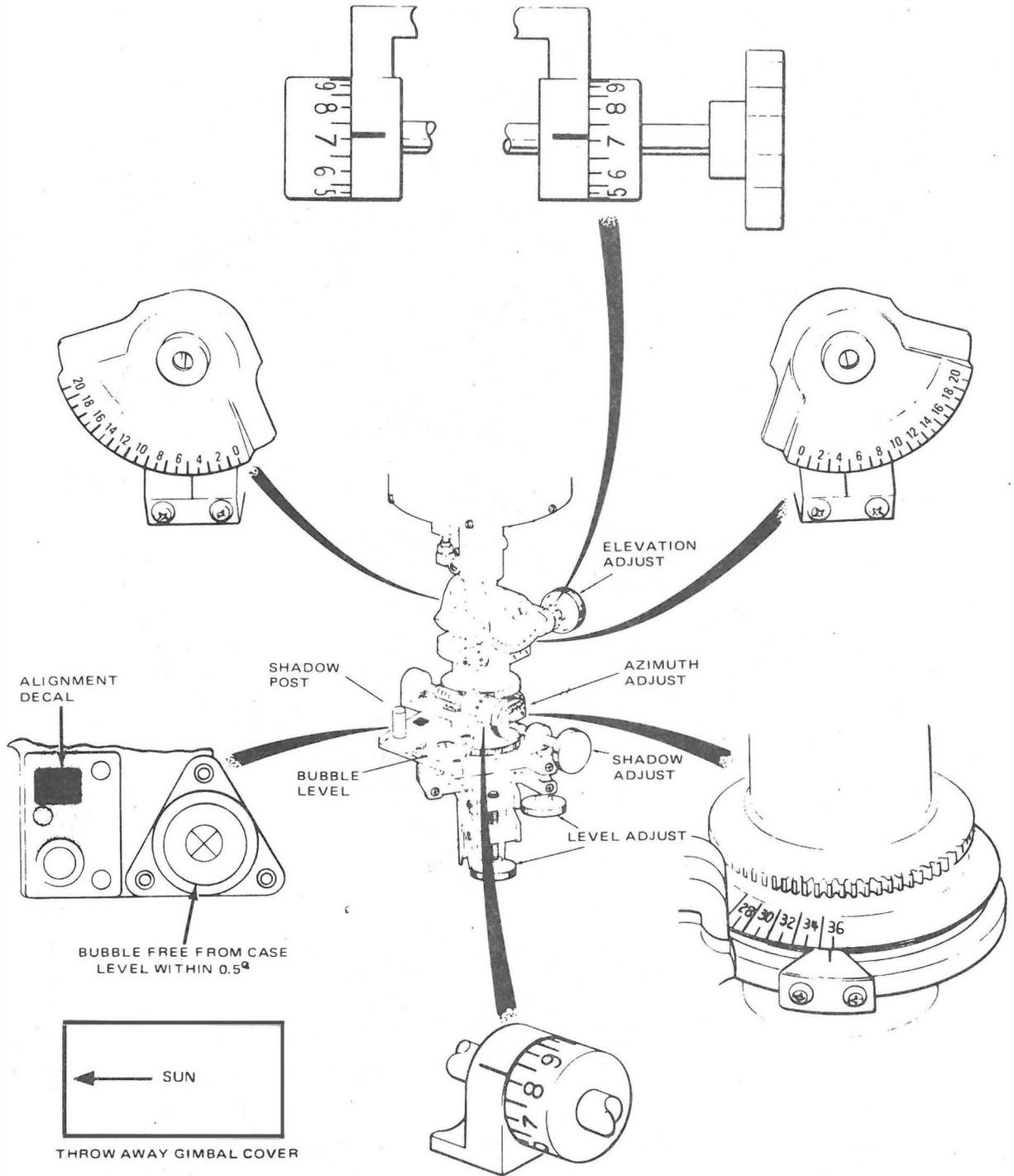
Figure 4-3. Alignment and Leveling Devices (Sheet 2 of 6)
