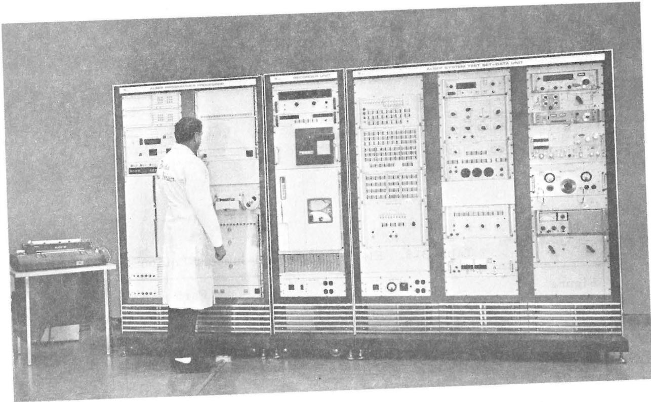
Figure 3-3. ALSEP System Test Set
