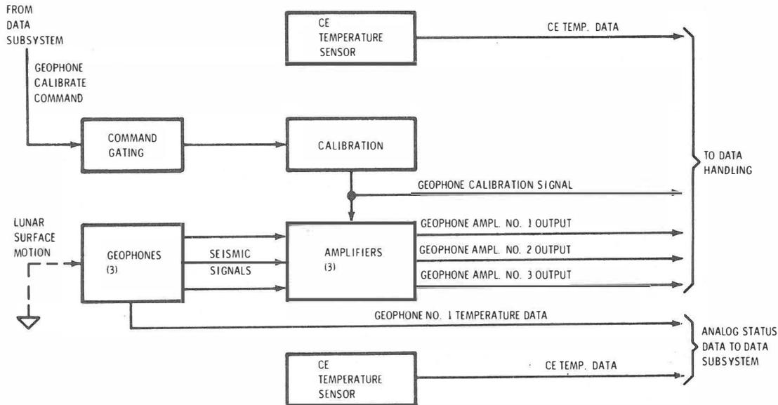
Figure 2-51. ASE Seismic Signal Detection Function, Block Diagram
