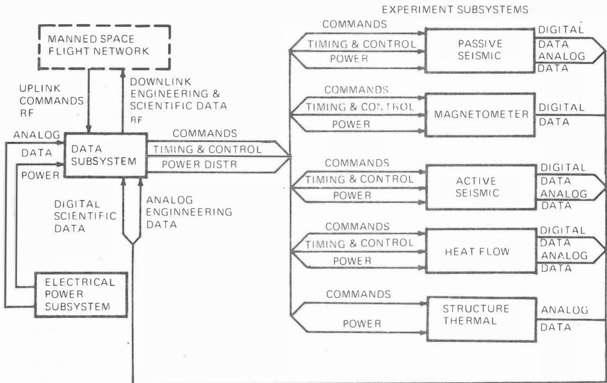
Figure 1-4. Apollo 16 ALSEP System, Simplified Block Diagram
