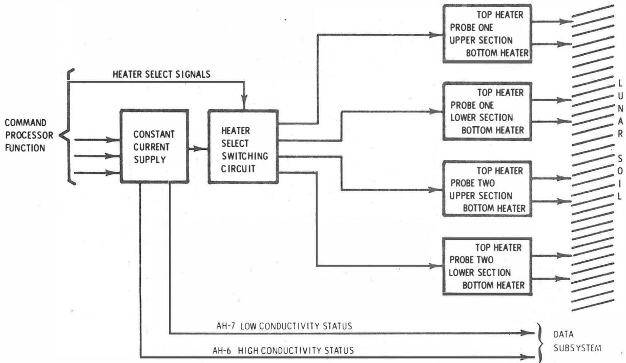
Figure 2-69. HFE Conductivity Heater Function, Block Diagram
