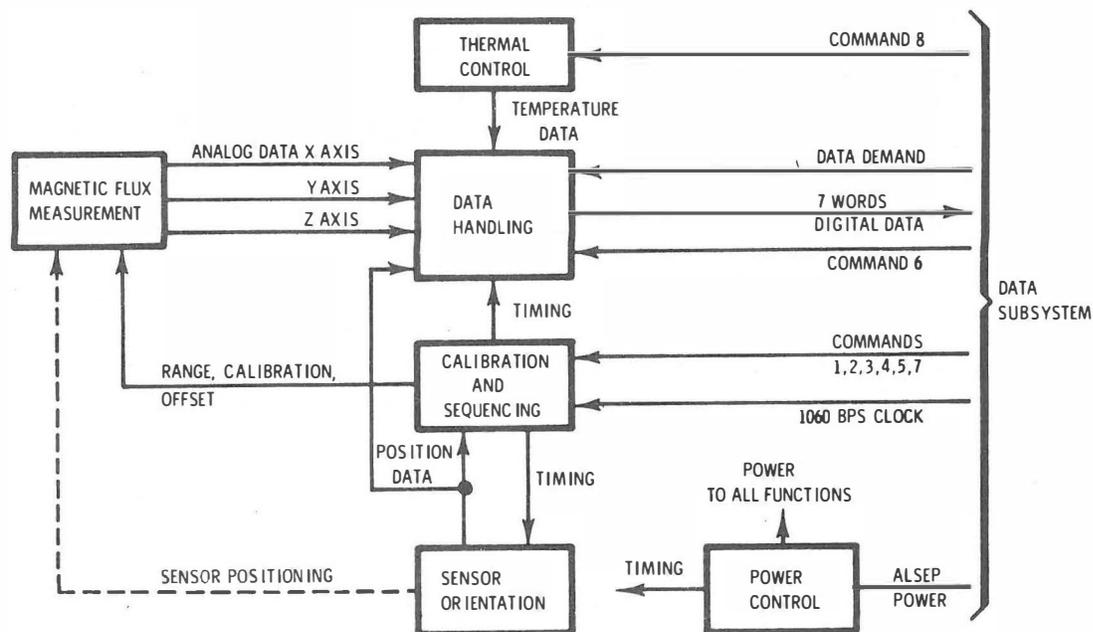
Figure 2-56. LSM Experiment, Functional Block Diagram
