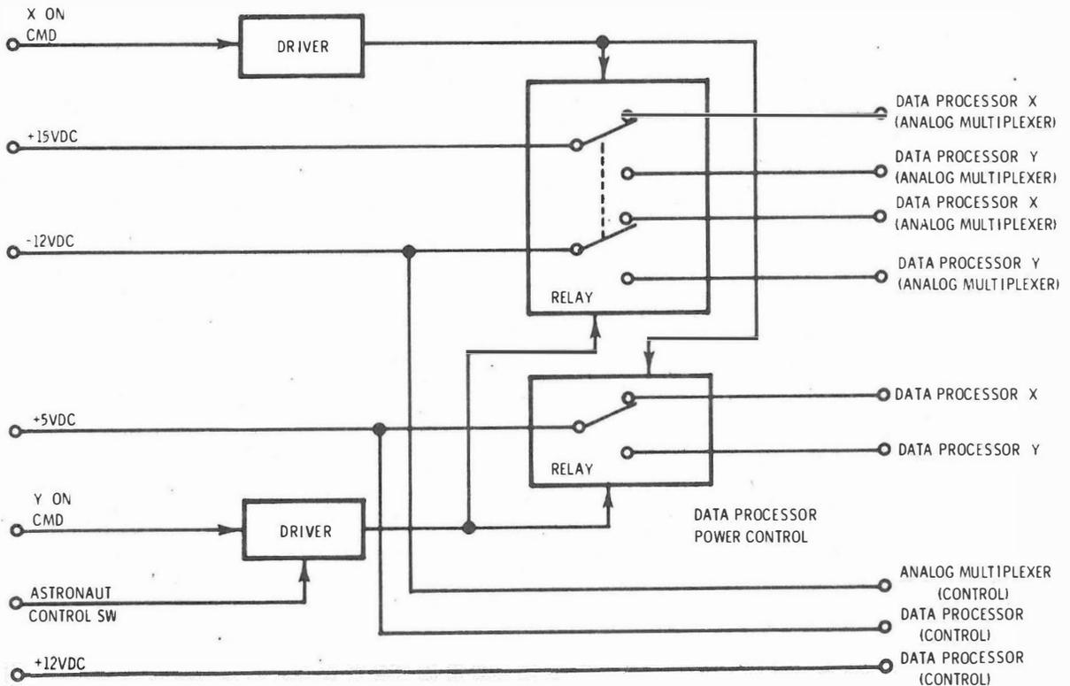
Figure 2-38. Data Processor Power Control
