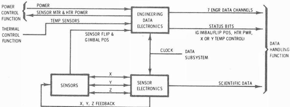
Figure 2-57. LSM Electromagnetic Measurement and Housekeeping Function, Block Diagram
