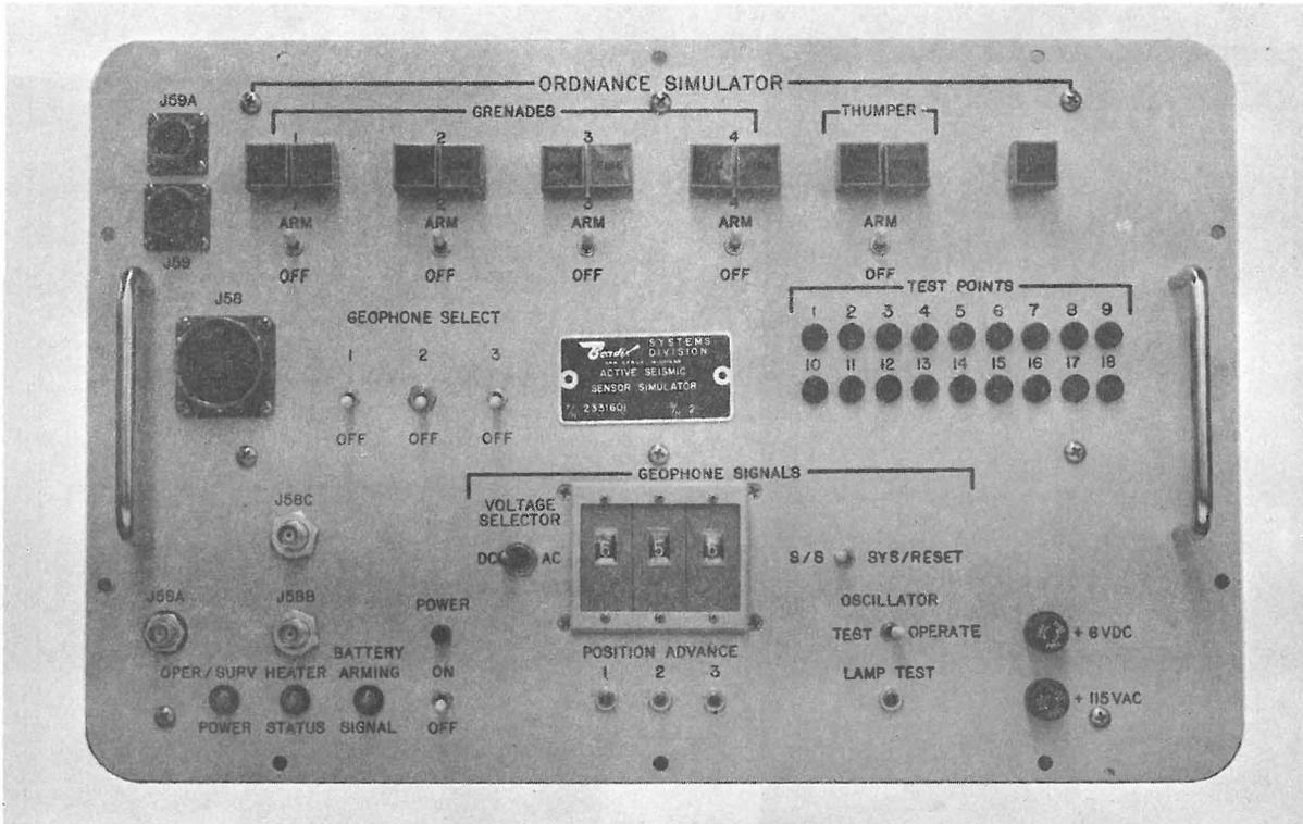
Figure 3-11. Active Seismic Sensor Simulator
