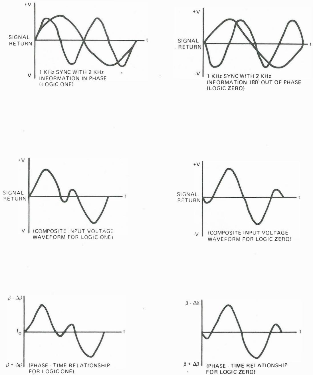
Figure 2-20. Data Subsystem Command Receiver Output Signal Characteristics
