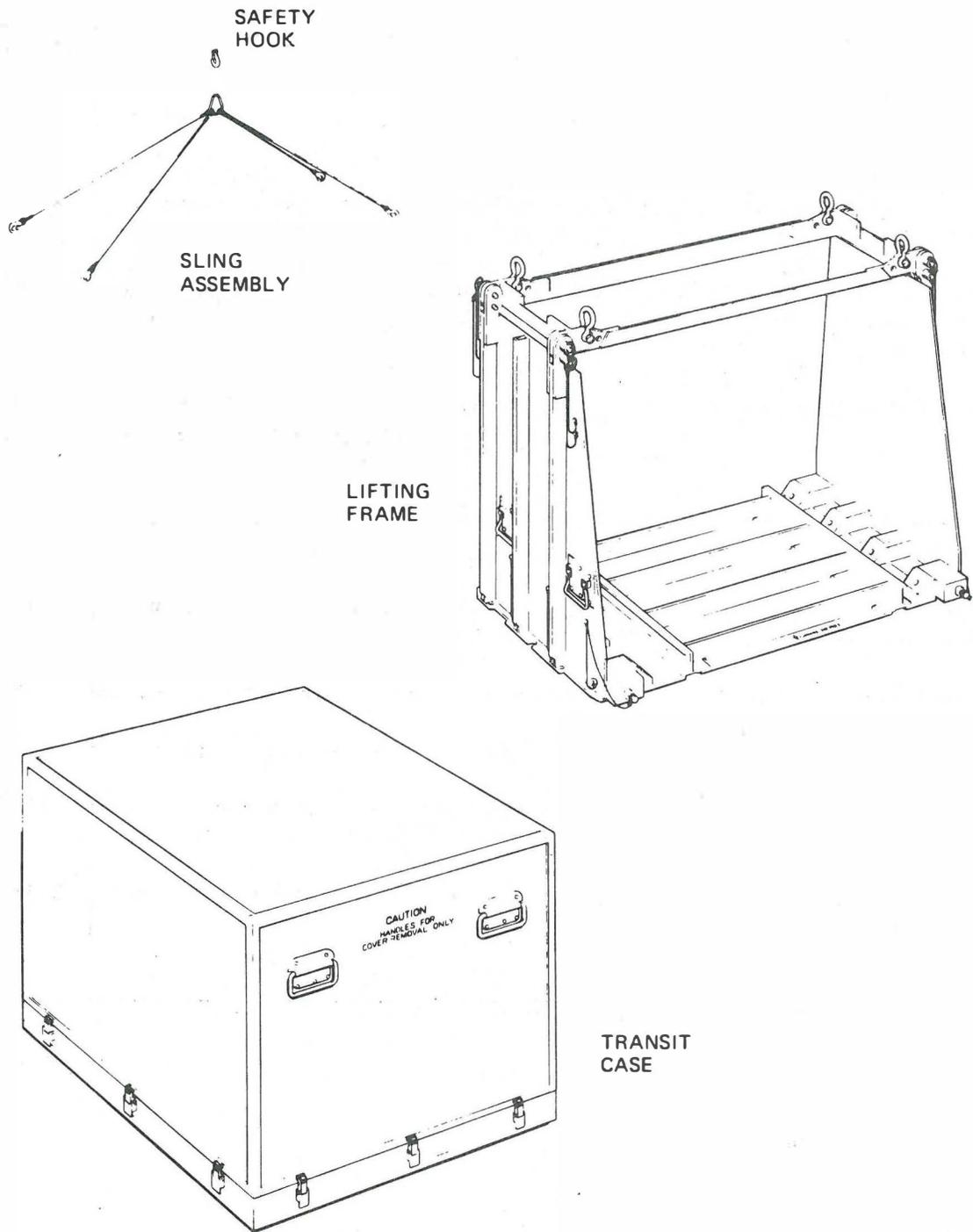
Figure 3-20. SLA Installation GSE
