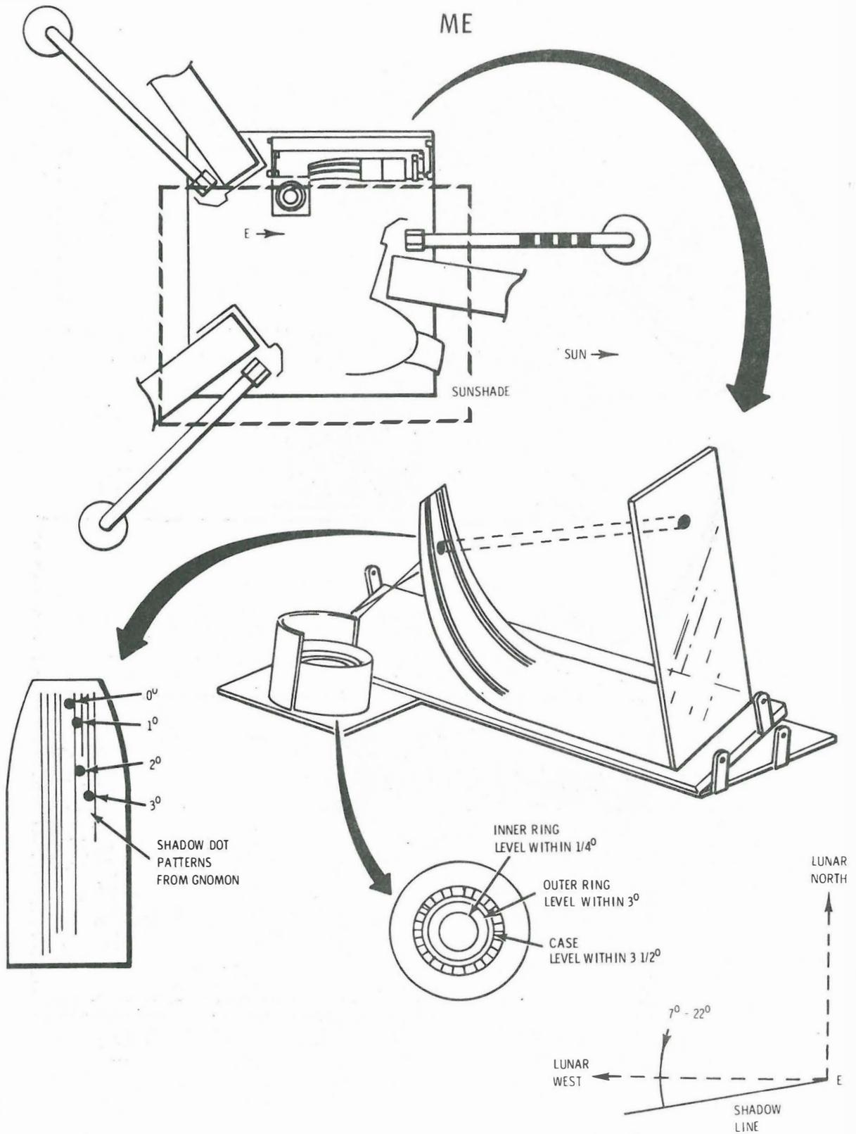
Figure 4-3. Alignment and Leveling Devices (Sheet 4 of 6)
