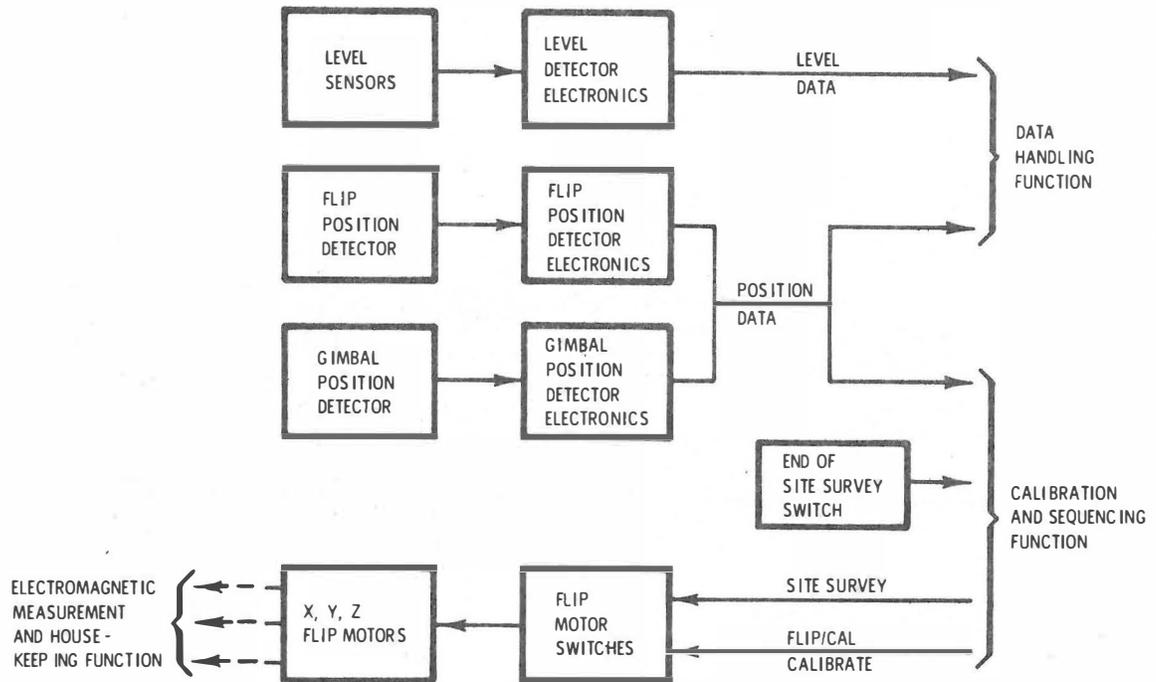
Figure 2-59. LSM Sensor Orientation Function, Block Diagram
