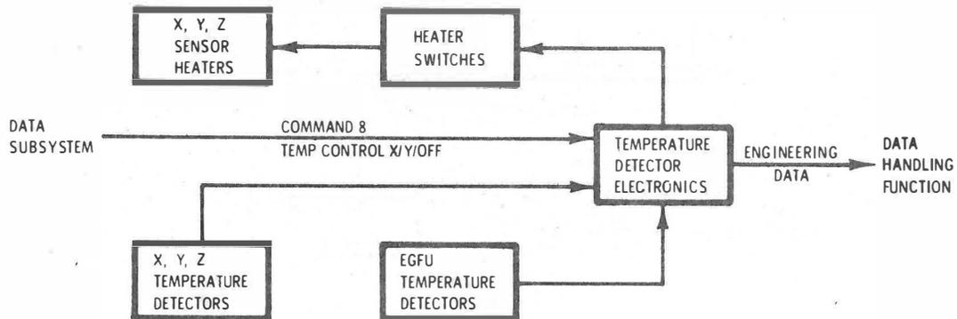
Figure 2-62. LSM Thermal Control Function, Block Diagram
