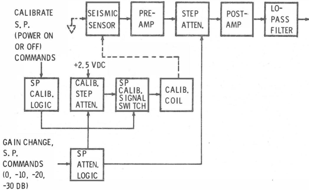
Figure 2-42. PSE Short Period Seismic Activity Monitoring Function, Block Diagram
