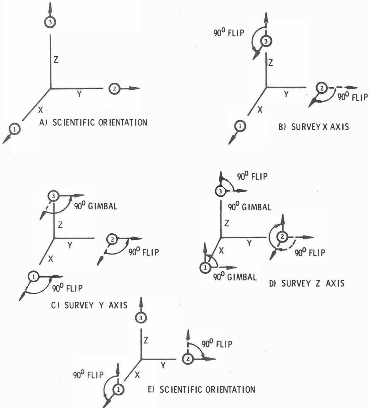
Figure 2-60. LSM Site Survey Sensor Gimbal and Flip Sequence
