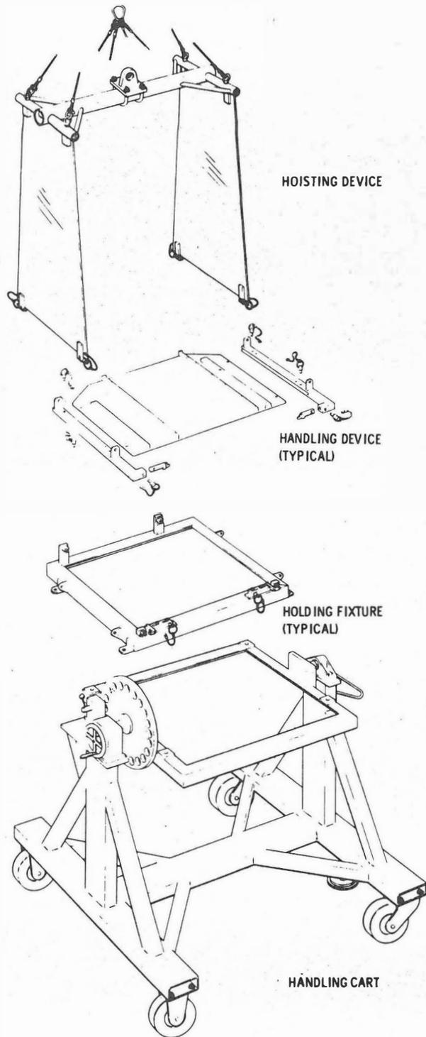
Figure 3-16. Subpackage Handling GSE
