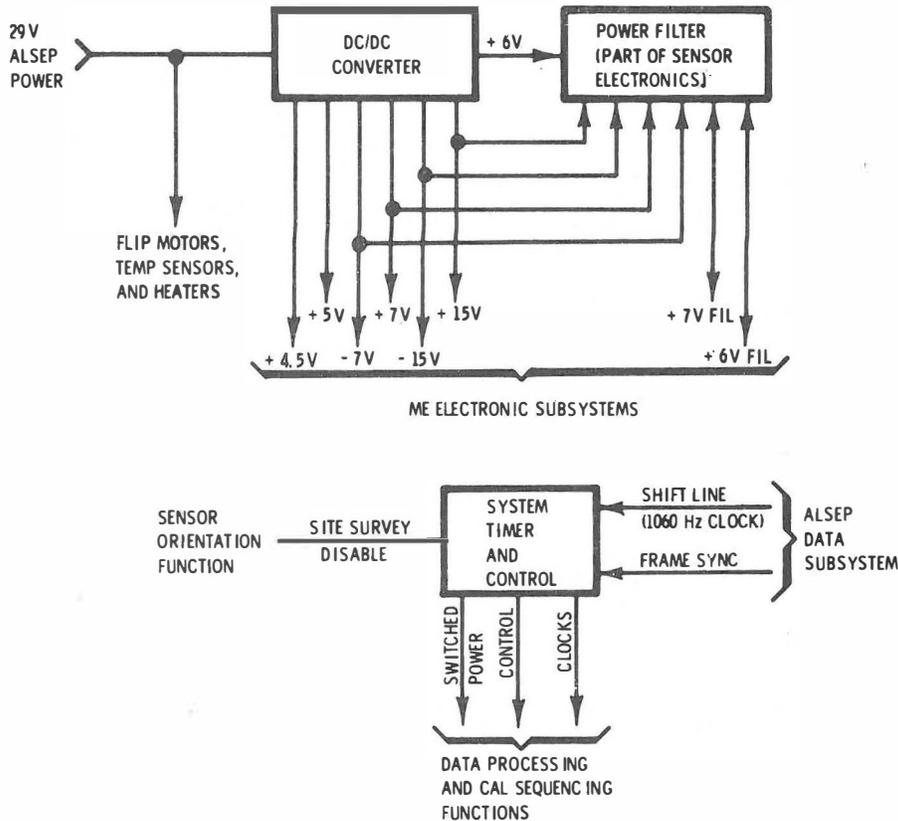
Figure 2-63. LSM Power Control and Timing Function, Block Diagram
