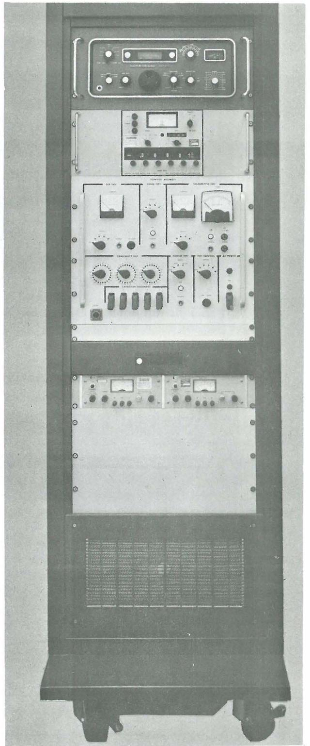
Figure 3-10. Grenade Launch Assembly Test Set
