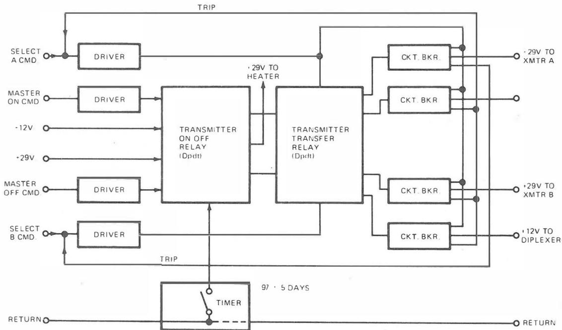
Figure 2-37. Data Subsystem Transmitter Power Control
