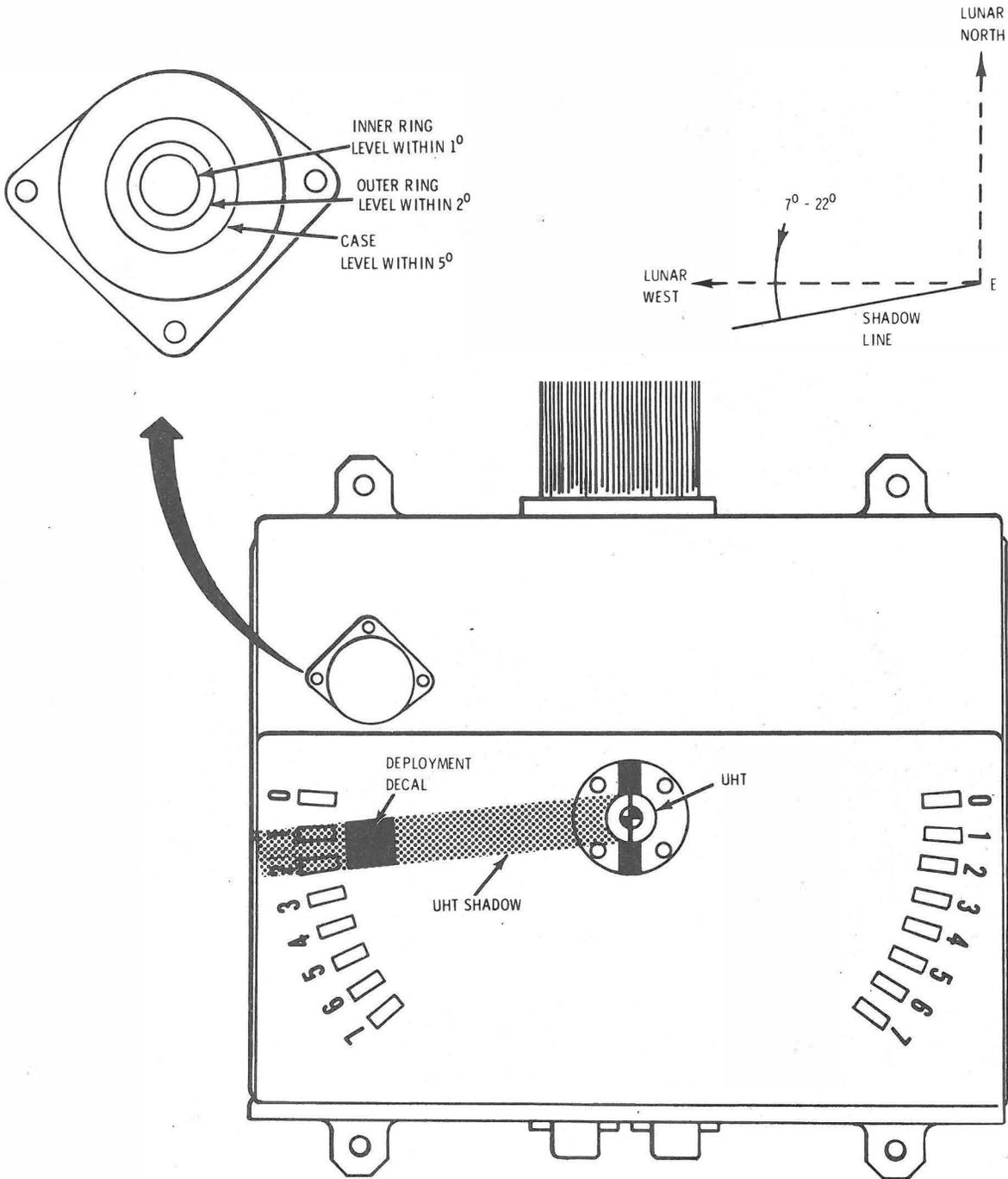
Figure 4-3. Alignment and Leveling Devices (Sheet 5 of 6)
