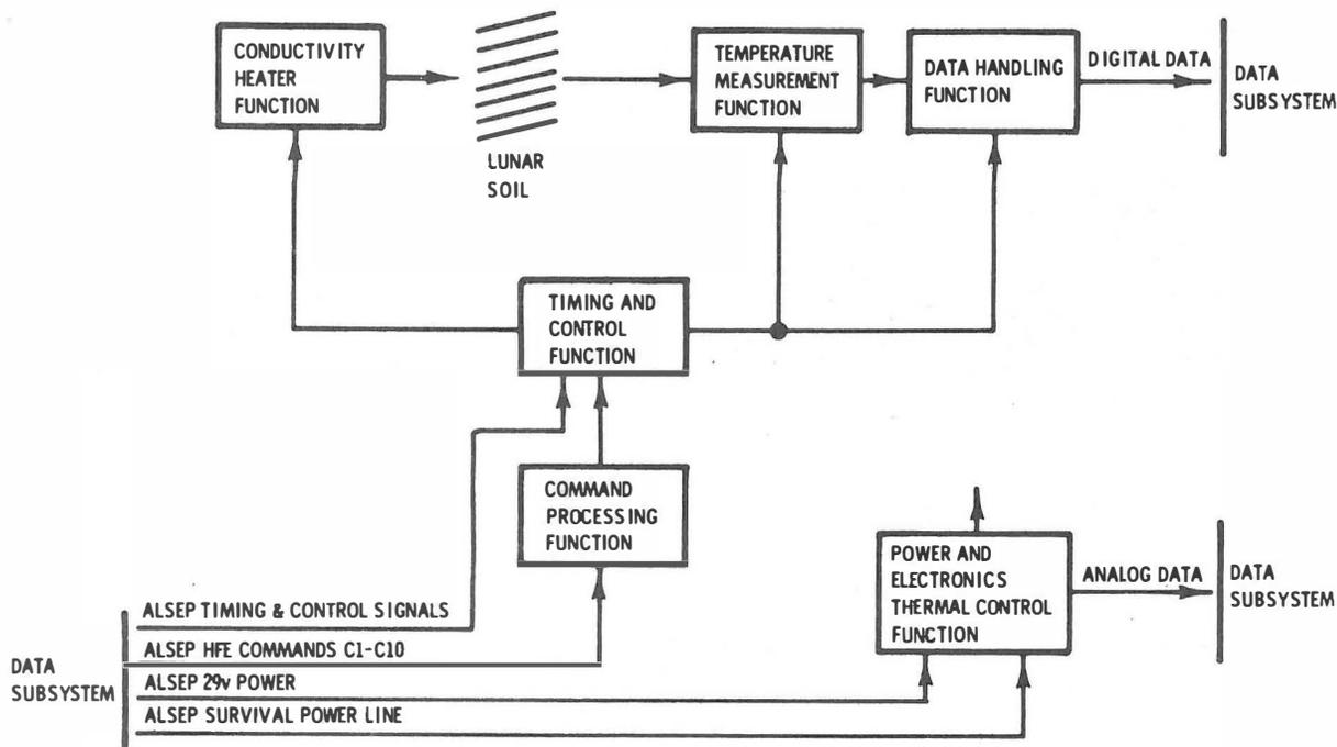
Figure 2-65. Heat Flow Experiment, Functional Block Diagram
