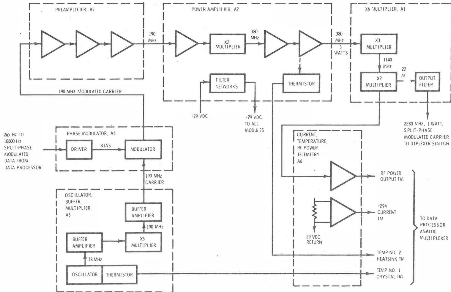
Figure 2-34. Data Subsystem Transmitter, Block Diagram
