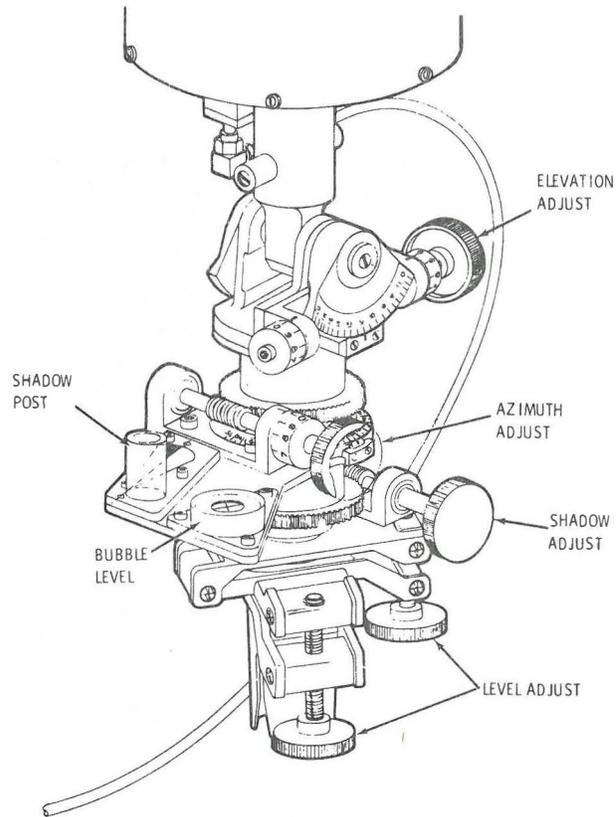
Figure 4-14. Antenna Aiming Mechanism
