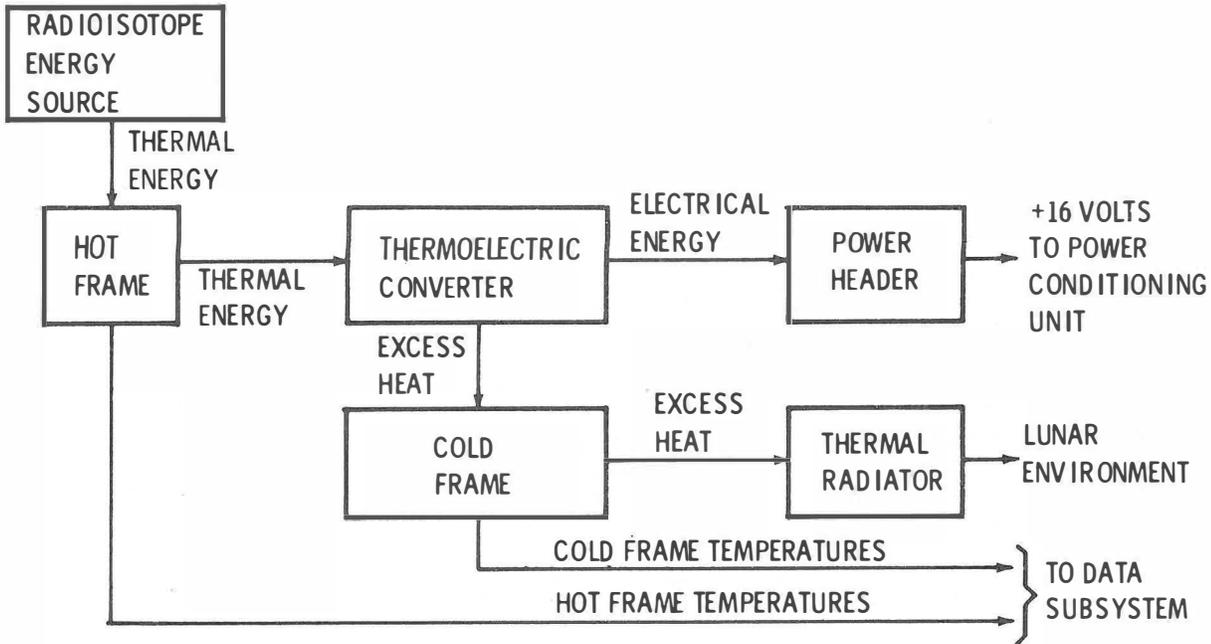
Figure 2-9. EPS Power Generation Function, Block Diagram
