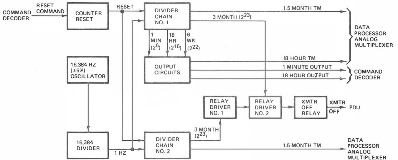
Figure 2-26. Resettable Solid State Timer, Block Diagram
