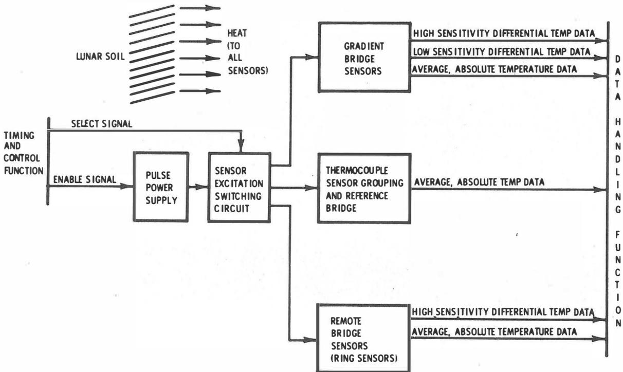
Figure 2-68. HFE Temperature Measurement Function, Block Diagram
