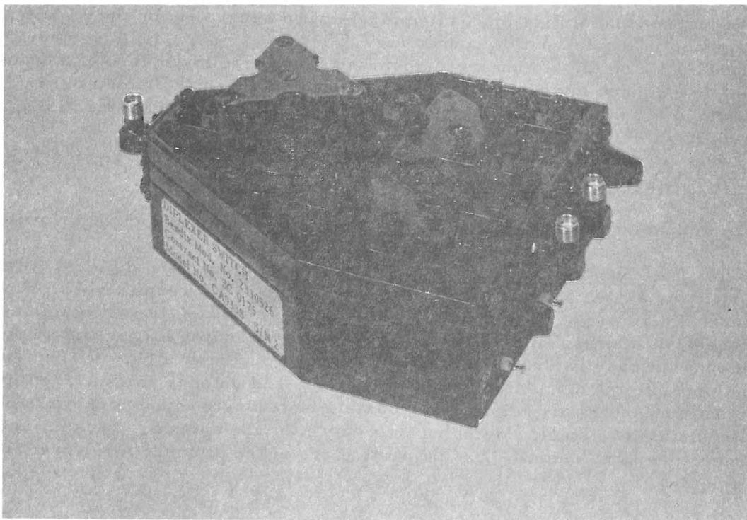
Figure 2-16. Data Subsystem Diplexer Switch
