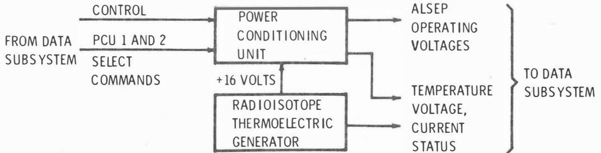
Figure 2-8. Electrical Power Subsystem, Functional Block Diagram
