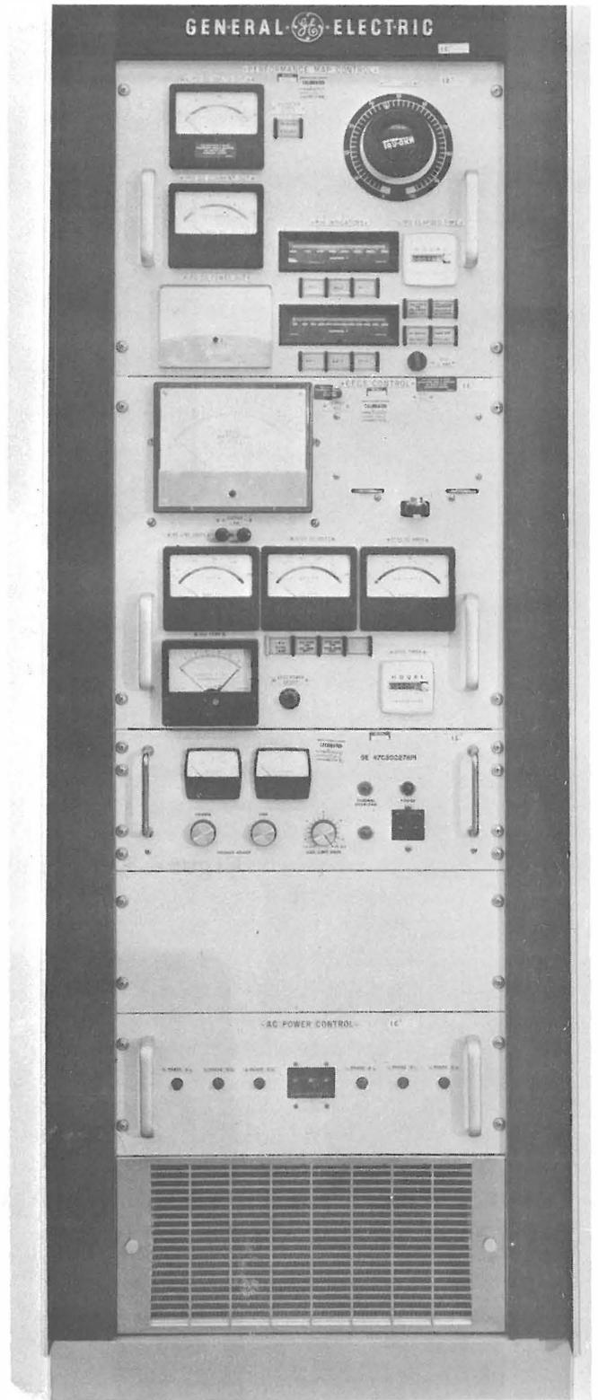
Figure 3-6. Integrated Power Unit Test Set
