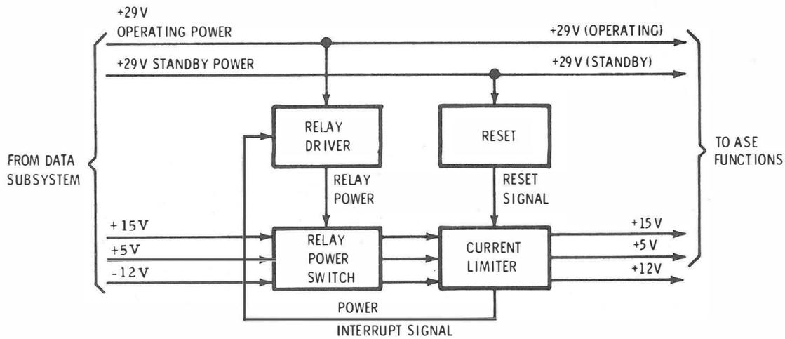
Figure 2-54. ASE Power Control Function, Block Diagram
