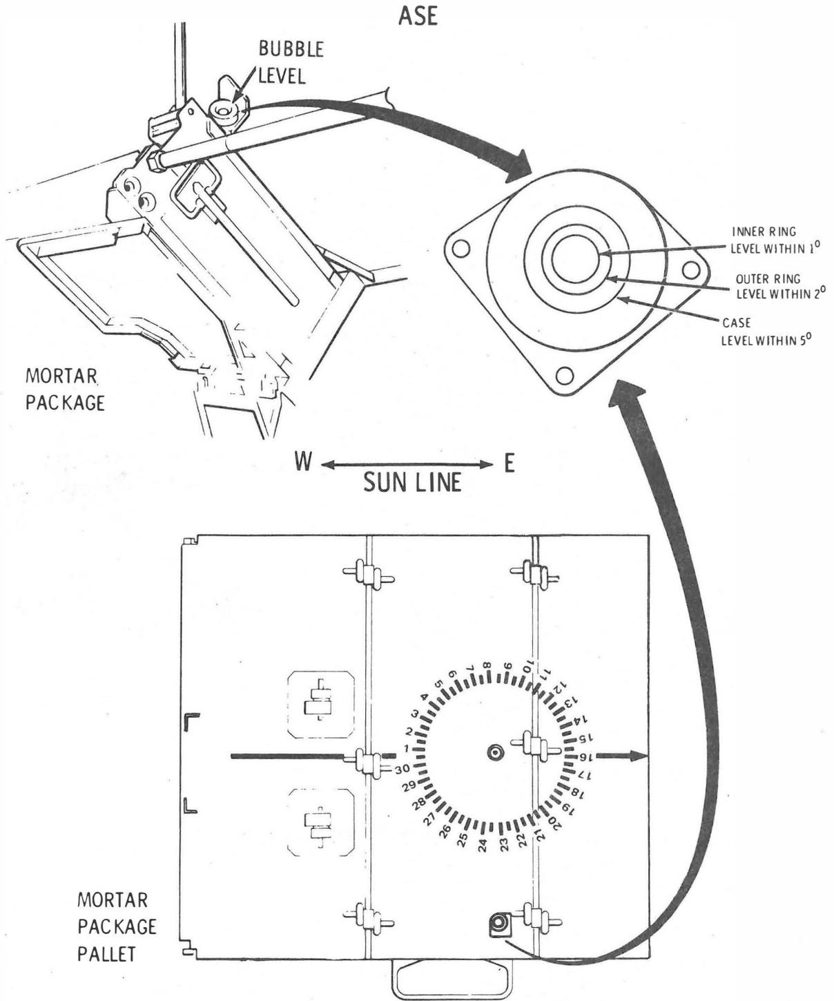
Figure 4-3. Alignment and Leveling Devices (Sheet 6 of 6)
