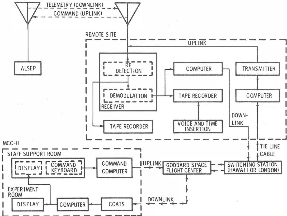
Figure 4-16. MSFN Functional Block Diagram
