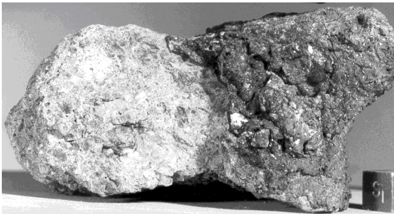
Figure 10: Another view of 67435 showing the extent of glass coating. Cube is 1 cm. NASA S72-43896.
