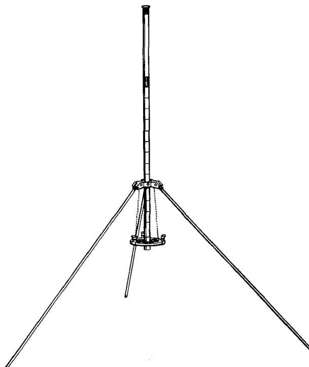
FIGURE 45.—Gnomon. This device is used to provide a physical scale and to calibrate the photometric properties of the samples on the Moon. It can also be seen in figure 46, an Apollo 14 photograph. The long central rod swings freely and indicates the vertical. Its shadow is used to determine direction from the known position of the Sun. The color scale, omitted from this sketch for simplicity, can be seen in other figures.
