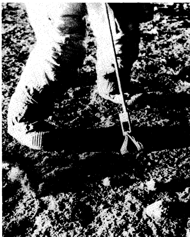
FIGURE 38.—Tongs shown in use on Apollo 12 to collect a small rock. NASA PHOTO S-71-31075.
