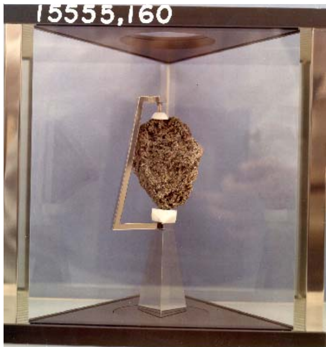
Figure 22: Display case with 1555,160. Case is made from optical glass and filled with dry nitrogen.
