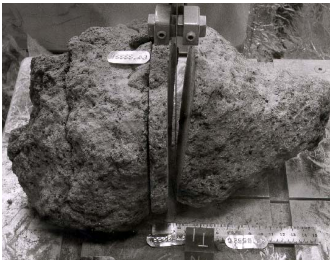
Figure 23: First saw cuts of 15555. Photo number S71-57110. Cube is 1 inch.
