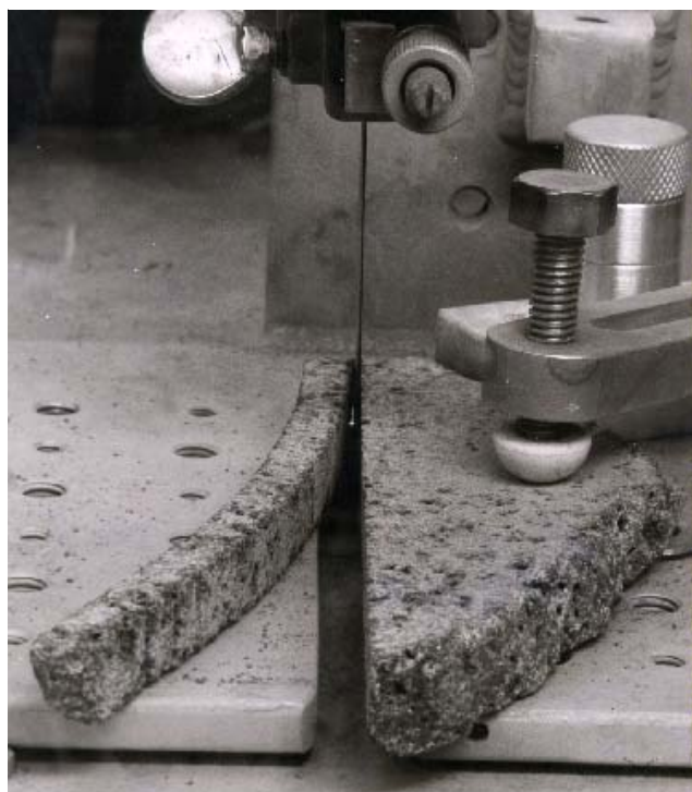
Figure 24: Sawing slab. Photo # S71-57094.
