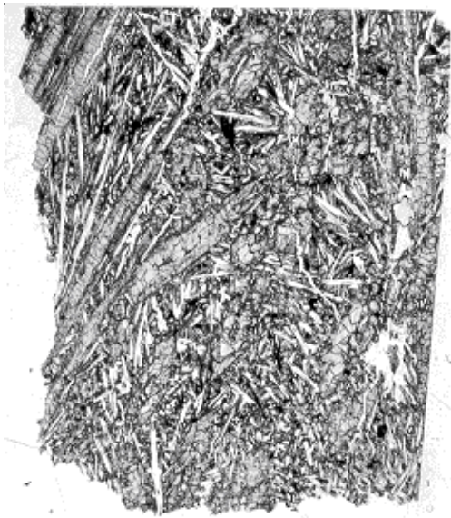
Figure 2: Large scale photo of thin section 15495,92 from the data pack. Scale is 1 cm. Large elongate pyroxene crystals separate regions of subophitic matrix.
