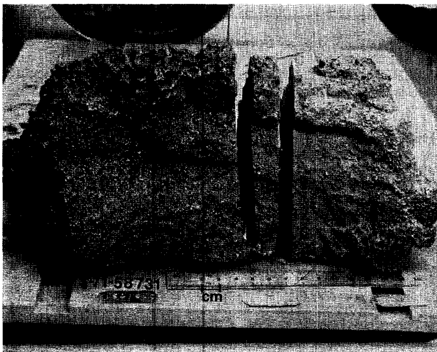
Figure 1. Sawing of 15015, showing vesicular glassy coat.
