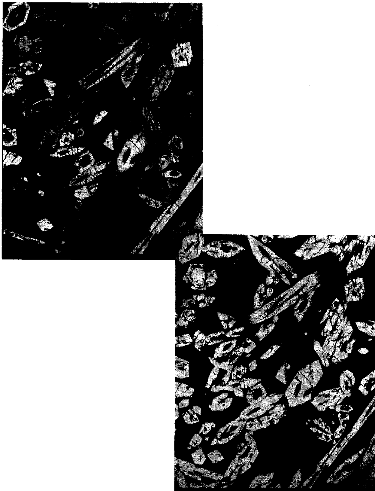
Figure 2. Paired photomicrographs of 15125,7; left, crossed polarizers; right, plane transmitted light. Widths about 1.25 mm.
