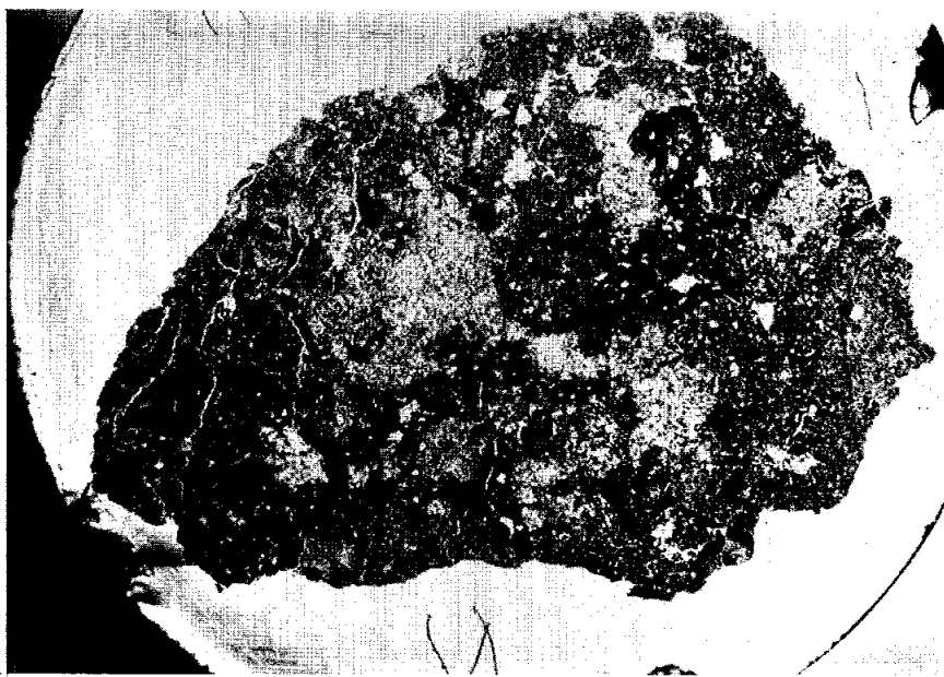
Figure 2. Whole thin section photograph of 15256,47. Transmitted light. Width about 1.5 cm.
