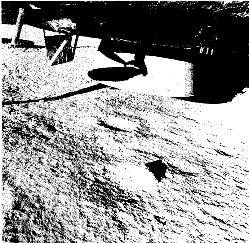
FIGURE 1-10.—The LM-inspection procedure included detailed examination and documentation of the surface materials eroded by the plume of the descent engine. The grooving that indicates radial transport of material from the point below the engine is evident. The erosion did not destroy small craters under the engine bell. The prominent rock in the foreground was later collected as a sample (AS14-66-9261).
