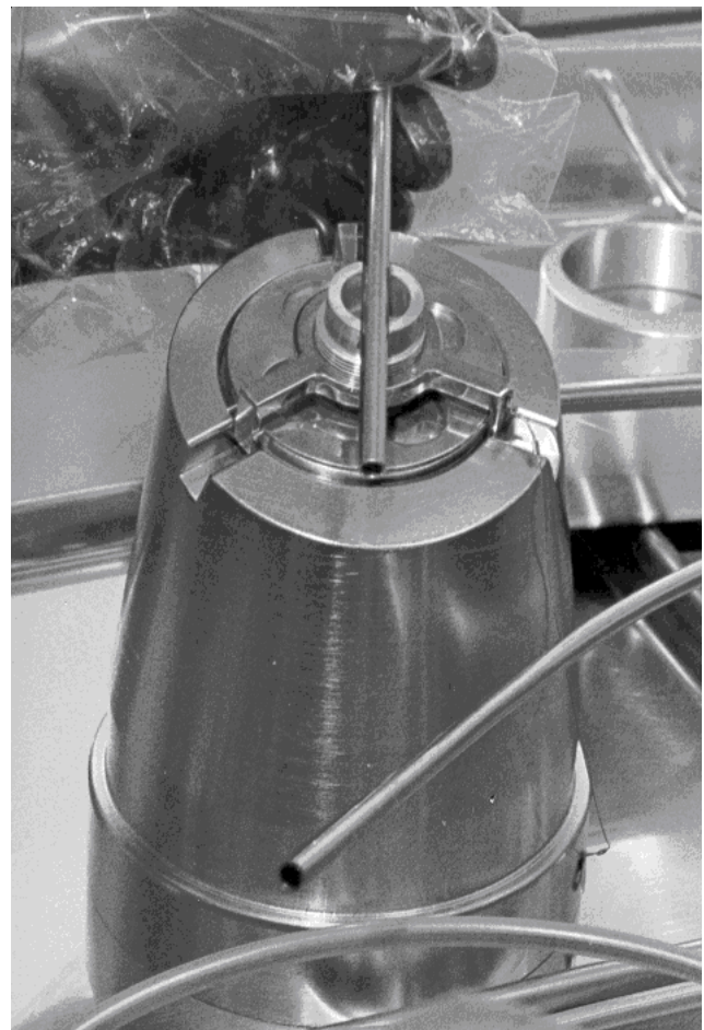
Figure 6: Opening the SESC in the SESC holder at the Berkeley Lab (Burlingame et al. 1971).
