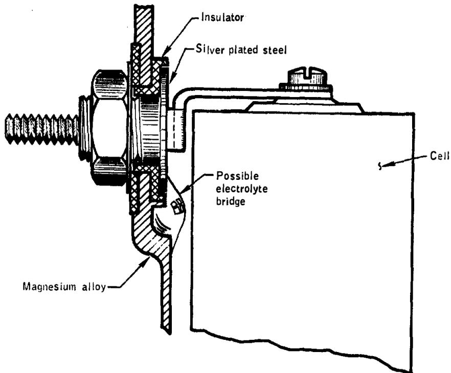
Figure 14-17.- Descent battery terminal configuration.
