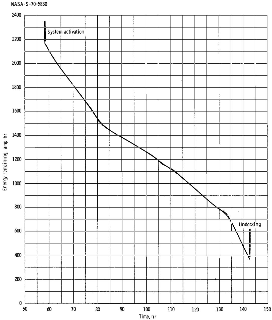
Figure 7.2-2.- Lunar module total battery capacity during flight.
