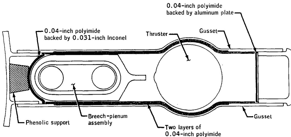
Figure 14-10.- Tunnel gusset protection.
