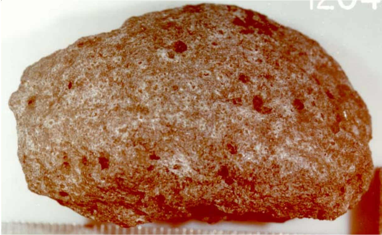
Figure 1: Lunar basalt 12043,0 showing zap pits and rounded surface. Sample is 4 cm. NASA # S94-035810.
