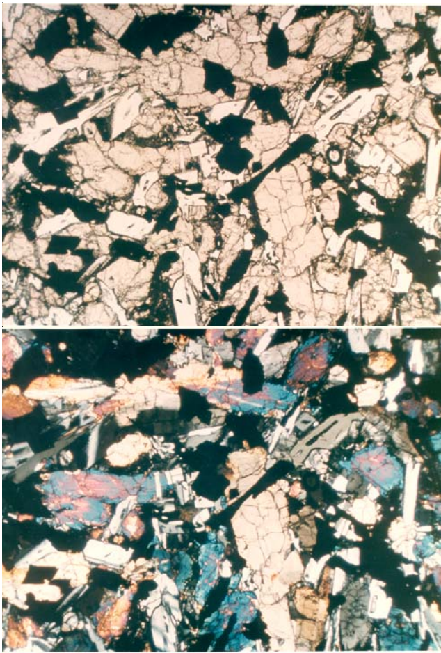
Figure 2: Photomicrographs of thin section of 10024 showing medium-grained basaltic texture. Field of view is 2.5 mm. NASA S70-49977 and 978.
