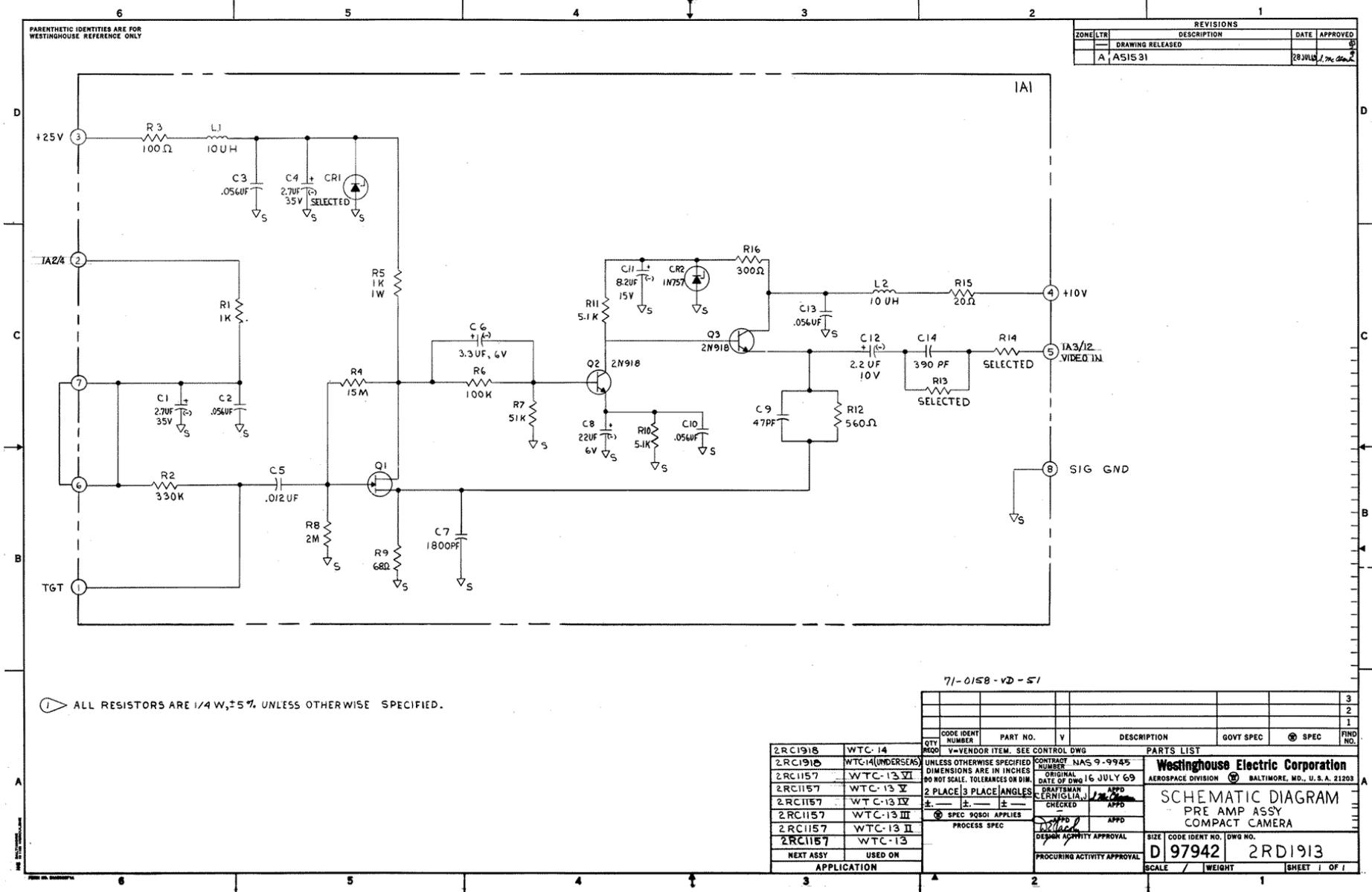
Figure 14. Preamplifier Schematic
