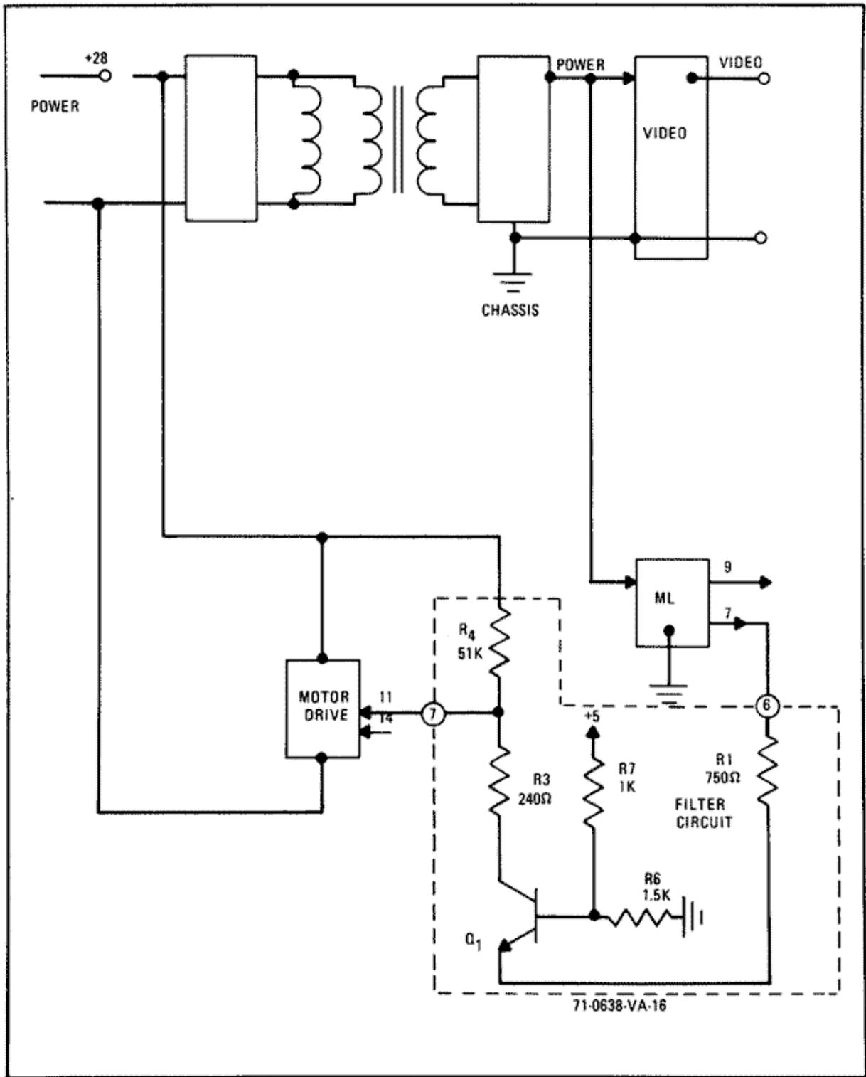
Figure 23. Filter Circuit Block Diagram
