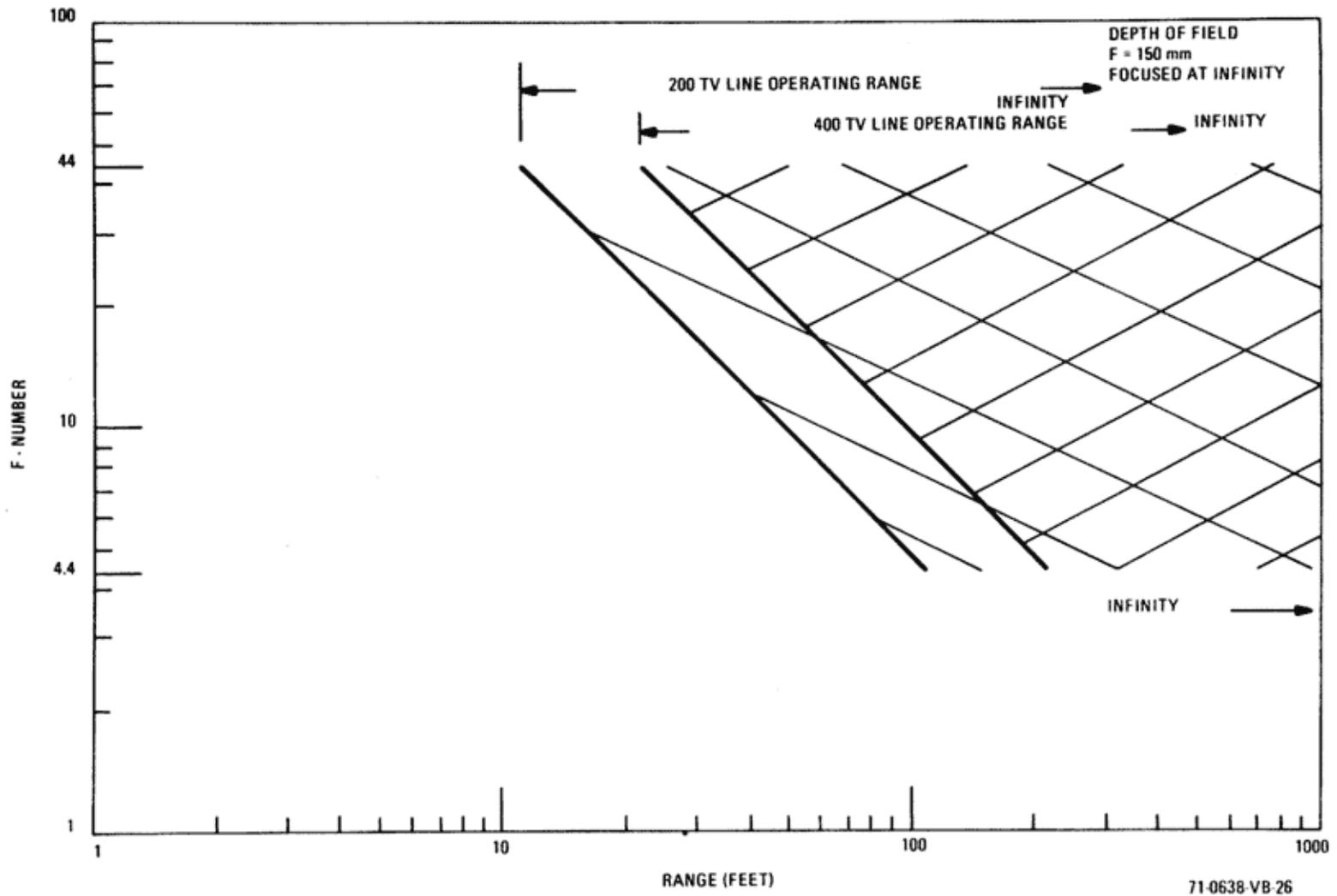
Figure 9C. Lens Depth of Field vs Zoom (150 mm)
