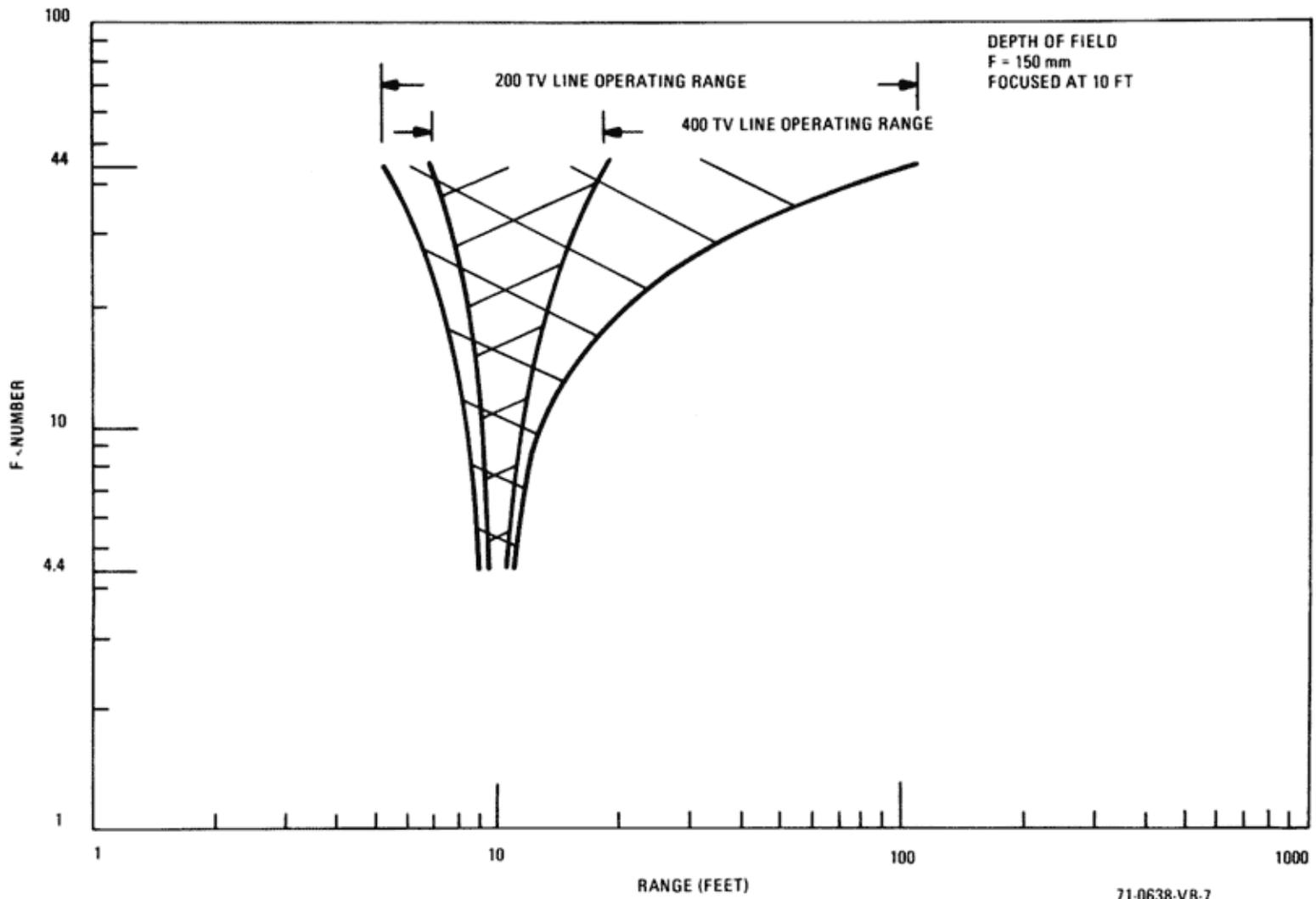
Figure 9B. Lens Depth of Field vs Zoom (150 mm)
