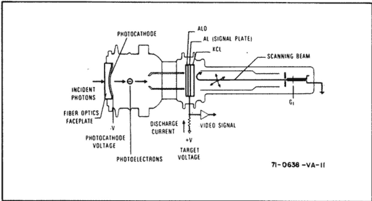
Figure 13. SEC Image Tube Layout
