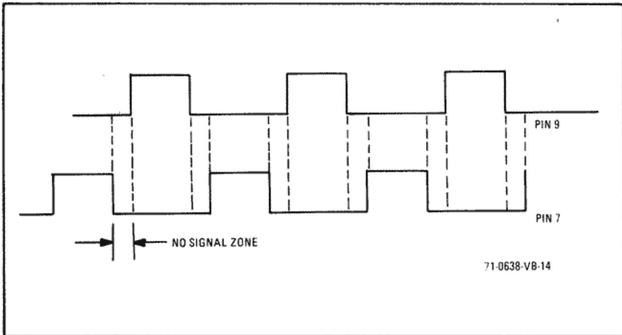
Figure 21b. Motor Input Signal Duty Cycle
