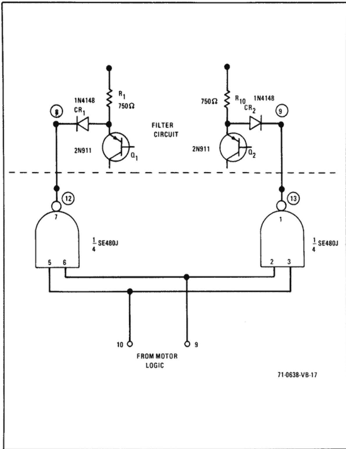
Figure 24. Fail Safe Circuit Schematic
