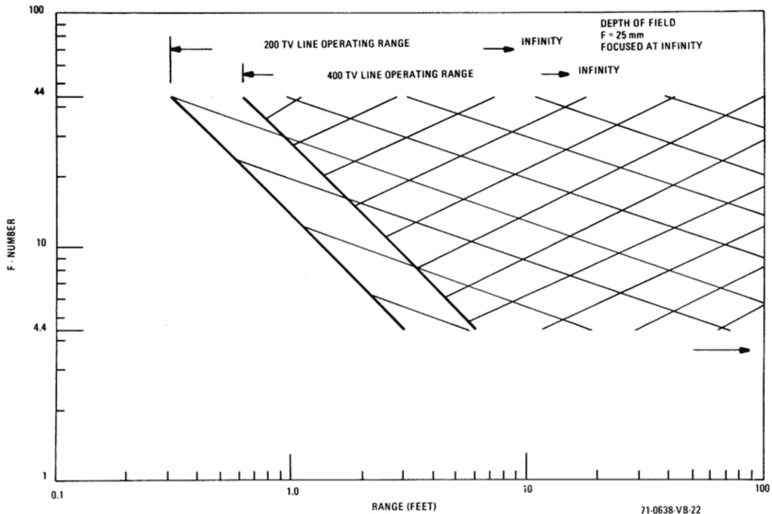
Figure 7C. Lens Depth of Field vs Zoom (25 mm)
