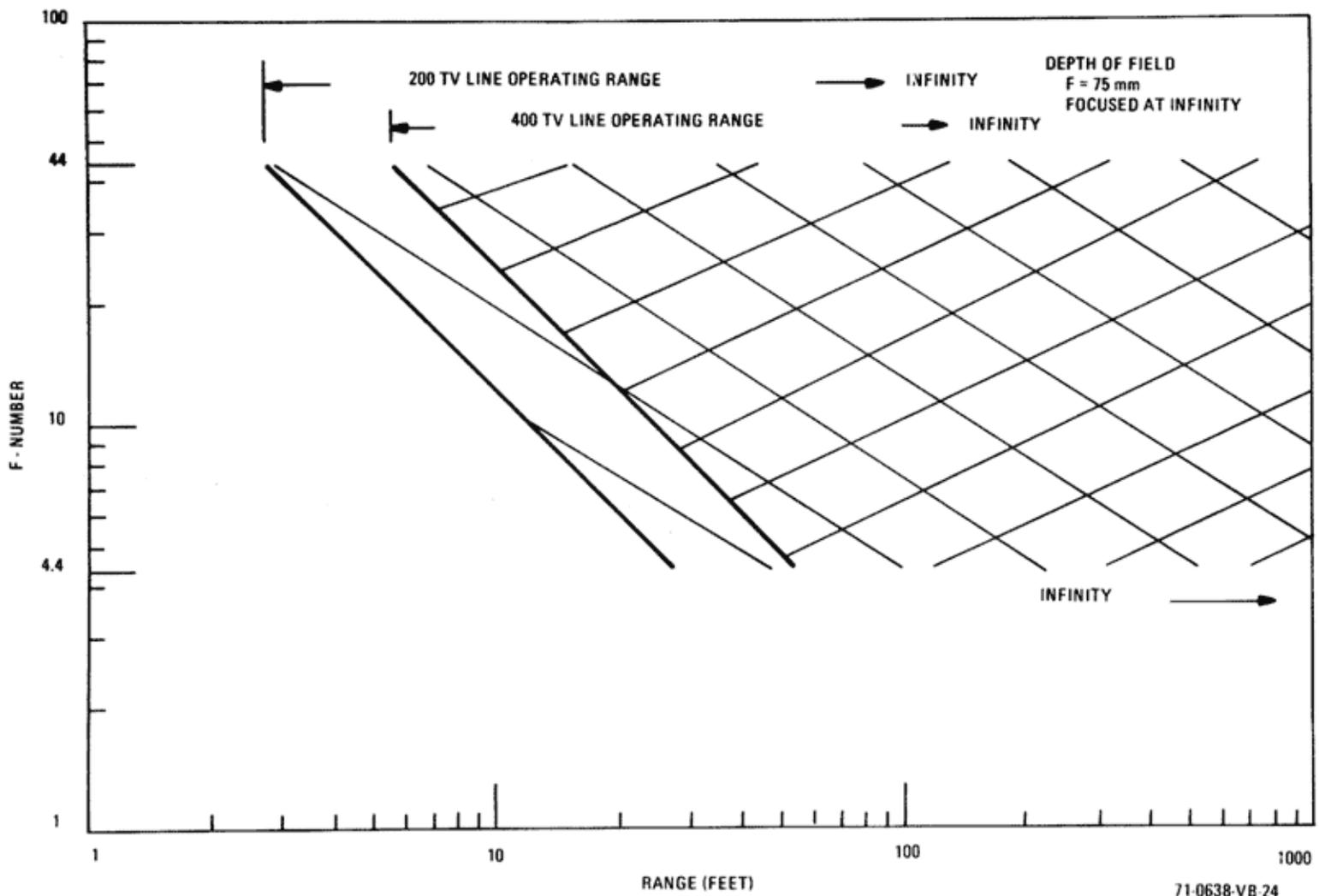
Figure 8C. Lens Depth of Field vs Zoom (75 mm)
