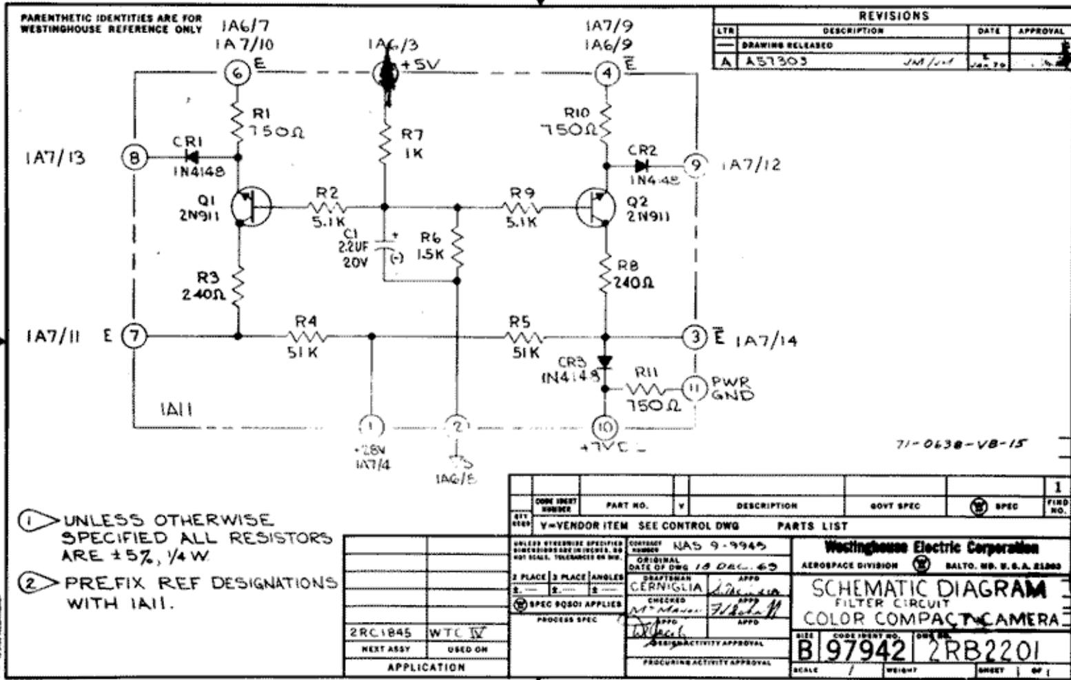
Figure 22. Filter Circuit Schematic
