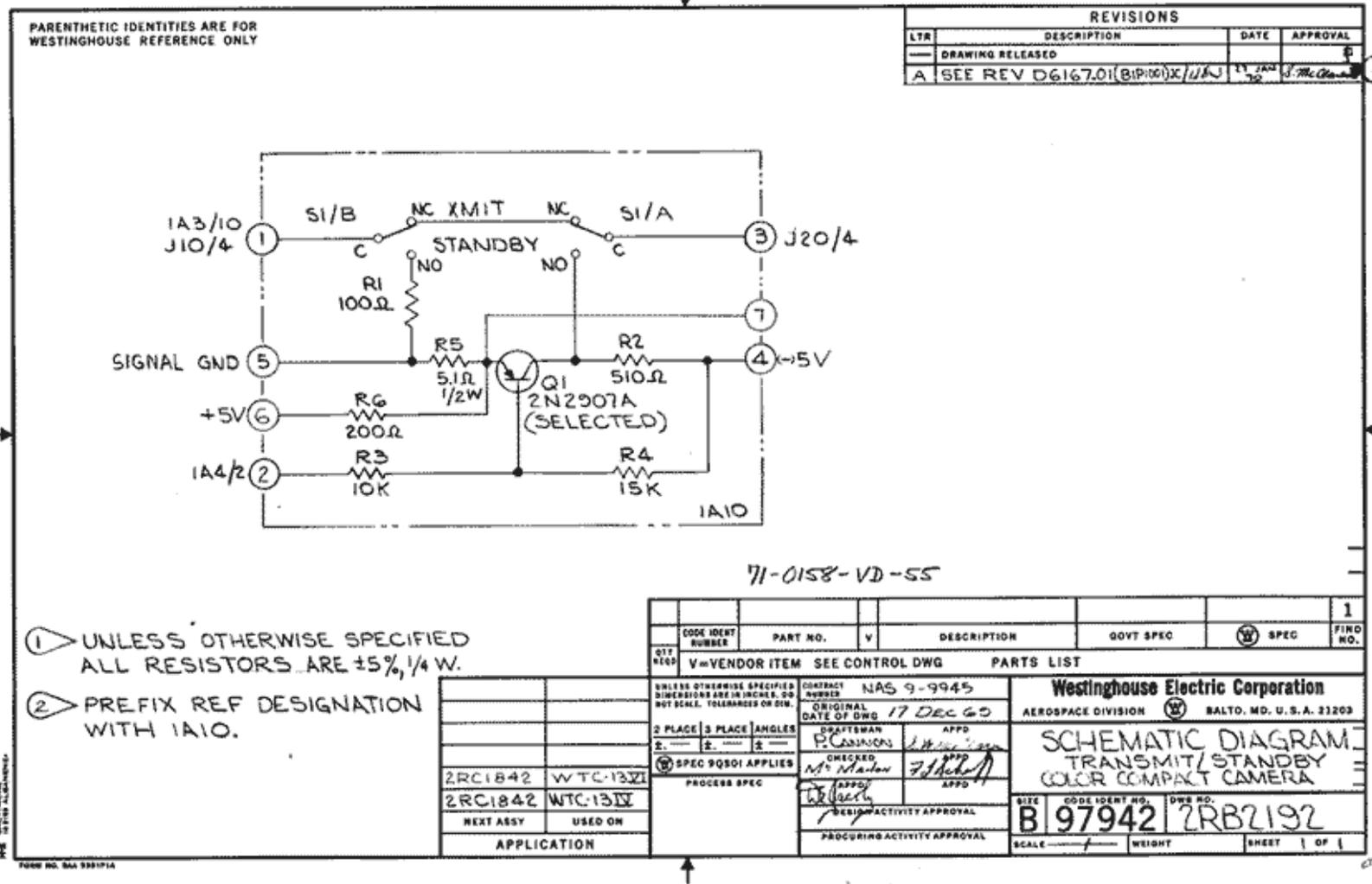
Figure 18. Transmit/Standby Switch Schematic
