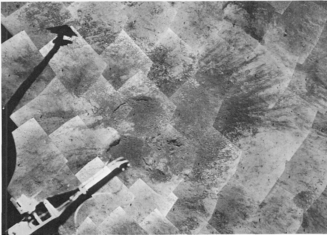
FIGURE 4-25.—Mosaic of computer-processed pictures, showing crushable block 1 impact area and soil disturbance caused by Surveyor VI vernier engine 1 during the hop (Nov. 15 and 16, 1967, Catalog 6-SE-43A).
