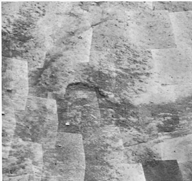
FIGURE 4-23.—Mosaic of computer-processed pictures, showing rays of fine, dark soil deposited by Surveyor V vernier engine 2 during the hop (Nov. 15 and 16, 1967, Catalog 6-SE-43C).
