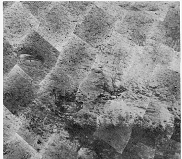
FIGURE 4-24.—Mosaic of computer-processed pictures, showing imprints of footpad 3 and crushable block 3 made during the initial landing and soil disturbance caused by Surveyor VI vernier engine 3 during the hop (Nov. 15 and 16, 1967, Catalog 6-SE-43B).
