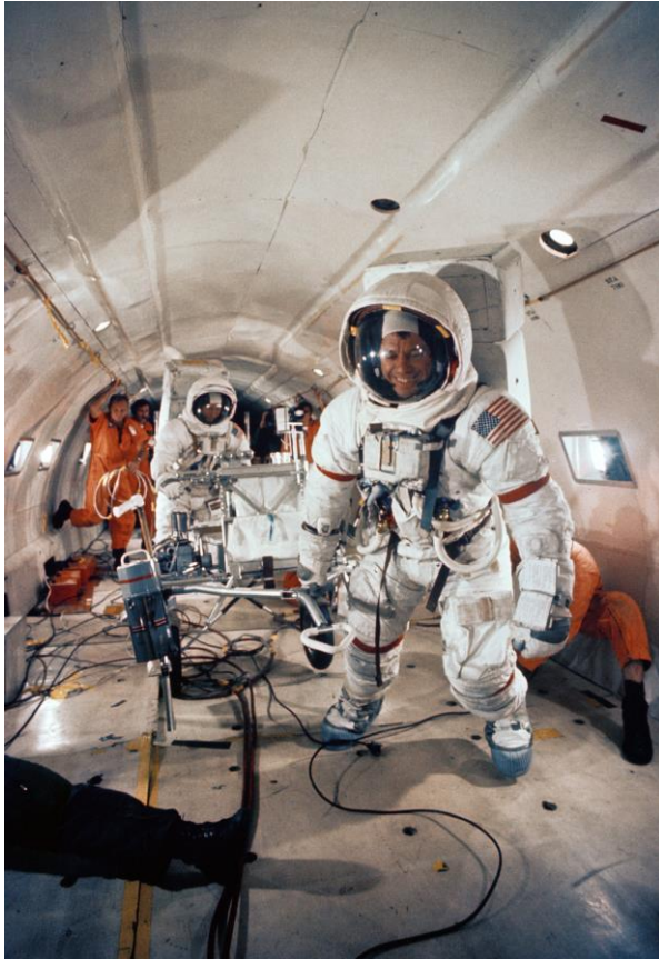
Figure 12. Alan Shepard trains for the Apollo 14 mission under 1/6 g on the KC-135. This test allowed him to simulate pulling the equipment transporter under similar gravity conditions as exist on the lunar surface. (NASA photo S70-53480)
