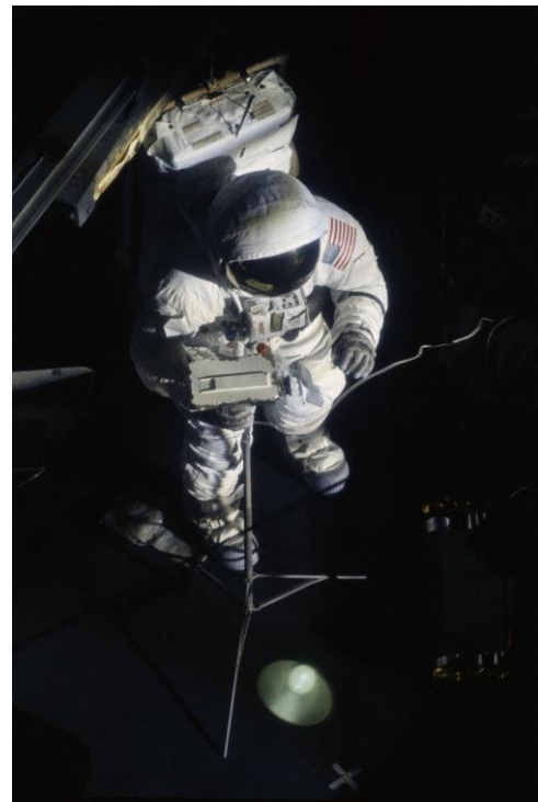
Figure 14. Suited test of the deployment of a lunar television camera while using the partial gravity (POGO) system to simulate 1/6 g. Note the attachment at the top of the unit to support most of the subject's weight. (NASA photo S71-16442)
