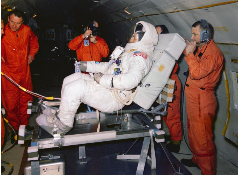
Figure 13. Astronaut Joe Engle testing the ability of the driver to move about adequately while driving the Lunar Rover under 1/6 g on the KC-135. (NASA photo S70-27154)
