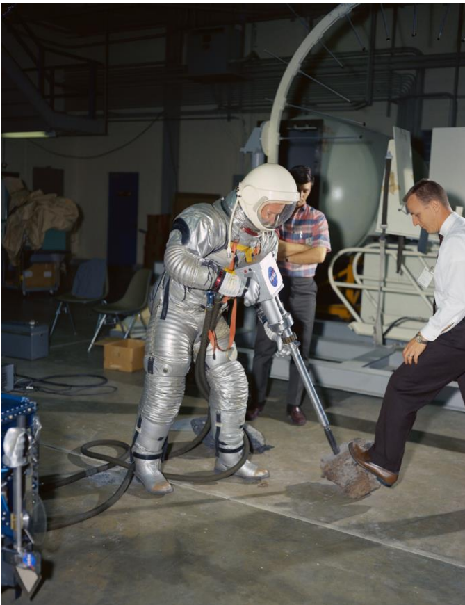
Figure 7. Uel Clanton conducting a suited test of an early version of the lunar drill in one of the Building 9 test facilities at the Manned Spacecraft Center. (NASA photo S66-20212)
