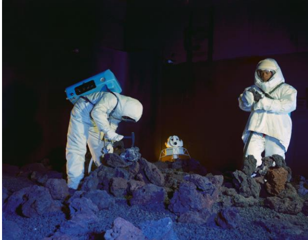
Figure 3. The "Moon Room" in one of the buildings at Ellington Air Force Base. Simulated lunar surface conditions and lighting were used to test the astronauts' abilities under lunar lighting conditions. This facility was used during 1963 and 1964 until the new facilities were available at the Manned Spacecraft Center in 1965. (NASA photo S64-23391)
