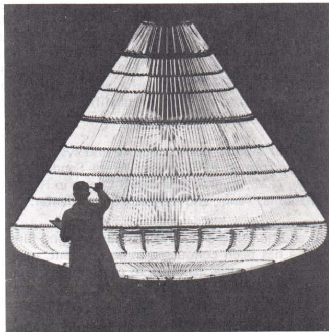
Oven-freezer tests CM structural strength by roasting one side at 600° while dousing other side with liquid nitrogen at
