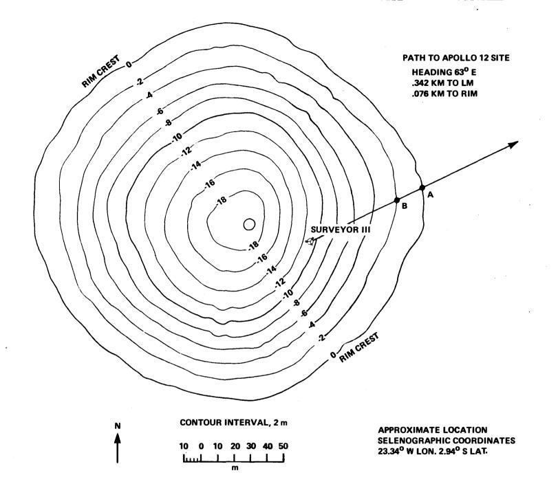
FIGURE 1 - CONTOUR MAP OF SURVEYOR III LANDING SITE PREPARED FROM PHOTOCLINOMETRIC PROFILES DERIVED FROM LUNAR ORBITER III PHOTOGRAPH H154, FRAMELET 27 (PHOTOCLINOMETRY BY H. E. HOLT AND S. G. PRIEBE) (FROM REFERENCE 2)
