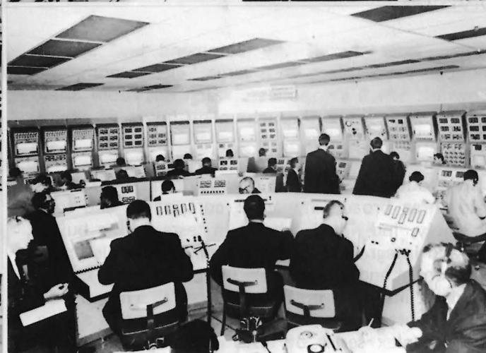
P-276 *Checkout at Downey; technicians check cabling to command and service modules (left), while others monitor responses to stimuli on battery of computerized display equipment*
