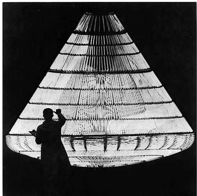
*Oven-freezer tests CM structural strength by roasting one side at 600° while dousing other side with liquid nitrogen at 320° below zero*
