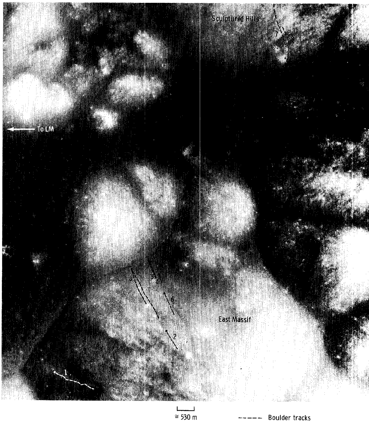
FIGURE 8-12.—Locations of boulder tracks on the East Massif and on the Sculptured Hills. For tracks identified by a letter, a definite causative boulder could be located; for tracks identified by a number, only the most probable causative boulder could be located.
