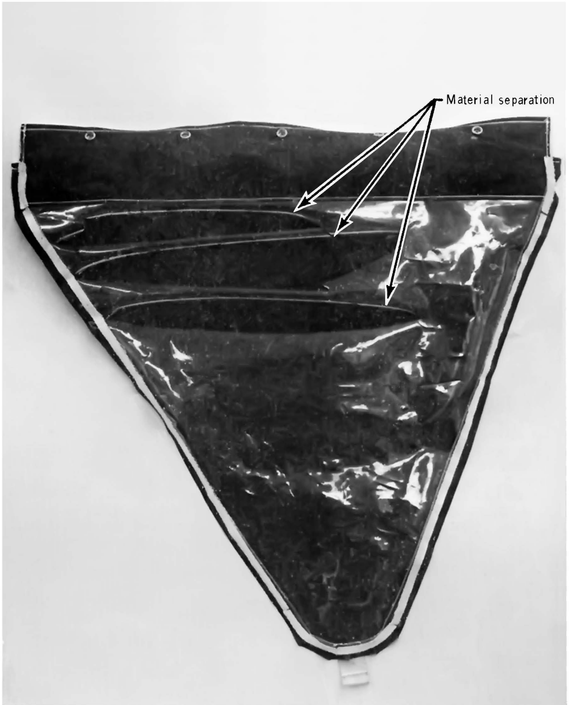
Figure 15.- Cracked left-hand window shade.
