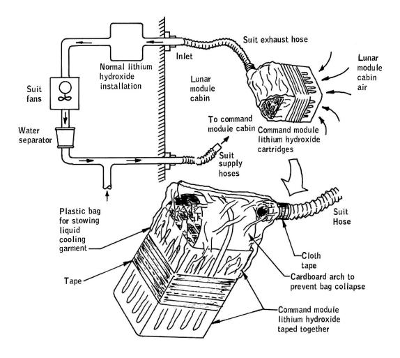
Figure 1.- Supplemental carbon dioxide removal system.
