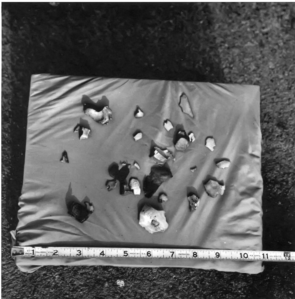
Figure F3.5-13.- Parts of probe insulator and tubing collected from area around test chamber.
