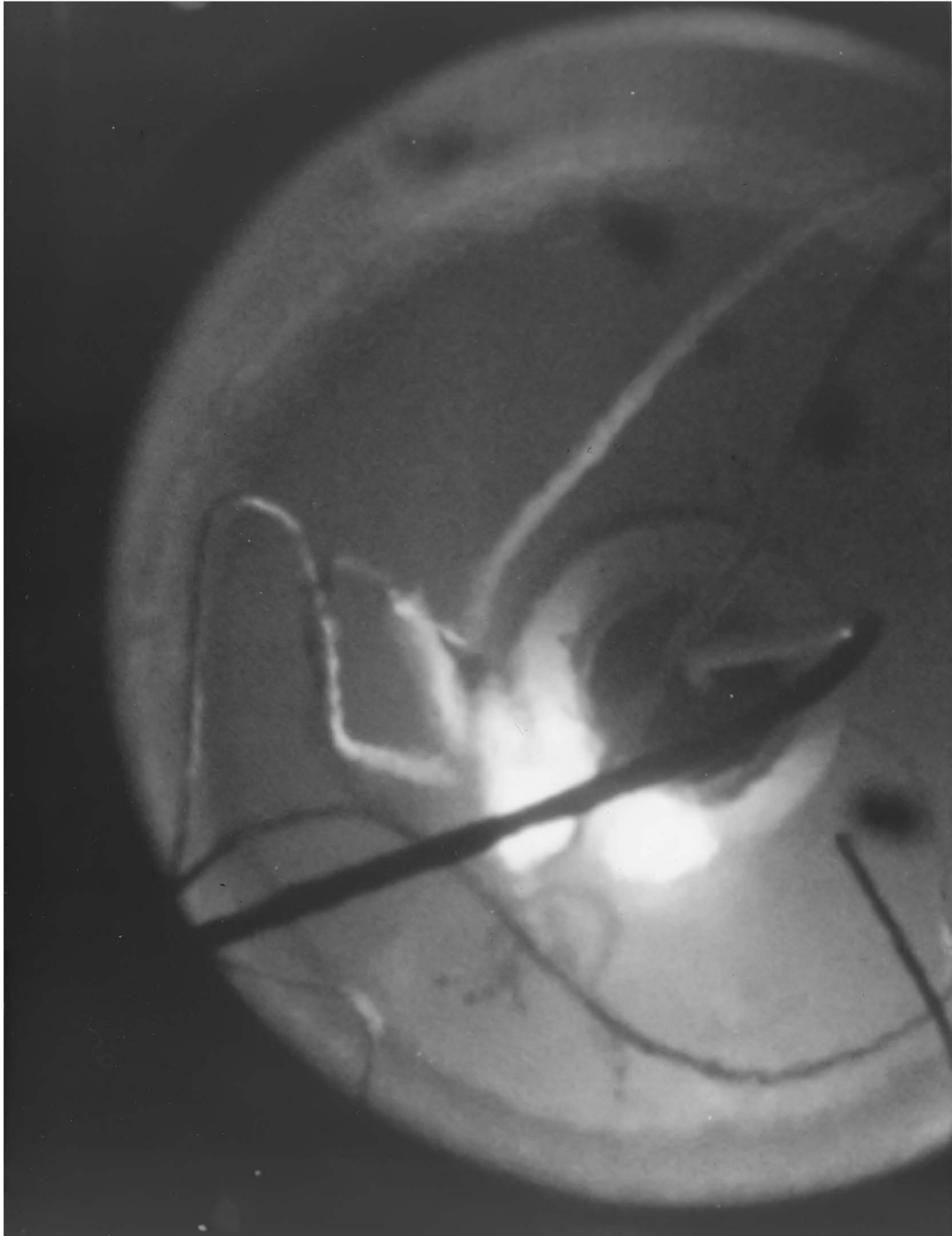
Figure F3.5-8.- Burning of adjacent wire bundles.
