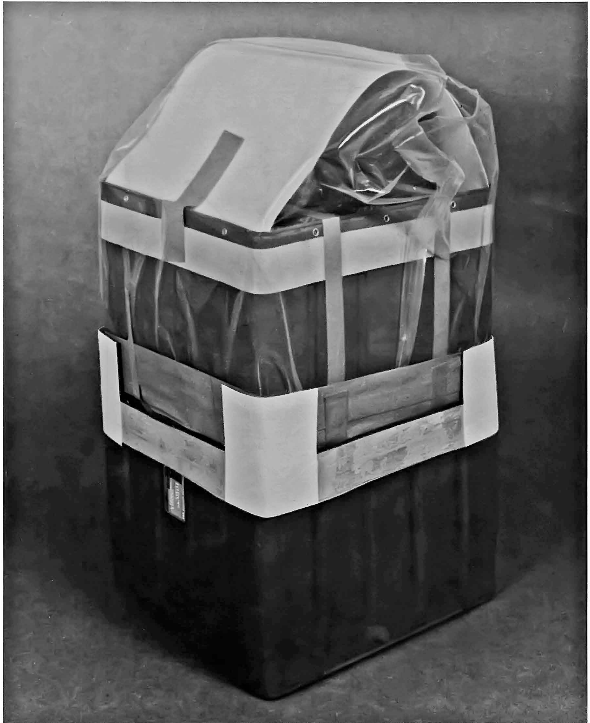
Figure 4-16.- Lithium hydroxide canister modification.
