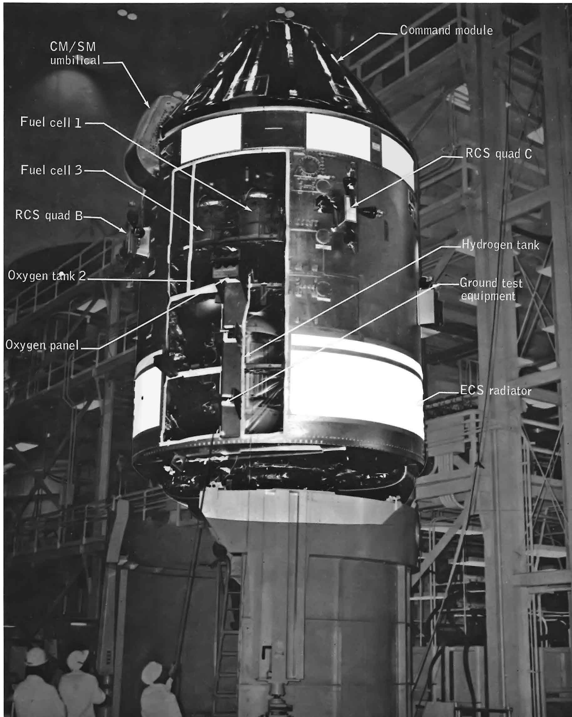
CSM in ground test with bay 4 panel removed.
