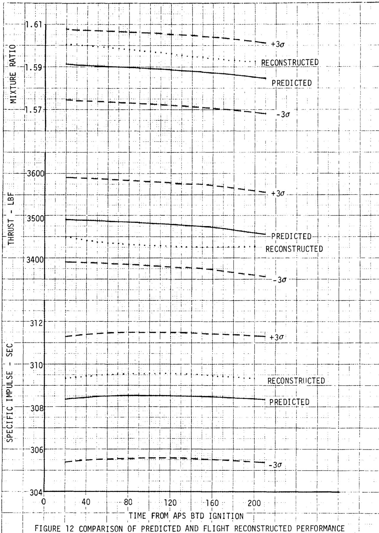
FIGURE 12 COMPARISON OF PREDICTED AND FLIGHT RECONSTRUCTED PERFORMANCE
