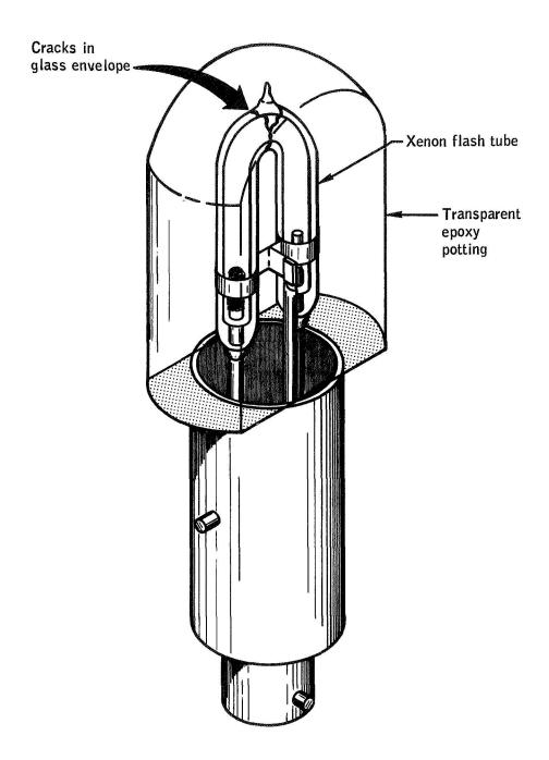
Figure 1.- Lamp assembly showing area of failure.
