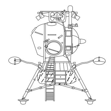
Figure 1-16. L3 lunar lander. The flat, downward-facing face (left) of the ovoid pressure cabin holds the round viewport (not visible). The Kontakt system passive unit is at cabin top, and two landing radar booms extend at left and right. Nozzles of two solid-fueled hold-down rockets are visible at the tops of the legs, near the bases of the radar booms.
