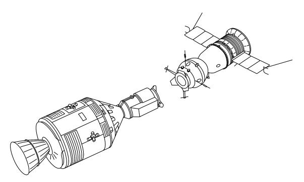
Figure 1-23. Apollo and Soyuz join in space. Note the docking module (DM) attached to Apollo's nose. The DM was stored for launch within a shroud between the CSM and the S-IVB second stage of the Apollo Saturn IB launch vehicle. In orbit the Apollo inserted its probe unit into the standard Apollo drogue unit of the docking module, extracted the DM from the S-IVB, then performed rendezvous and docking with the Soyuz spacecraft.
