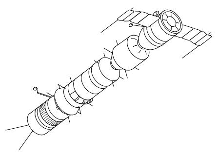
Figure 1-5. Soyuz A-B-C circumlunar concept. The drawing shows Soyuz-A (right), Soyuz-B booster, and Soyuz-C tanker with twin whip antennae (left).
