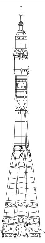
Figure 1-7. Soyuz rocket. With more than 1000 launches to its credit since 1963, the two-and-a-half-stage Soyuz rocket has flown more than any other. Propellants are liquid oxygen and kerosene. Weight of payload launched to 200-km, 51° circular orbit is 7000 kg.
