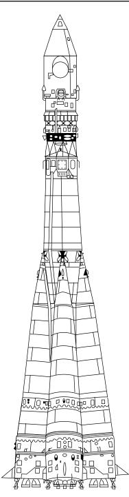
Figure 1-3. Vostok rocket. This is a two-and-a-half-stage derivative of the one-and-ahalf-stage rocket which launched Sputnik 1 (1957). Its original ancestor was the SS-6 "Sapwood" ICBM. It served as the basis for the Soyuz launcher (figure 1-7), in service today. Weight of payload launched to 200-km, 51° circular orbit is 4730 kg.
