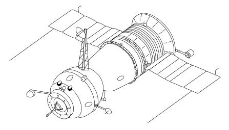
Figure 1-18. Salyut 1-type Soyuz. This was the Original Soyuz upgraded for Salyut space stations. The probe and drogue docking system (left) permitted internal transfer of cosmonauts from the Soyuz to the station.
