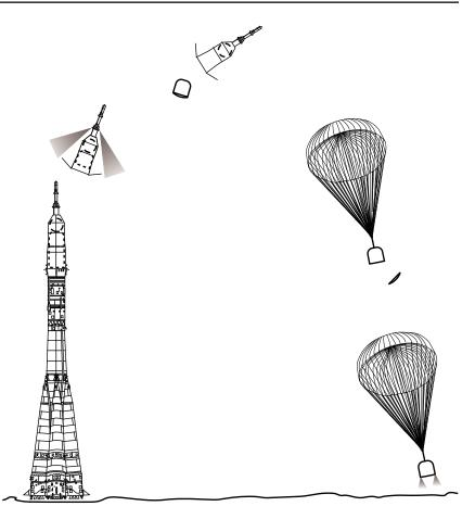
Figure 1-29. Soyuz launch pad abort sequence. The modules of the Soyuz spacecraft are shown beneath the launch shroud by dashed lines. Note the separation plane between the Soyuz descent and service modules.
