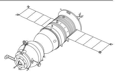
Figure 1-30. Soyuz-TM spacecraft. Compare the antennae on the orbital module to those on Soyuz-T. Differences reflect the change from the Igla rendezvous system used on Soyuz-T to the Kurs rendezvous system used on Soyuz-TM.
