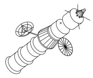
Figure 1-2. L1 Soyuz manned circumlunar concept (1962). Should not be confused with the L1 (Zond) spacecraft (figure 1-9). The cone at the front (right) of the L1 Soyuz is an attitude control module; behind it are cylindrical orbital and descent modules, and a frustum-shaped service module. The round appendage (right) is a solar array, and the dish, a high-gain antenna. At the rear of the L1 are three booster modules.
