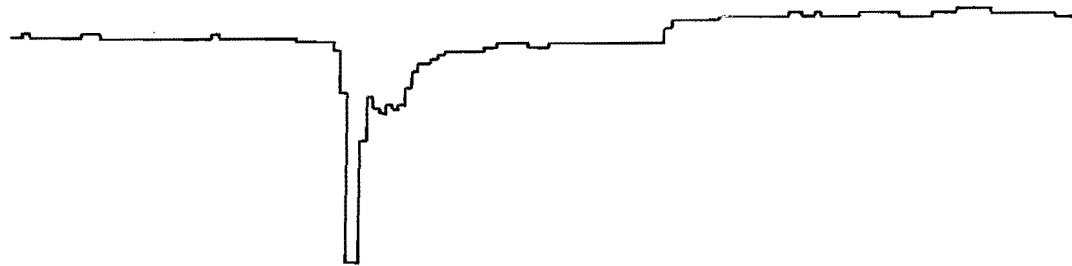
D. Test, result of applying localized flame on gas chromatograph signal wire.
