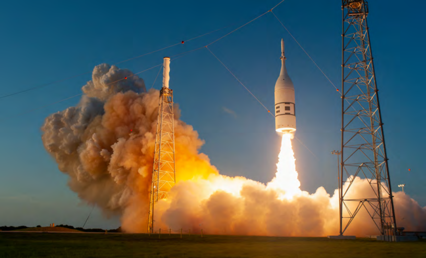
▲ A fully functional launch abort system with a test version of Orion attached launches on NASA's Ascent Abort-2 atop a booster provided by Northrop Grumman on July 2, 2019, from Launch Pad 46 at Cape Canaveral Air Force Station in Florida. Image credit: NASA
