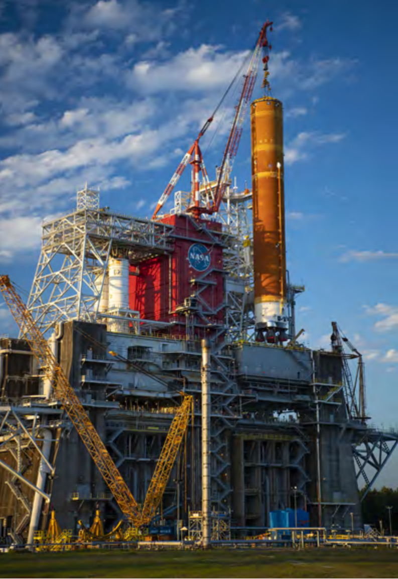
▲ Following a successful Green Run hot fire test at Stennis on March 18, 2021, teams lift the first core stage of the agency's SLS rocket from the B-2 Test Stand. Image credit: NASA
