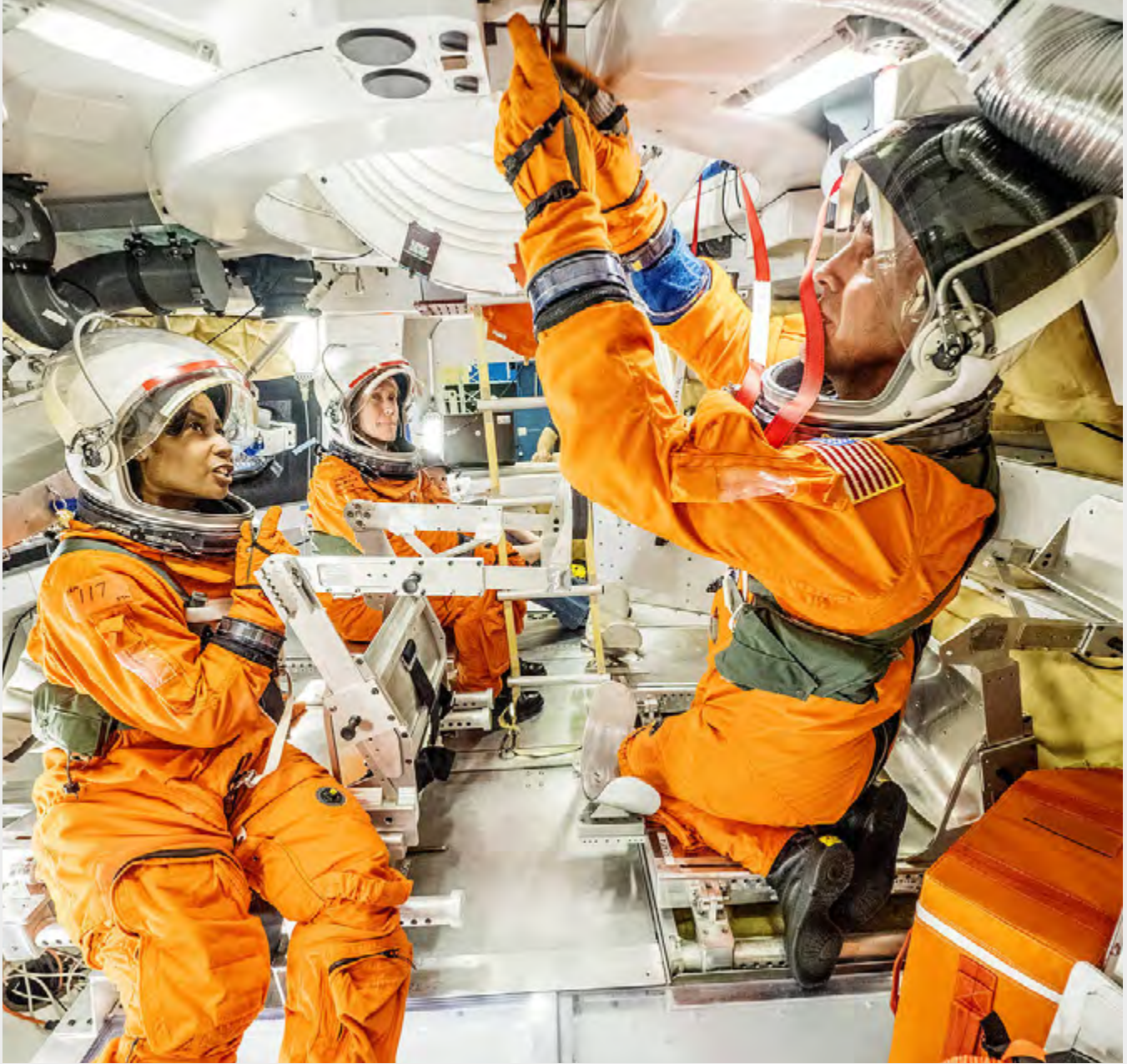
▲ Astronauts Stephanie Wilson, Karen Nyberg, and Rick Mastracchio (left to right) assist in testing the docking hatch on a representative model of the Orion spacecraft at Johnson Space Center. Image credit: NASA
