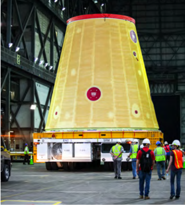
▲ In High Bay 4 of the VAB at Kennedy Space Center, pathfinders, or full-scale replicas of SLS solid rocket booster segments, are stacked during a training exercise on Jan. 8, 2020. Image credit: NASA
