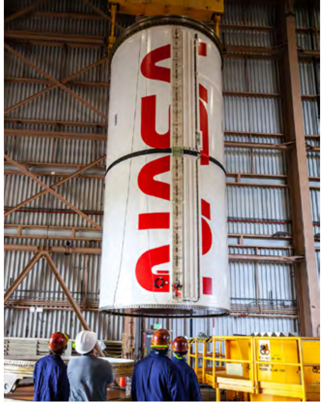
▲ The NASA “worm” livery and black-and-white photogrammetric markings are visible on completed solid rocket motor segments. Image credit: NASA
