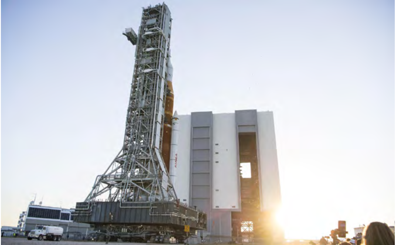
▲ NASA's mobile launcher, atop Crawler-Transporter 2, moves into High Bay 3 at the Vehicle Assembly Building (VAB) on Sept. 8, 2018, at Kennedy Space Center. Image credit: NASA
