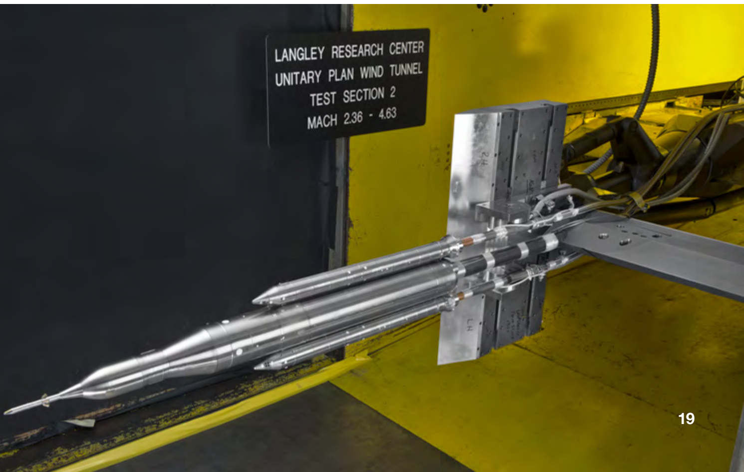
▼ A model of SLS is tested in the Unitary Plan Wind Tunnel at Langley using high-pressure air blown through the solid rocket boosters to simulate the booster separation motors' firing. Image credit: George Homich
