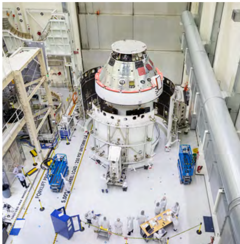
▼ Engineers work to fit three spacecraft adapter jettison fairing panels onto Orion's service module inside Kennedy's Neil Armstrong Operations and Checkout Building on Oct. 13, 2020. Image credit: NASA
