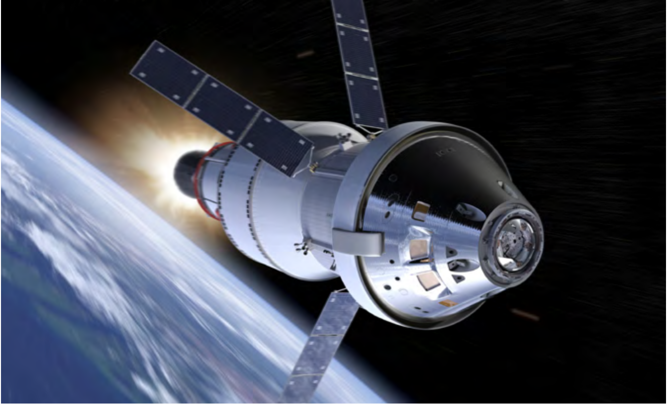
▼ An artist's impression of the Orion spacecraft with ESA's service module. The module sits directly below Orion's crew capsule and provides propulsion, power, thermal control, and water and air for four astronauts. The solar array spans 19 m and provides enough power for two households. Image credit: NASA
