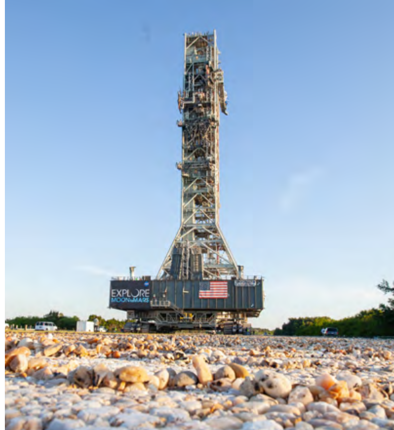
▲ NASA's' mobile launcher makes a solo trek along the crawlerway atop Crawler-Transporter 2 to Kennedy's Launch Complex 39B on June 27, 2019. Image credit: NASA
