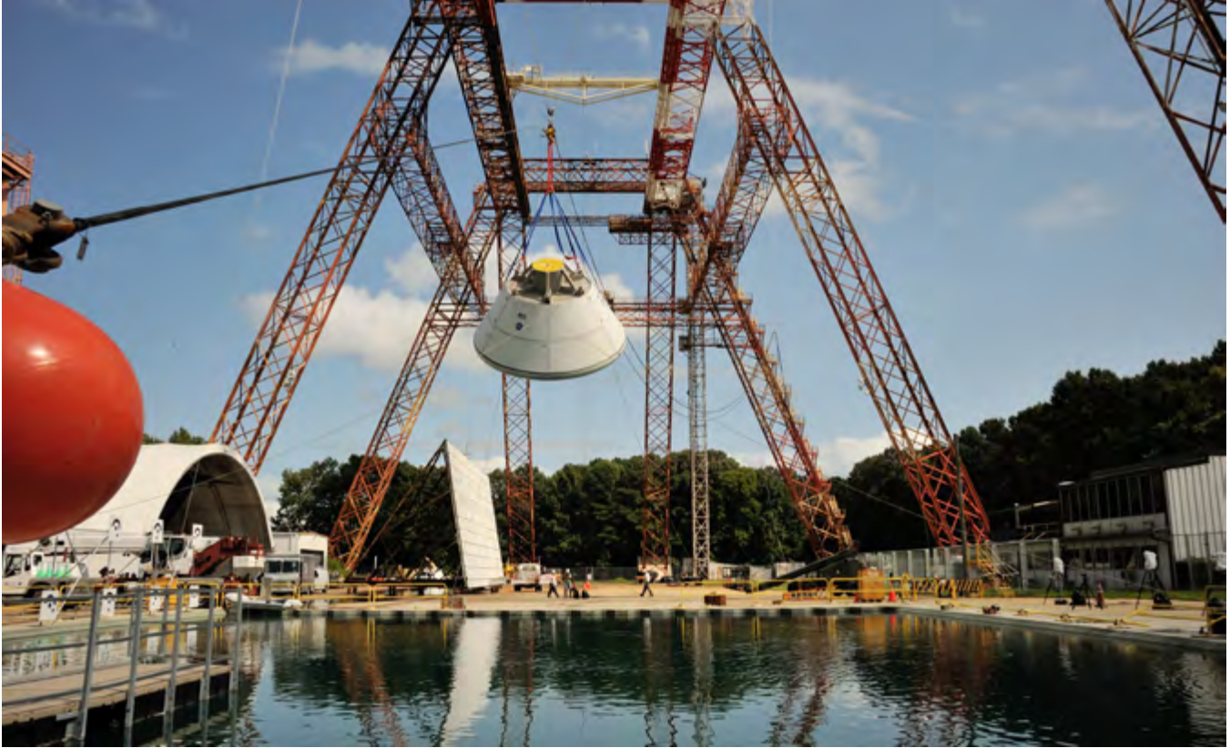
▲ Teams conduct a vertical drop test of an Orion test article as part of water-impact testing at the Hydro Impact Basin at Langley’s Landing and Impact Research Facility. Image credit: NASA
