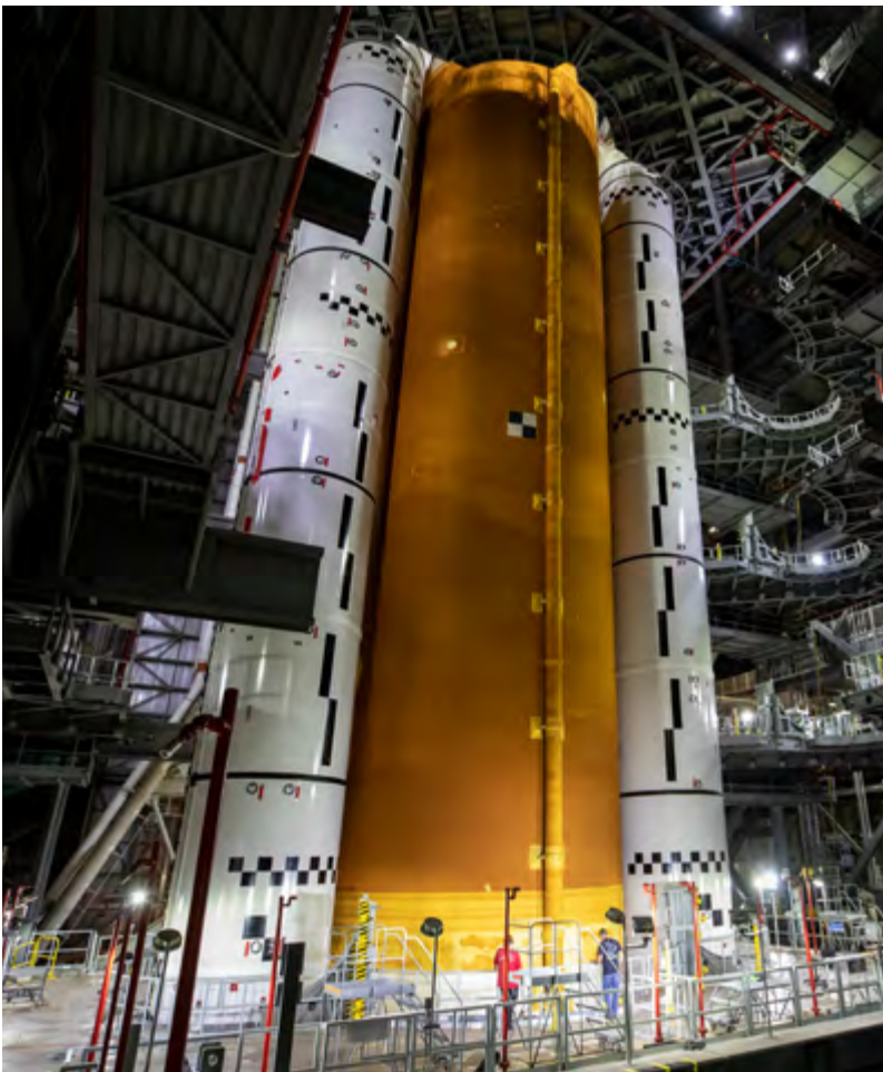
▲ The SLS core stage is shown atop the mobile launcher inside High Bay 3 of the VAB at NASA's Kennedy Space Center on June 12, 2021. Image credit: NASA
