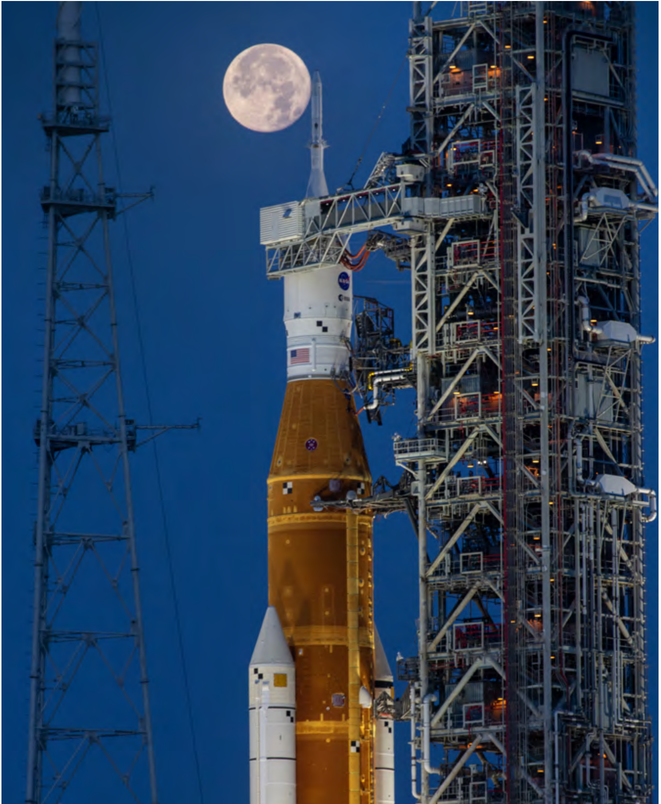
▲ A full Moon is in view from Launch Complex 39B at NASA's Kennedy Space Center in Florida on June 14, 2022. The Artemis I Space Launch System (SLS) and Orion spacecraft, atop the mobile launcher, were being prepared for a wet dress rehearsal to practice timelines and procedures for launch. Image credit: NASA
