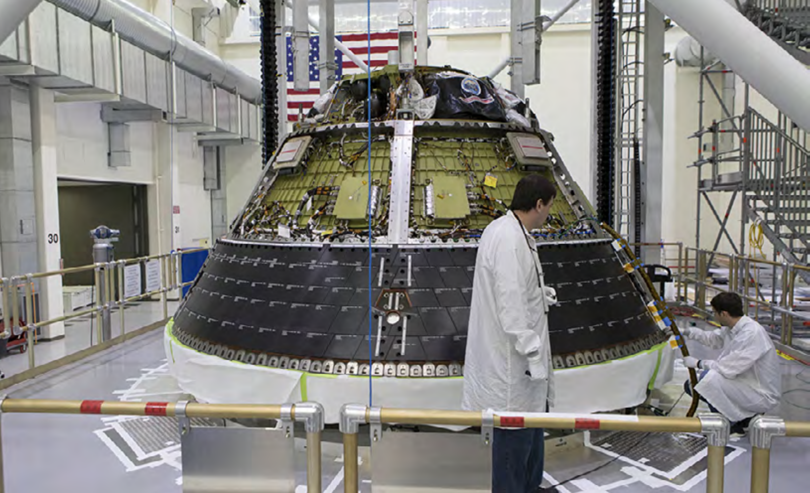
▲ Lockheed Martin technicians test the fitting of the Orion spacecraft's heat shield back shell panels inside the Neil Armstrong Operations and Checkout Building high bay at NASA's Kennedy Space Center in Florida. The back shell panels serve as the outer layer of the spacecraft and will protect it against the extreme temperatures of re-entry from deep space. Image credit: NASA
