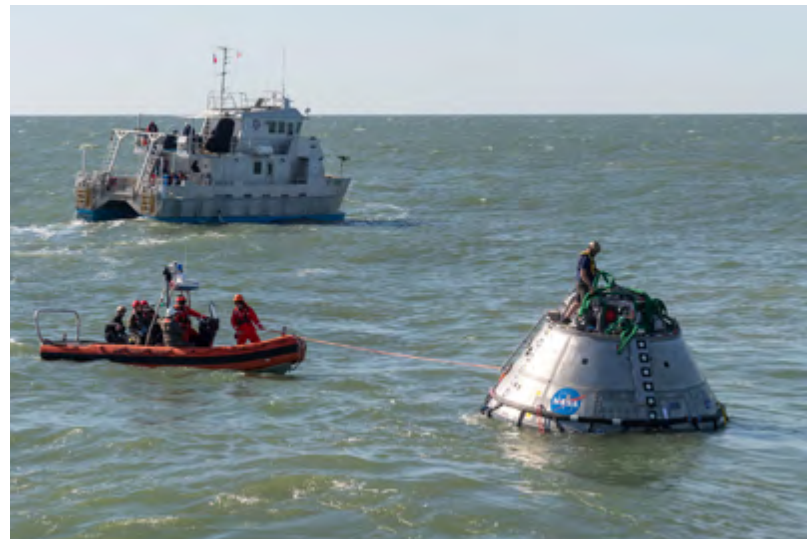
▲ The Orion Crew Module Uprighting System (CMUS) and Neutral Buoyancy Laboratory team completed two successful sea tests off the coast of Galveston, Texas. CMUS is designed to inflate five bags after the Orion spacecraft and its crew splash down after returning from deep space missions, enabling the capsule to right itself. Image credit: NASA
