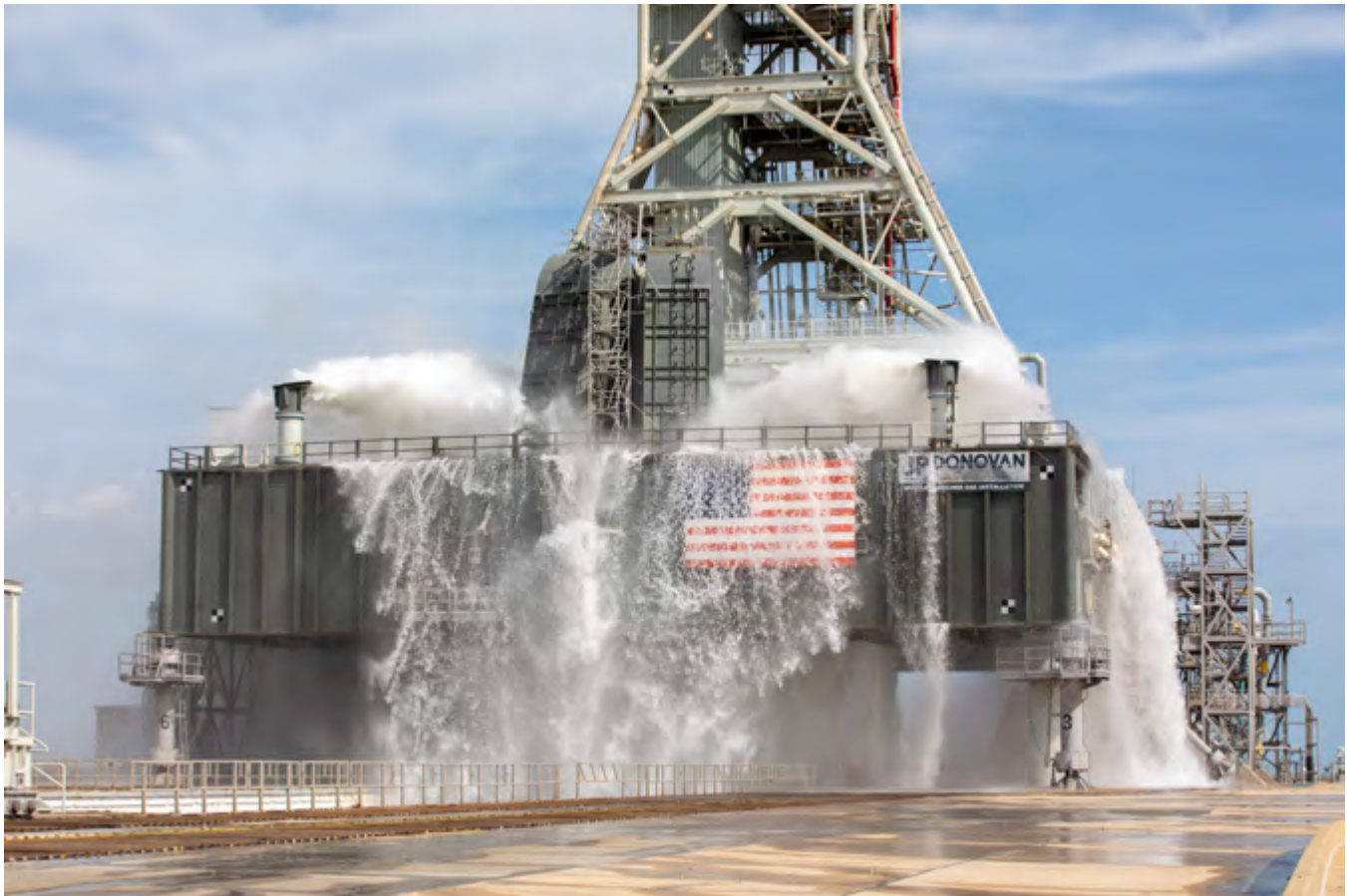
▲ A wet flow test at Launch Pad 39B on Sept. 13, 2019, tests the sound suppression system that will be used for the launch of NASA's Space Launch System for the Artemis I mission. During the test, about 450,000 gallons of water poured onto the Pad B flame deflector, the mobile launcher flame hole, and the launcher's blast deck. Image credit: NASA
