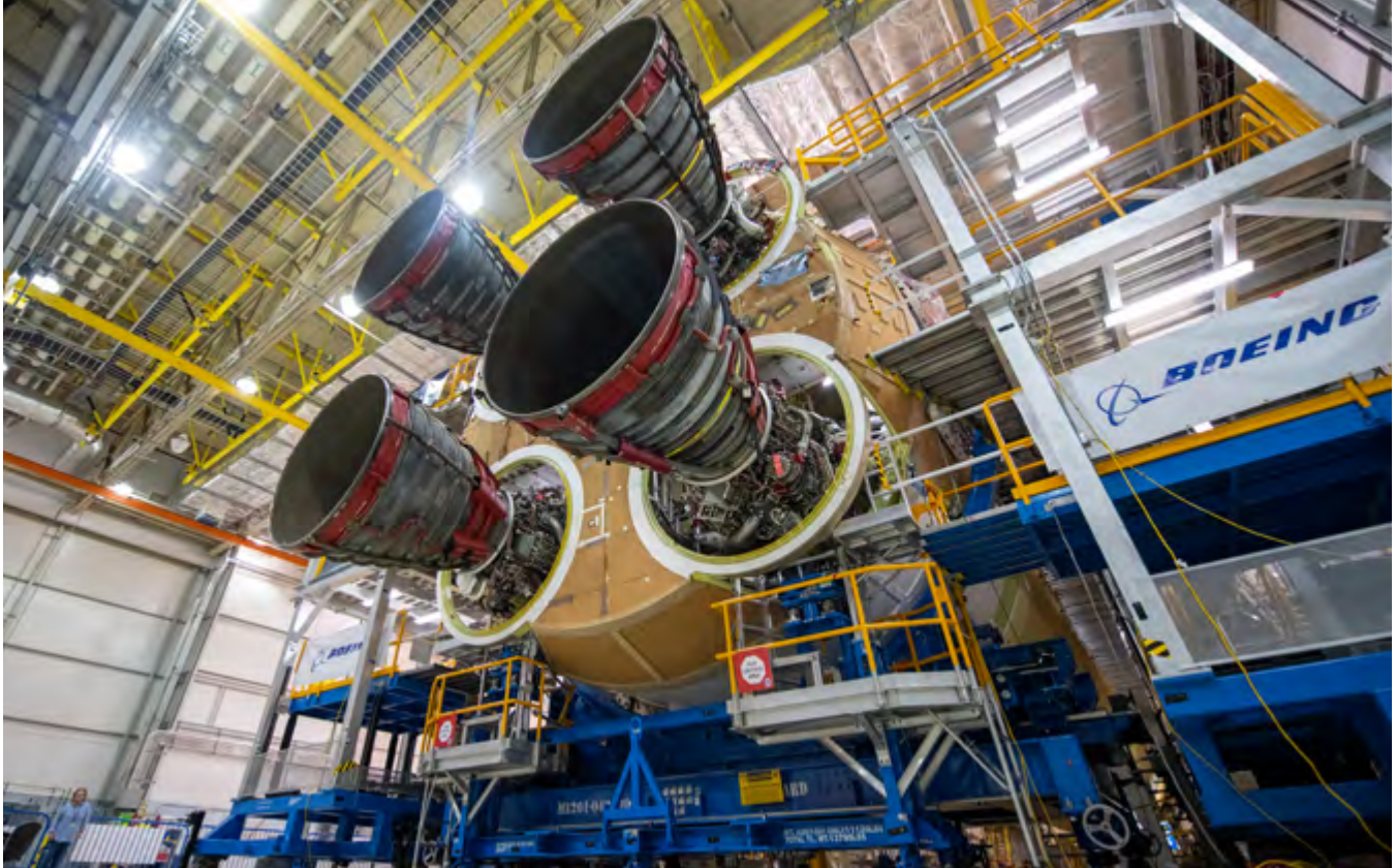
▲ All four RS-25 engines attached to the SLS core stage inside NASA's Michoud Assembly Facility in New Orleans. Image credit: NASA
