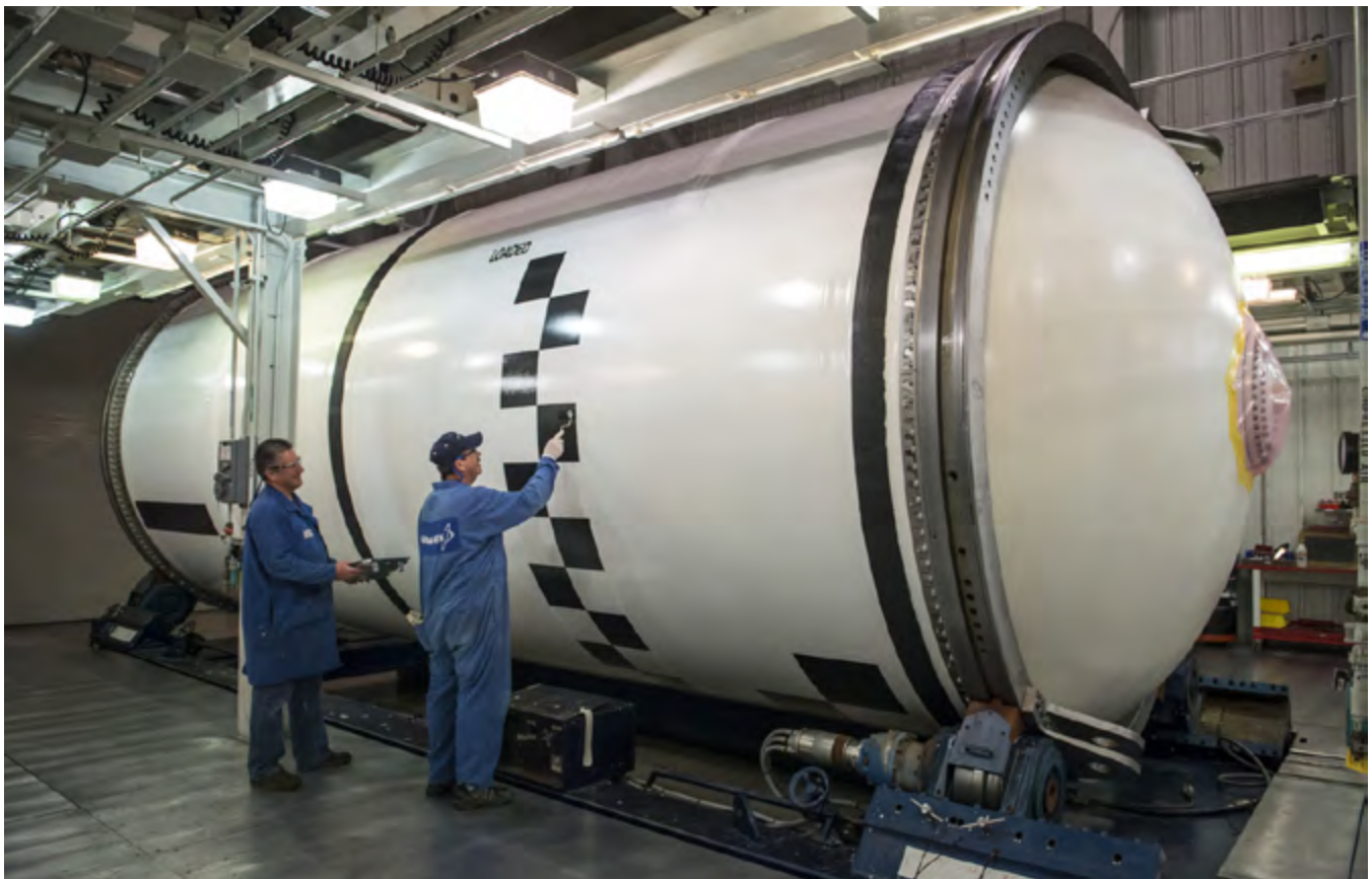
▼ Technicians with lead solid rocket boosters contractor Northrop Grumman paint photogrammetric markings on one segment of an SLS solid rocket motor.
