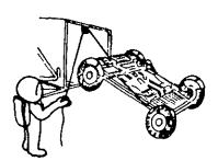
FORWARD CHASSIS LOCKS IN POSITION. ASTRONAUT LOWERS LRY TO SURFACE WITH SECOND REEL.
