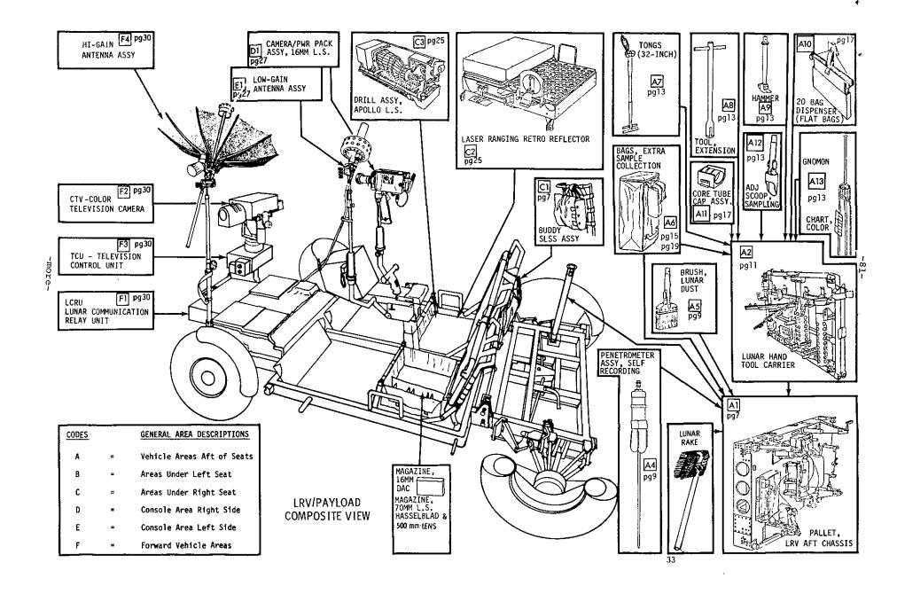
The LRV will travel to the Moon folded inside stowage Quadrant 1 of the lunar module's descent stage. During the first lunar surface EVA period the astronauts will manually deploy the vehicle and prepare it for cargo loading and operation.
