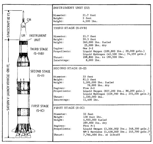
NOTE: Weights and measures given above are for the nominal vehicle configuration for Apollo. The figures may vary slightly due to changes before launch to meet changing conditions. Weights of dry stages and propellants do not equal total weight because frost and miscellaneous smaller items are not included in chart.
