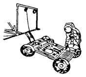
. ASTRONAUT UNFOLDS SEATS, FOOTRESTS, ETC. (FINAL STOP)
