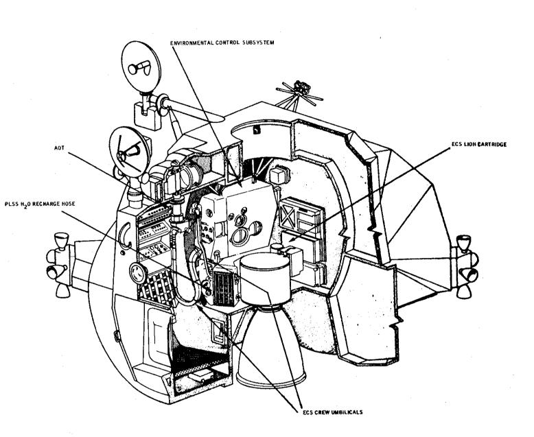
Cutaway of LM cabin interior, left half
