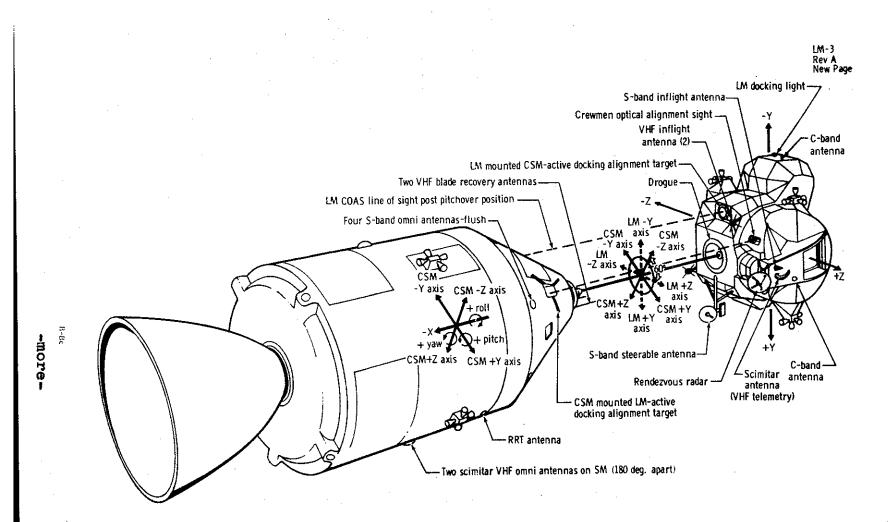
Figure 8-3.2. - LM-CSM antenna locations.
