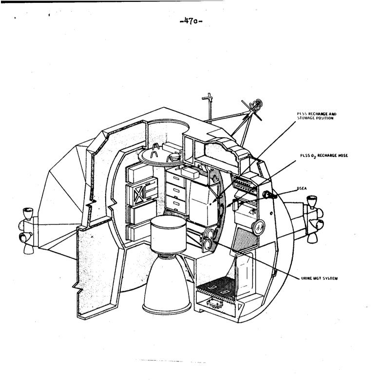
Cutaway of LM cabin interior, right half
