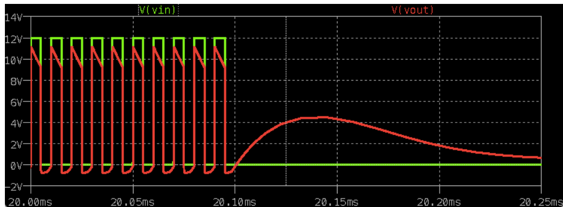
Figure 6. Gate Drive Circuit LTSpice Simulation During Abrupt Turn-Off (Green – Gate Drive Input from PWM Controller. Red – MOSFET Gate-Source Voltage)
