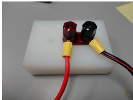
Figure 1: NBL Banana Plug Receptacle (electrical power)
