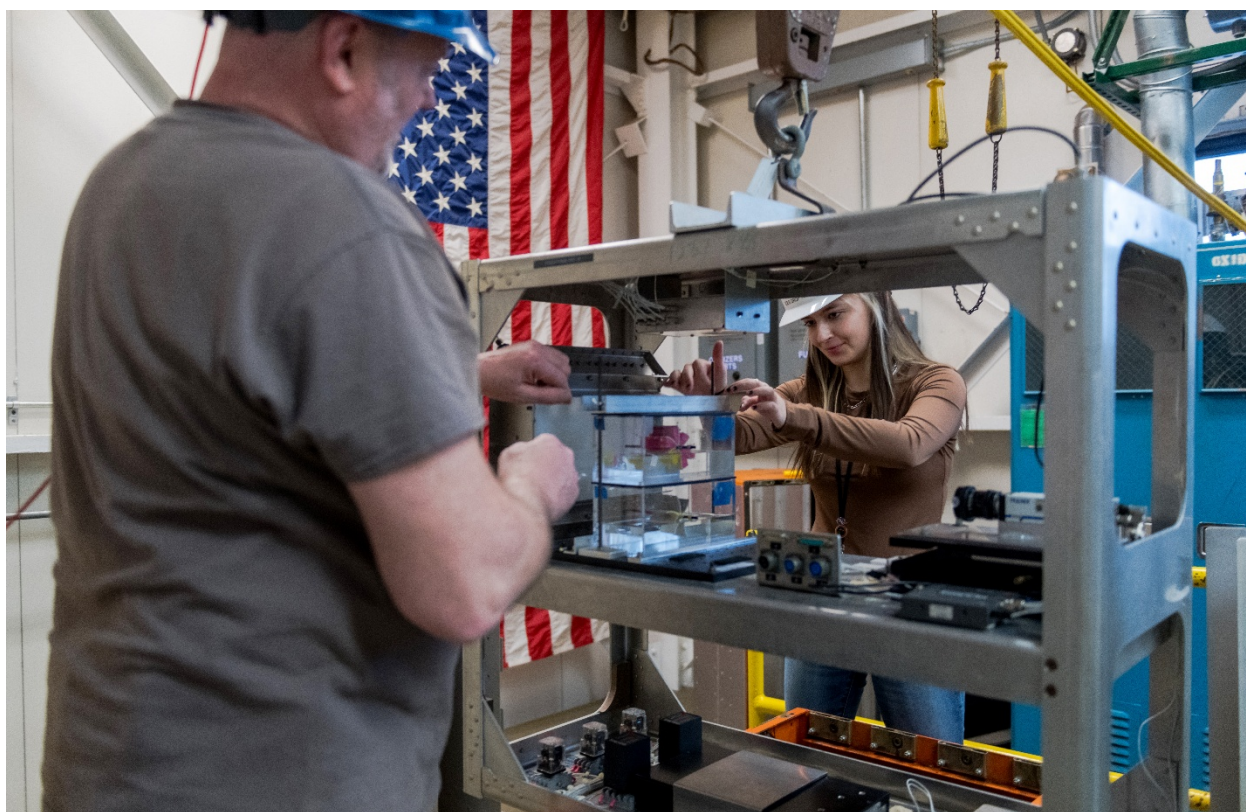
Figure 2 - Preparing for a drop on the fifth floor of the 2.2 Second Drop Tower.
