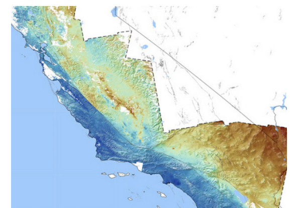
InSAR and GNSS-constrained displacement in California. Cornell University/Rowena Lohman
