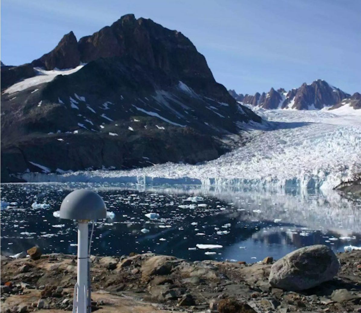
A GNET station weighs ice mass change in Greenland. Cornell University/Mike Willis
