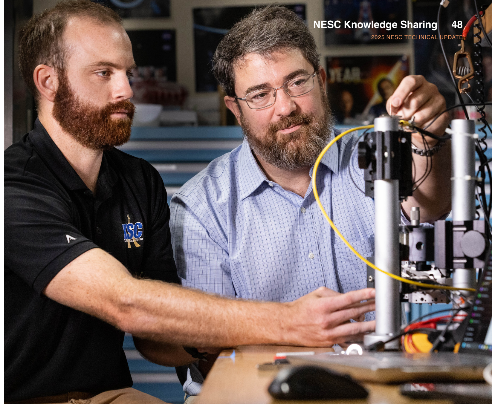
Left to right, Stefan Tomović and Dr. Christopher Biagi evaluate pressure transducers for the NESC. The probe is designed to improve the detection of thruster pressure sensor anomalies for the agency's Commercial Crew Program.
