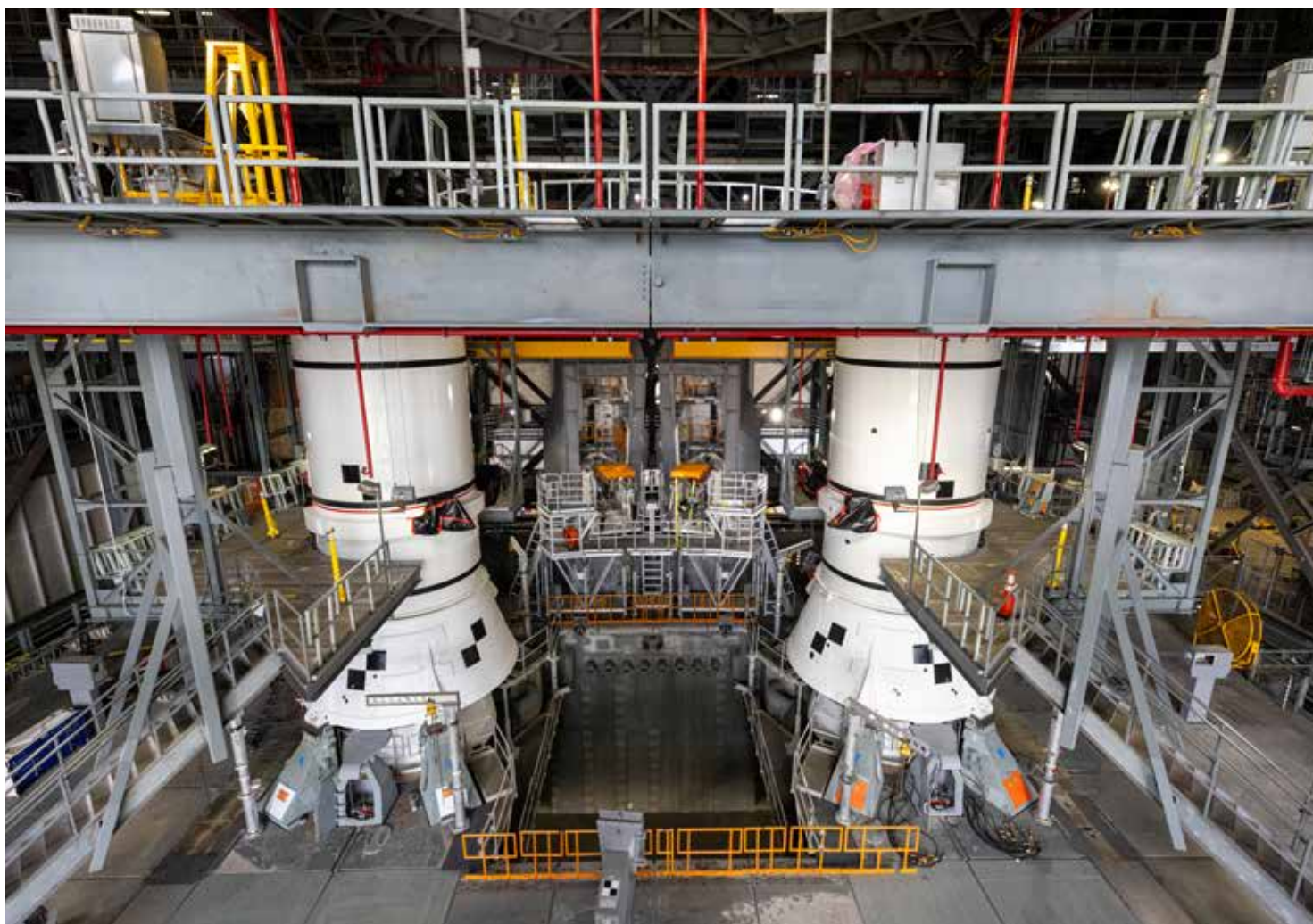
The left-hand and right-hand aft assembly solid rocket booster segments for NASA's Artemis III SLS rocket are secured to the mobile launcher at the agency's Vehicle Assembly Building at NASA's Kennedy Space Center in Florida on Saturday, July 11, 2026.
