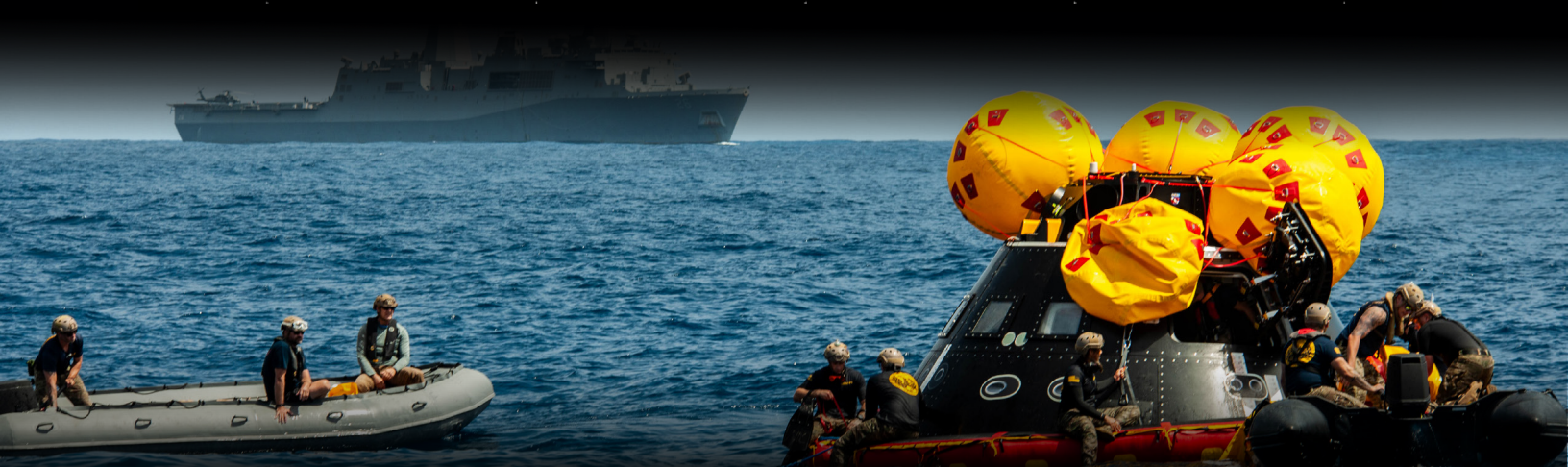
Image Caption: A NASA recovery team works near a floating Artemis II crew module test article during an underway recovery exercise at sea. The suited personnel and support vessels surround the capsule as part of training operations to practice safe astronaut retrieval after splashdown. Credits: NASA/Kenny Allen
