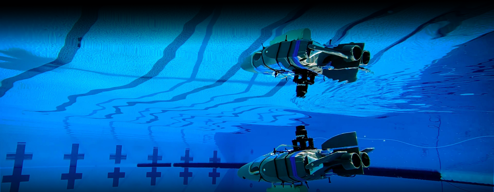
Image Caption: A prototype of a robot designed to explore the subsurface oceans of icy moons glides through a pool at Caltech in September 2024, its reflection visible below the water’s surface. The prototype was built at NASA’s Jet Propulsion Laboratory in Southern California to demonstrate the feasibility of a mission concept called SWIM, short for Sensing With Independent Micro-swimmers. The SWIM concept involves dozens of self-propelled, cellphone-sized robots exploring the waters of icy moons, like Jupiter’s Europa and Saturn’s Enceladus. Delivered to the subsurface ocean by an ice-melting cryobot, the tiny robots would zoom away to look for chemical and temperature signals that could point to life. Credit: NASA/JPL-Caltech
