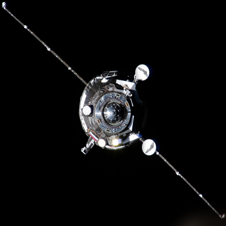
Image Caption: The uncrewed Progress 93 resupply ship from Roscosmos, carrying about three tons of food, fuel, and supplies for the Expedition 73 crew, is pictured automatically approaching the International Space Station before docking to the Zvezda service module's rear port for six months of cargo activities. Credits: NASA
