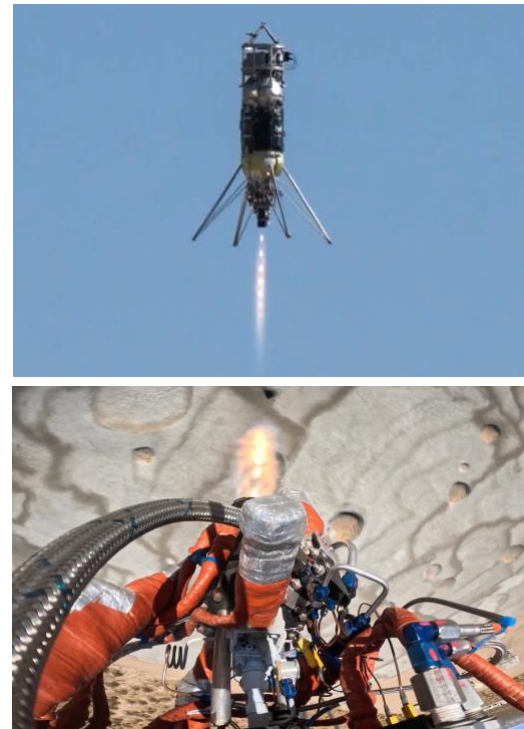
In November 2025, Astrobotic tested its hazard detection lidar sensor aboard its Xodiac lander (top) flying over its simulated lunar terrain (bottom) in preparation for its upcoming CLPS mission to the Moon. Credits: Astrobotic
