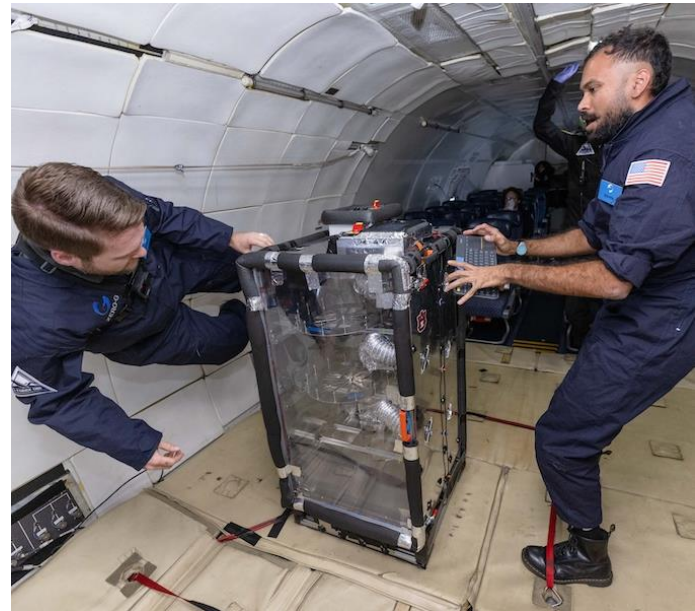
During two parabolic flight campaigns in FY 2025, Auburn University tested self-folding materials for use in lightweight, dust-resistant designs to deploy solar arrays and to open/close antennas. Credits: Zero Gravity Corp.
