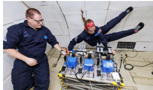
Testing three designs for a water separator during 2022 parabolic flights enabled Teledyne Energy Systems to down-select and integrate the best option into its commercial space fuel cell in 2025. Credits: Zero Gravity Corp.
