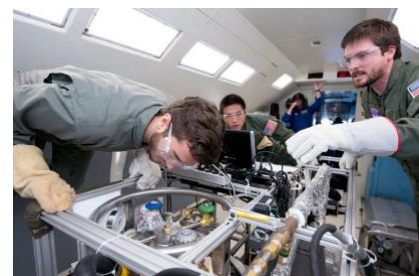
Parabolic flight test of cryogenic line chilldown in microgravity. Credits: NASA
