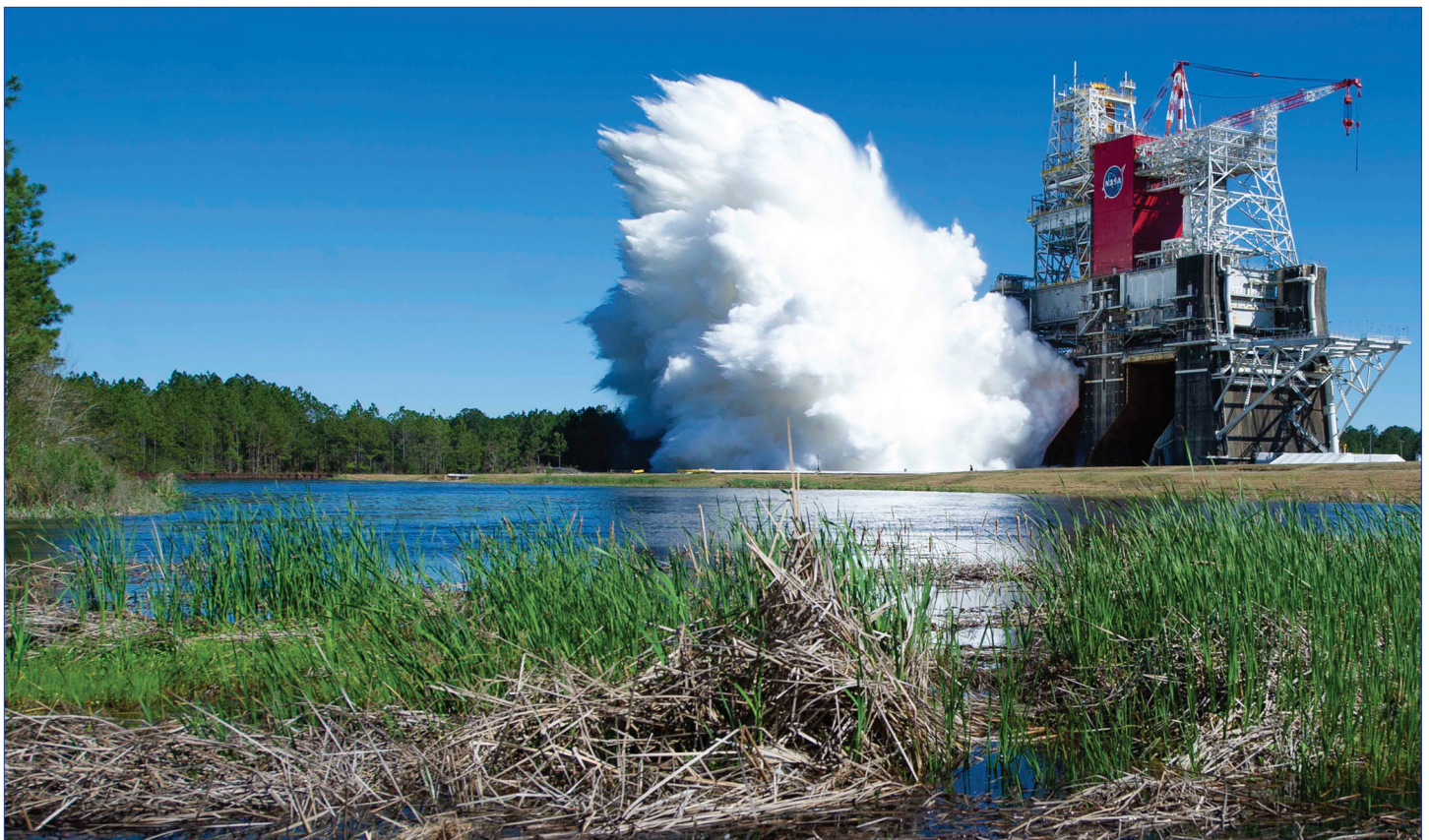
Stennis tests the first core stage of NASA's Space Launch System rocket, firing its four RS-25 engines simultaneously on the B-2 Test Stand (2021).
