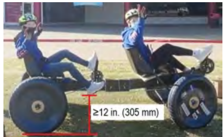
Figure 1: Vehicle Height Requirement.
