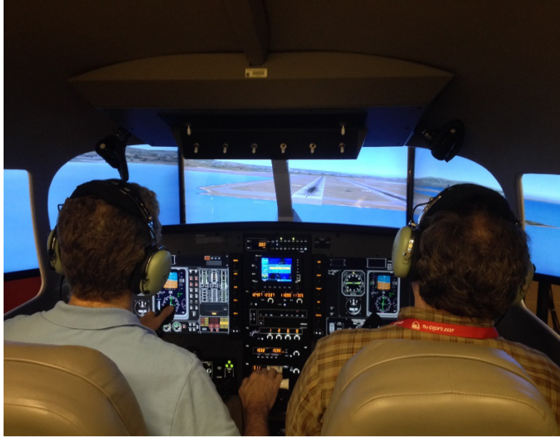
Figure 13. Interior view of flight simulation test bed for piloted evaluations.
