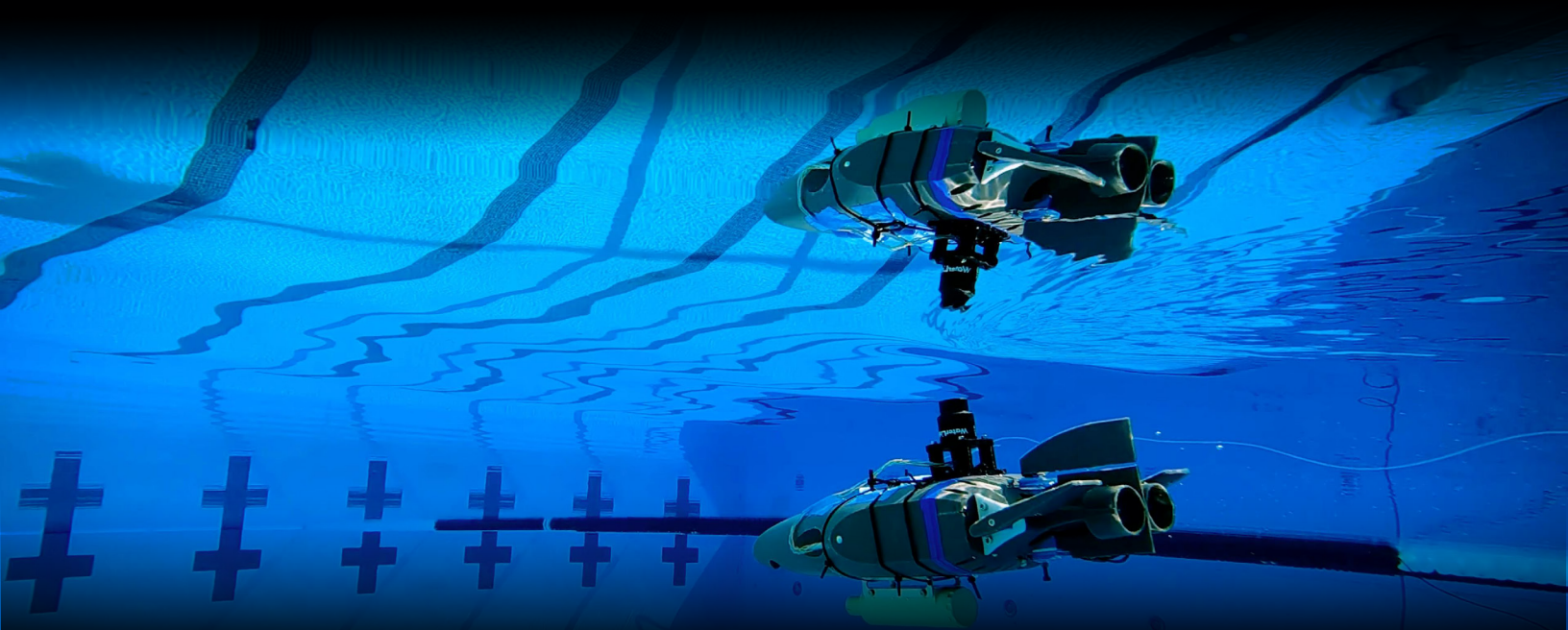
Image Caption: A prototype of a robot designed to explore the subsurface oceans of icy moons glides through a pool at Caltech in September 2024, its reflection visible below the water’s surface. The prototype was built at NASA’s Jet Propulsion Laboratory in Southern California to demonstrate the feasibility of a mission concept called SWIM, short for Sensing With Independent Micro-swimmers. The SWIM concept involves dozens of self-propelled, cellphone-sized robots exploring the waters of icy moons, like Jupiter’s Europa and Saturn’s Enceladus. Delivered to the subsurface ocean by an ice-melting cryobot, the tiny robots would zoom away to look for chemical and temperature signals that could point to life. Credit: NASA/JPL-Caltech
