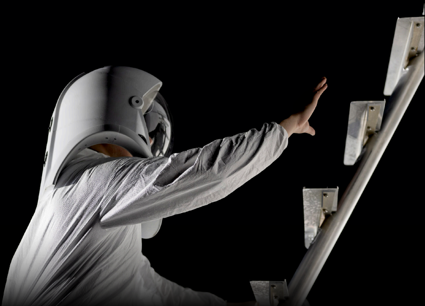
Image Caption: Wearing a low-fidelity spacesuit, a test engineer studies how the extreme lighting of the Moon’s South Pole could affect surface operations during Artemis III. Teams at NASA’s Marshall Space Flight Center’s Flat Floor Facility used high-intensity lights positioned at a low angle to replicate the strong shadows that are cast across the lunar South Pole by the Sun. Credit: NASA/C. Beason
