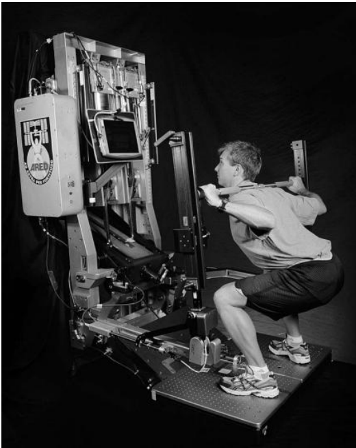
Demonstration of the Advanced Resistive Exercise Device (ARED) Source: NASA
