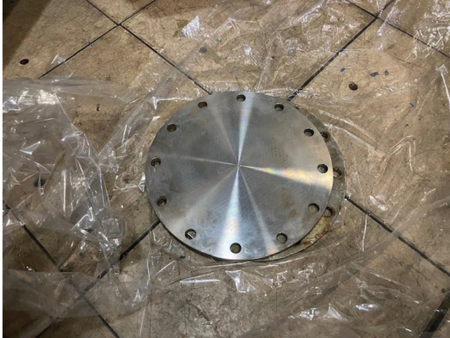
Figure 27. Example of metal cover to be installed over existing penetrations after solar simulator removal, allowing for future equipment to be added without modifications to the pressure vessel.
