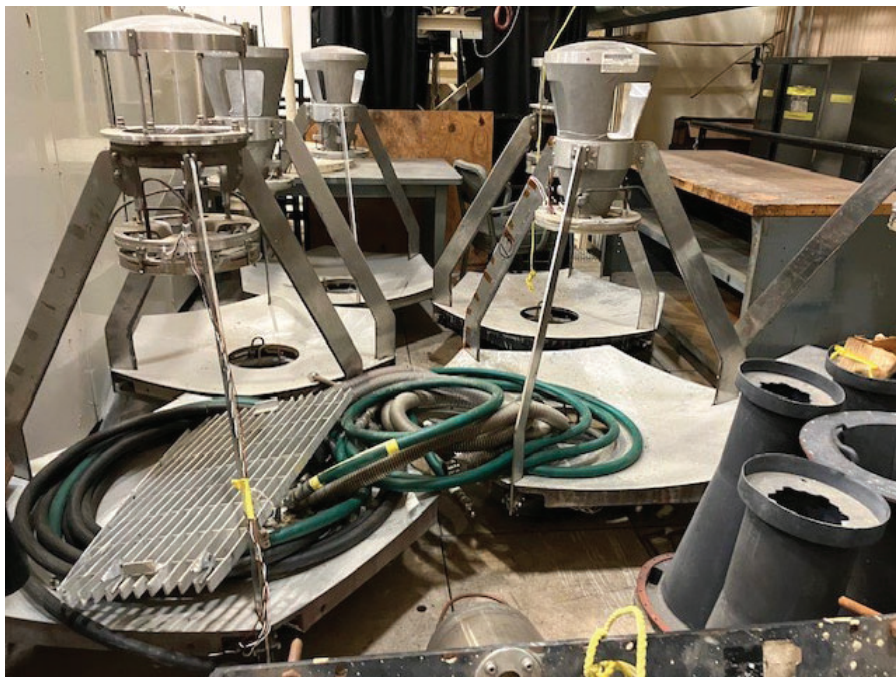
Figure 26. Mirrors for solar simulators on Chamber B, removed over 15 years ago, to be excessed.
