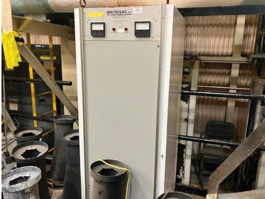
Figure 15. Example of peripheral remote control unit for solar simulators on Chamber B to be removed and excessed.
