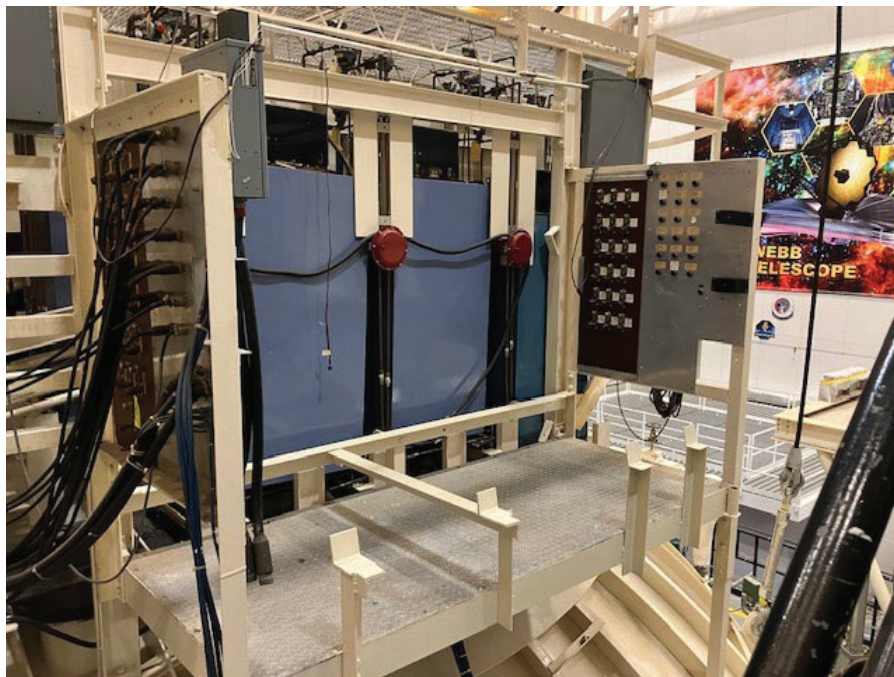
Figure 8. Solar simulators located on the top of Chamber B.
