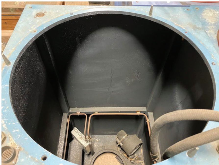
Figure 32. Solar simulator module source and collection optics housing internal components, showing frame for xenon lamp source and collection optics.
