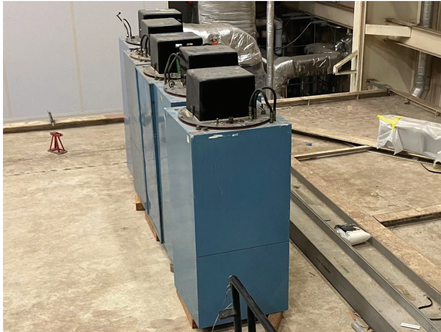
Figure 29. Solar simulator module xenon lamp source and collection optics housing showing removable panel on one side.
