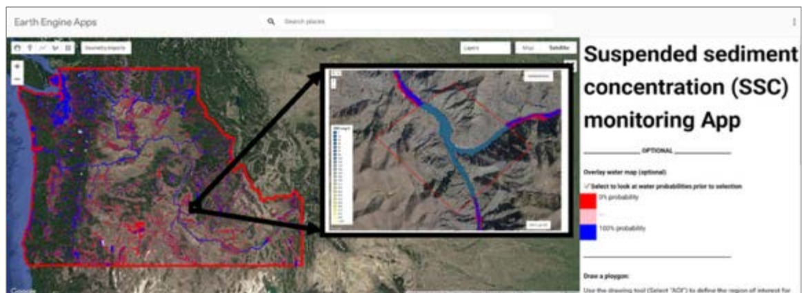
Screenshot of the suspended sediment concentration Google Earth Engine monitoring app using Landsat and Sentinel-2 imagery. Credit: U.S. Department of the Interior.
