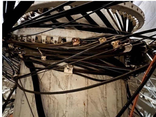
Figure 5: Cable Wrap Damage
