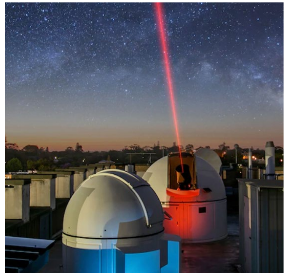
Figure 11.41 The 70 cm Western Australian Optical Ground Station (WAOGS) is installed on a rooftop at the University of Western Australia. Credit: The International Centre for Radio Astronomy Research.
