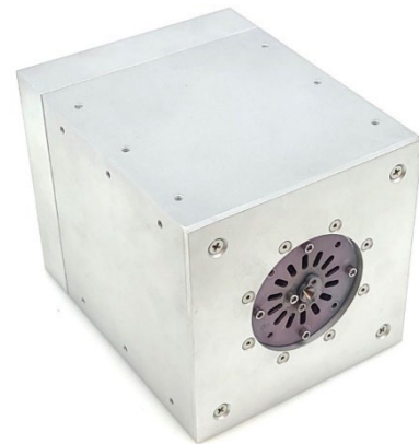
Figure 4.19: Aurora Resistojet Module for Attitude Control. Credit: Aurora Propulsion Technologies.
