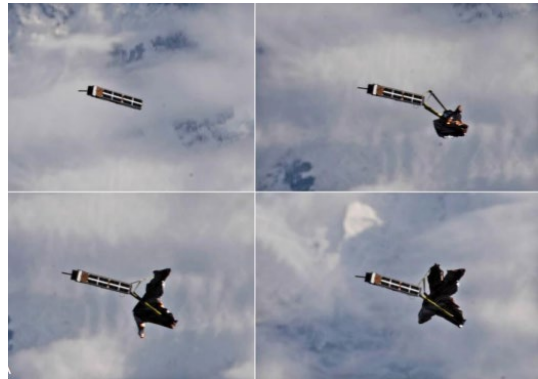
Figure 13.9: TechEdSat-10 aft-imaging captures Exo-Brake deployment July 2020 (29). Credit: NASA.
