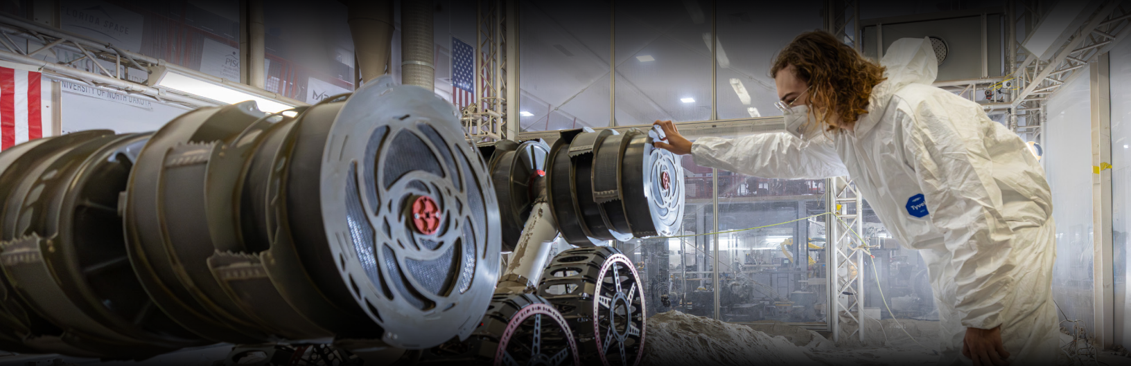
Image Caption: Ben Burdess, mechanical engineer, observes NASA’s Regolith Advanced Surface Systems Operations Robot (RASSOR) excavating simulated regolith, or lunar dust, during a test inside the Granular Mechanics and Regolith Operations Lab at NASA’s Kennedy Space Center in Florida on May 27, 2025. RASSOR is designed to work in low-gravity situations, using counter rotating bucket drums on each arm to collect and dump regolith for the extraction of hydrogen, oxygen, or water, resources critical for sustaining a habitable presence. Credit: NASA/F. Michaux
